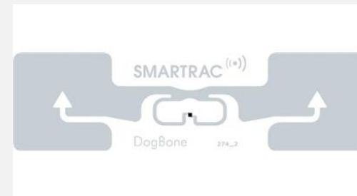
SMARTRAC DogBone RFID Wet Inlay (Monza 4D)
