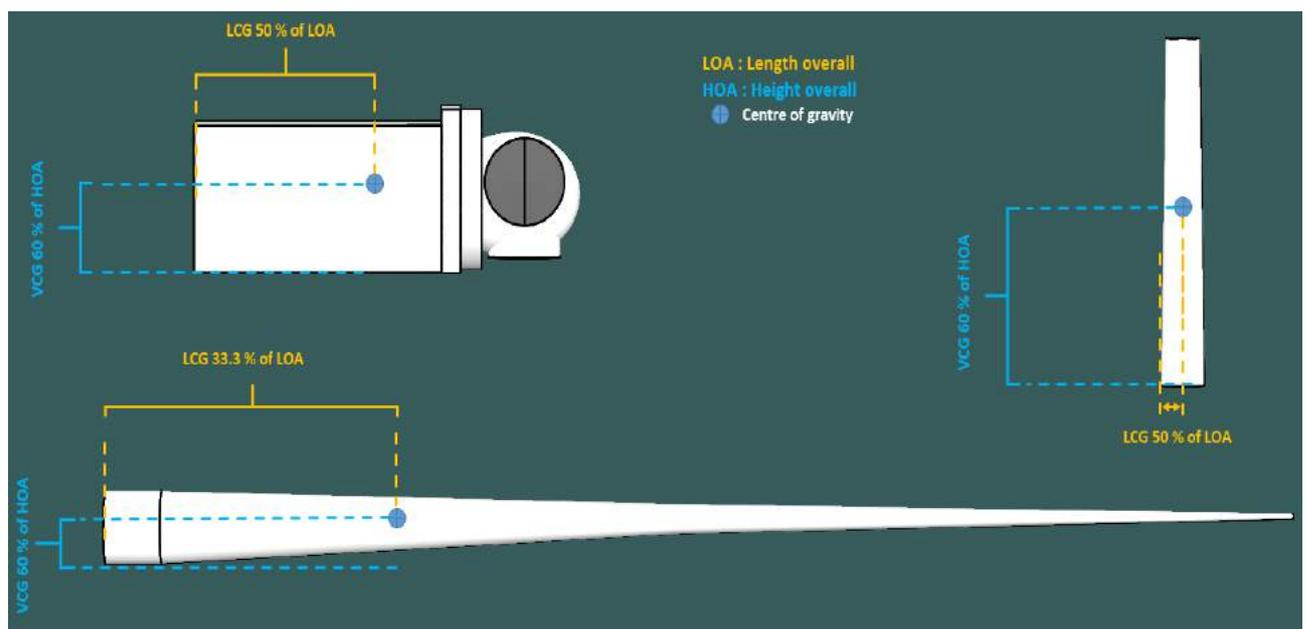
Figure 7-20 VCG, TCG & LCG of 12MW Wind Turbine
