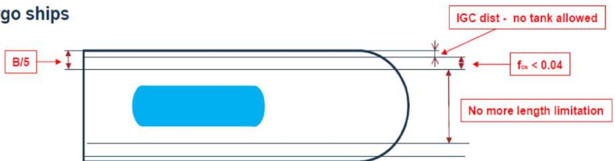
Figure 5-30 Location of LNG tank based on IGF code (Kokarakis 2015)
