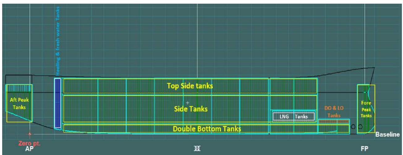
Figure 5-21 Side View of Decom Tools Vessel's Tanks
