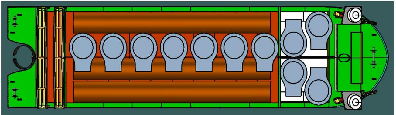
Figure 6-30 Top view of Load out of 12MW TP & Monopile (First Arrangement)
