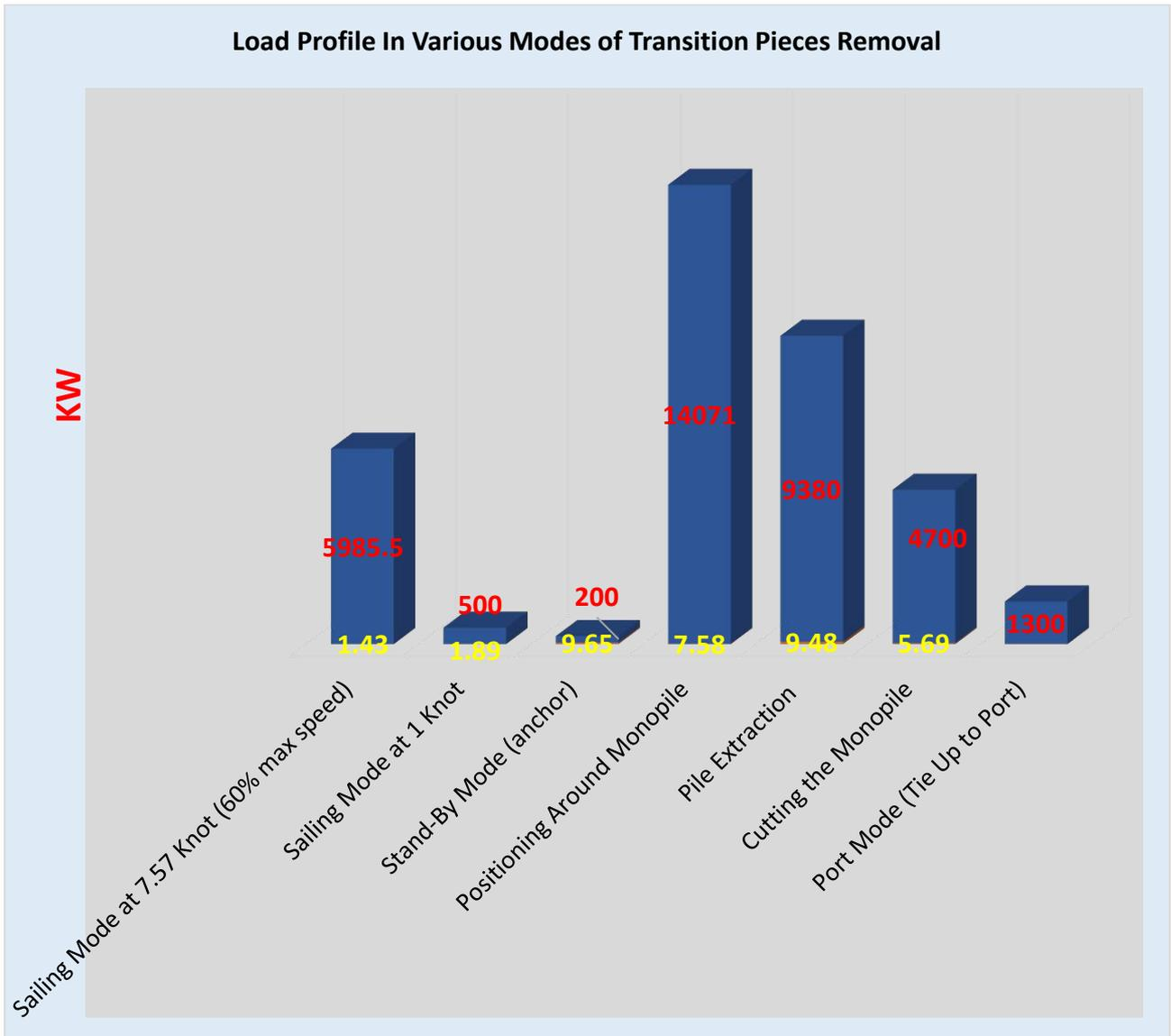
Figure 5-77 Load Profiles During Transition Piece Removal
