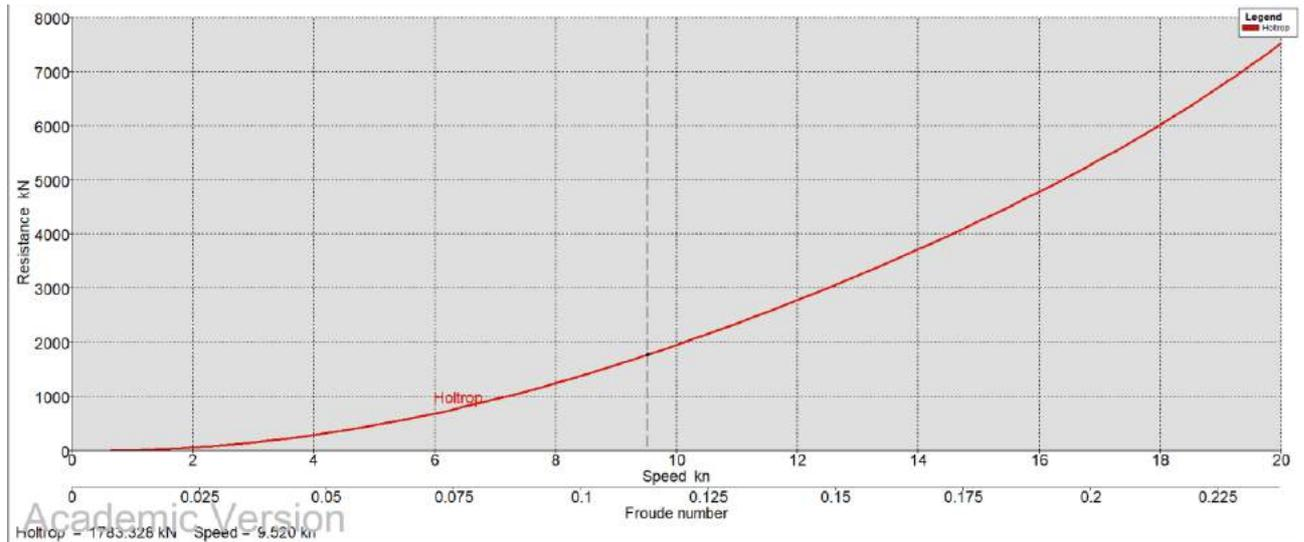
Figure 5-64 Correlation Between Speed and Resistance at Draft of 19.79 meters
