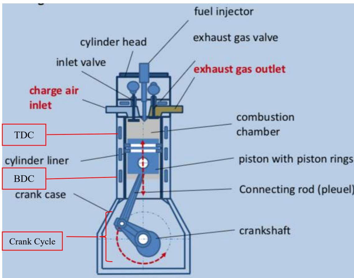
Figure 4-2 Cross Section of 4 Stroke Diesel Engine
