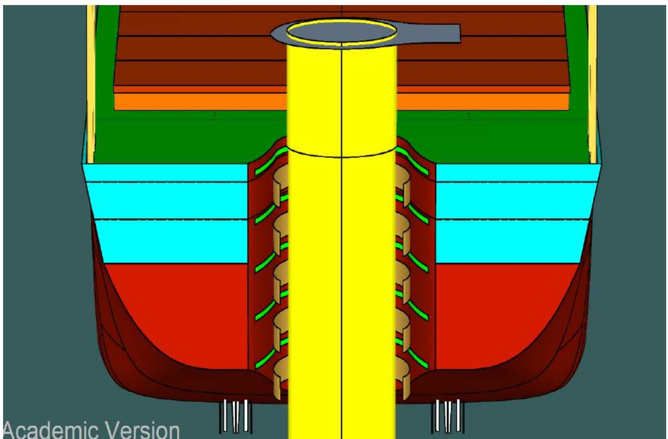
*Figure 6-93 Grippers are Open to hold the TP*
