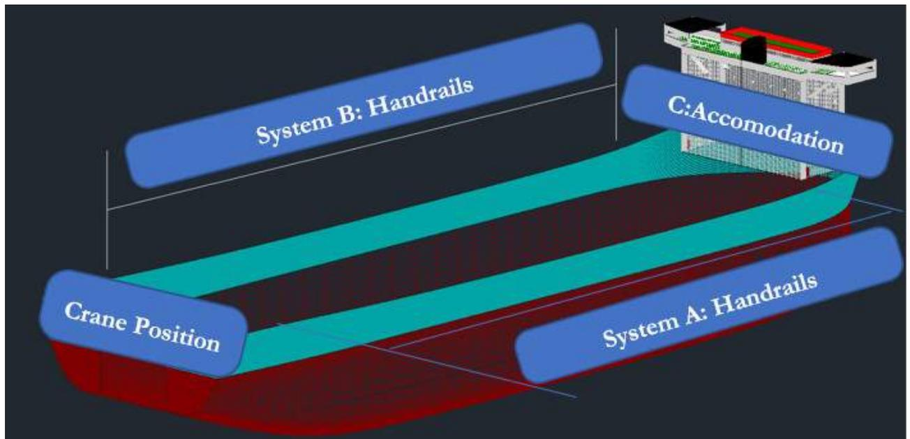
Figure 5-54 Location of Solar Panel on Decom Tools Vessel (System A, B & C)
