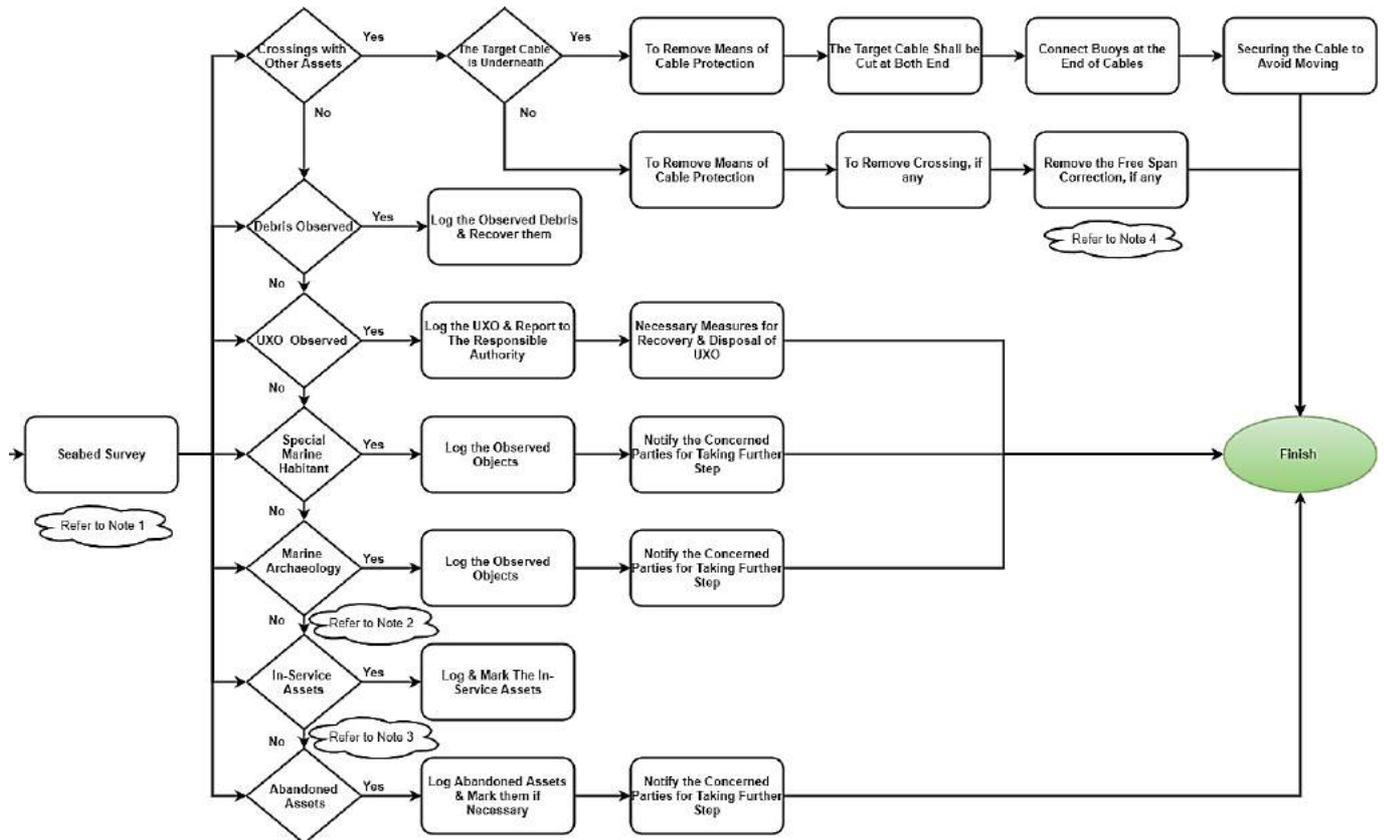
Figure 6-180 Pre-decommissioning Operation for Cable Extraction
