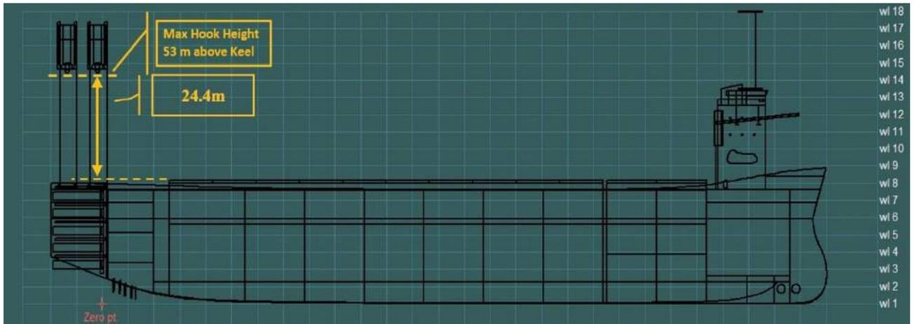
Figure 5-42 Height of Gantry Crane
