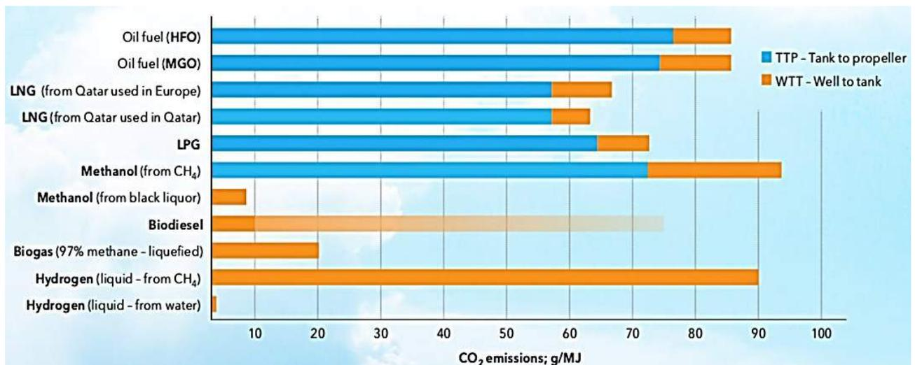
Figure 4-25 CO<sub>2</sub> Emission of Various Fuel Types
