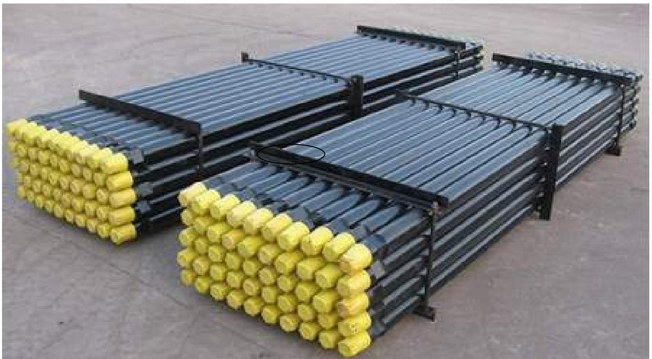
*Figure 6-236 Marshaling the Drill Pipes*
