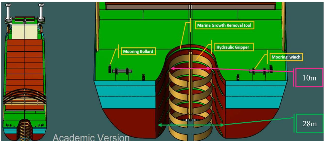
Figure 5-87 Details of Stern of the Decom Tools Vessel (Pile Gripper and MGR System)
