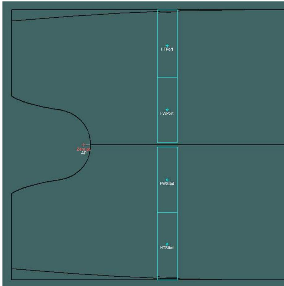
Figure 5-36 Plan of Fresh Water and Heeling Tanks
