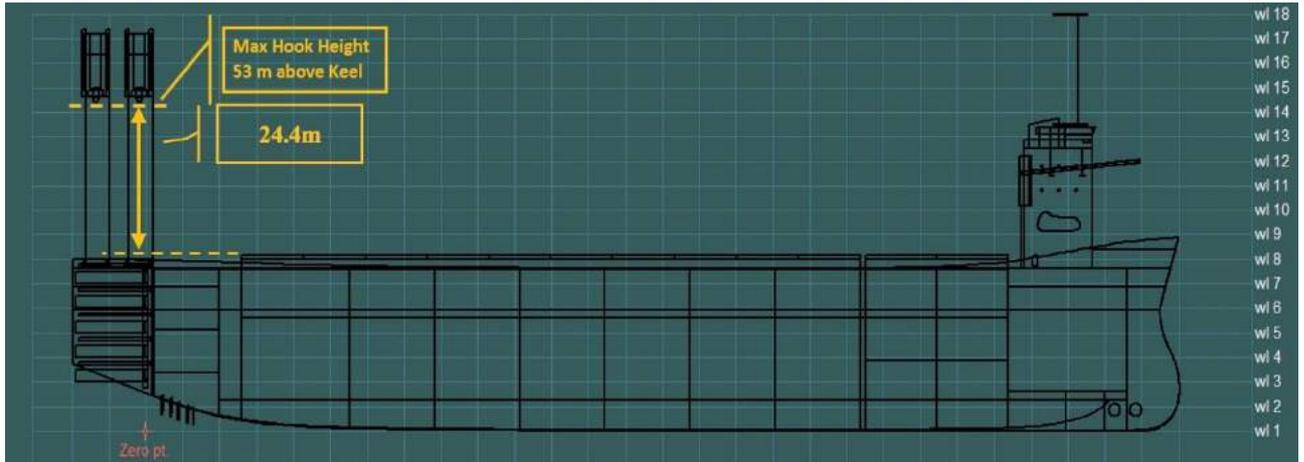
Figure 5-42 Height of Gantry Crane
