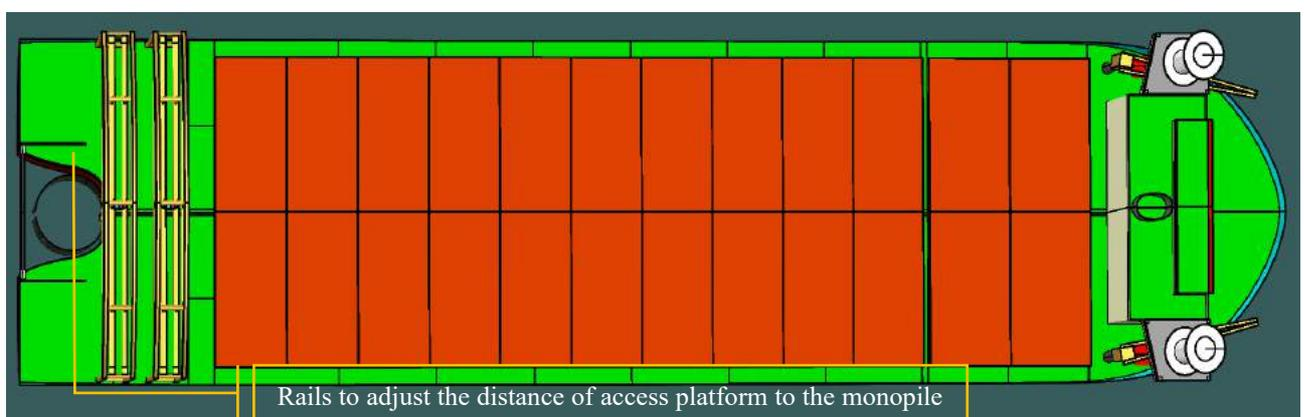
*Figure 6-145 Plan View of Access Platform*
