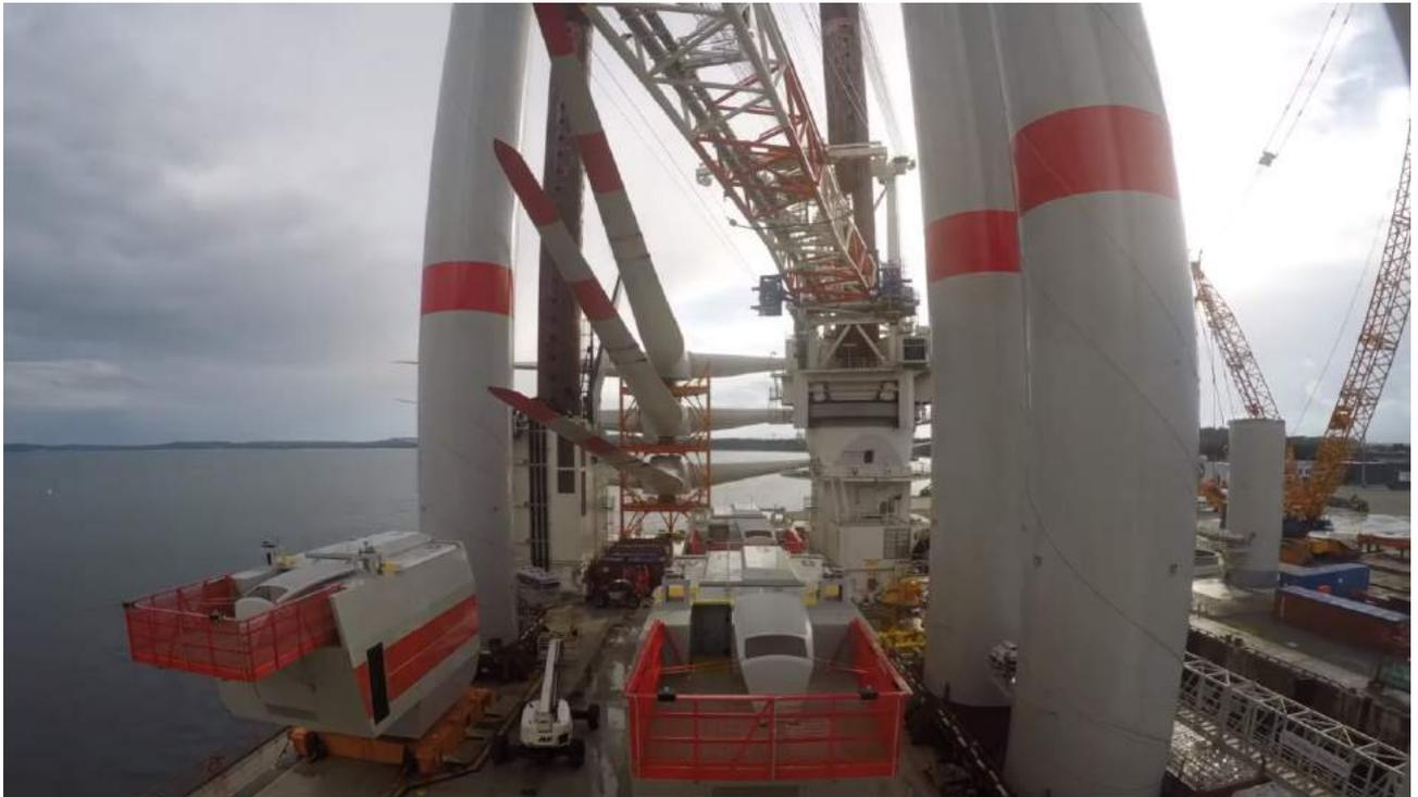
Figure 6-36 Transportation of 5MW Wind Turbine to Wikinger OWP (Fred Olsen Windcarrier 2017)
