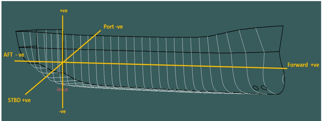
Figure 7-2 Direction and Coordinate of the Vessel
