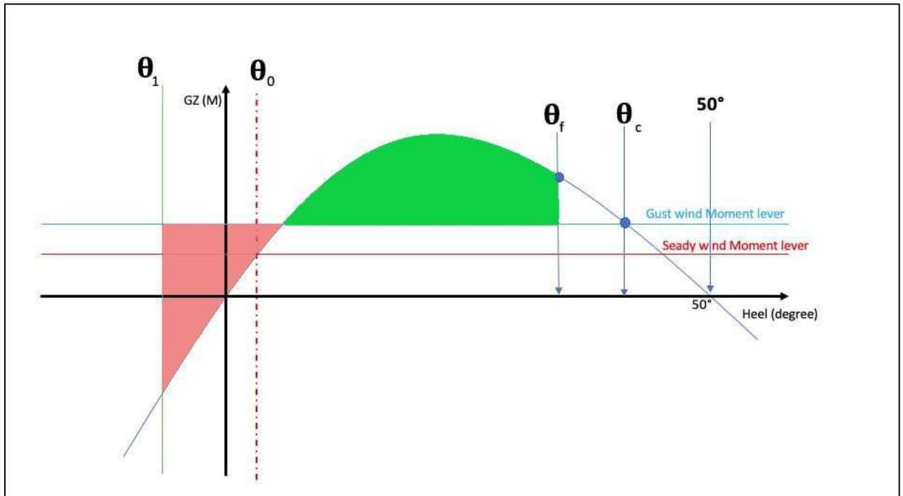
Figure 7-25 Sever Wind and Rolling GZ Curve
