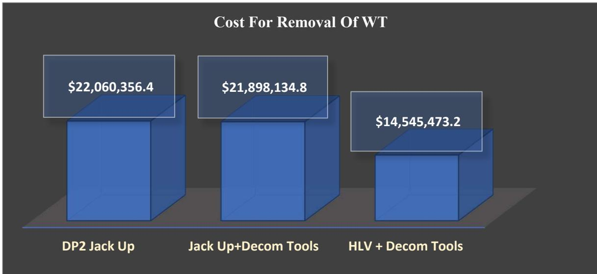
Figure 3-37 Cost of Various Logistic Configuration in Decommissioning of Noblewind OWP
