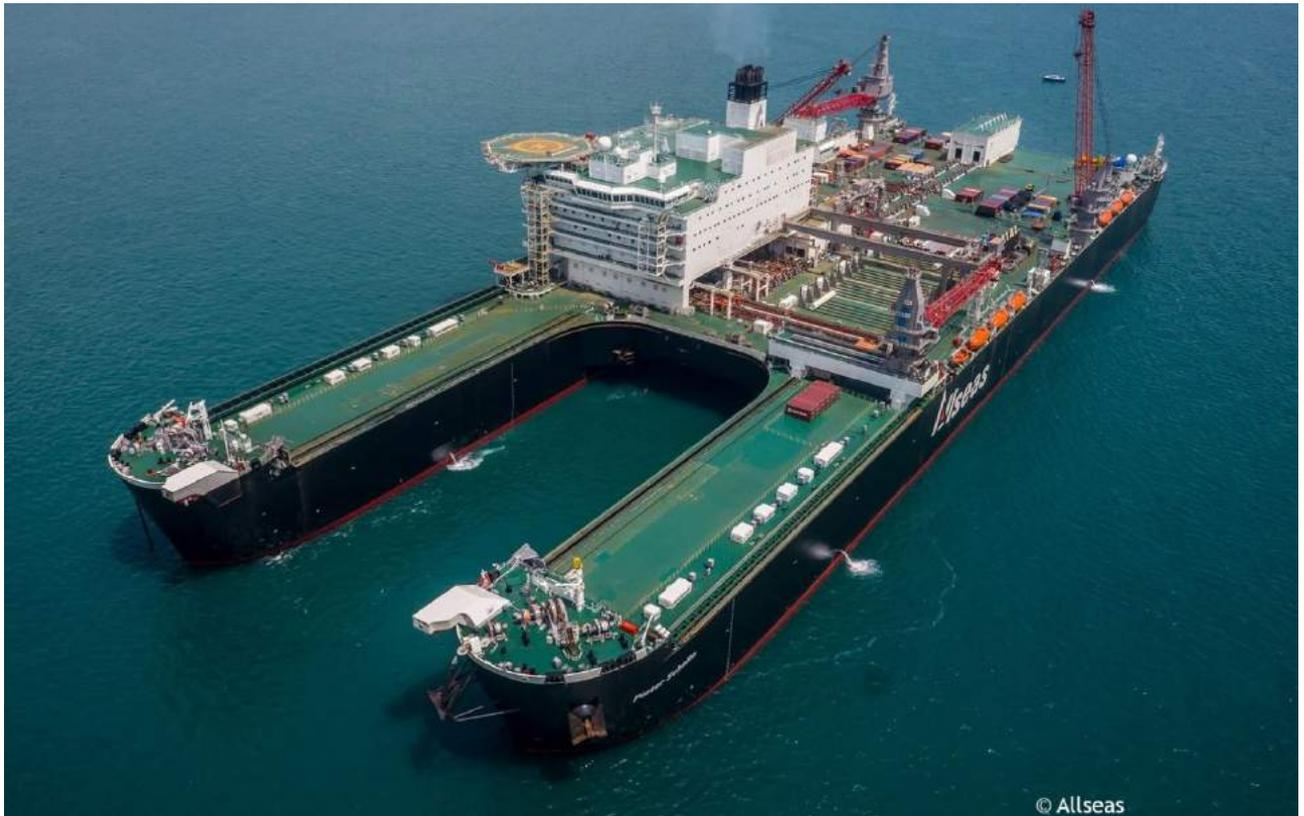
Figure 6-125 Pioneer Spirit without lifting Yokes
