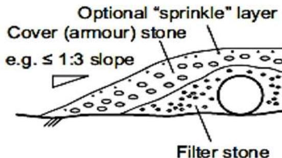
Figure 6-181 Rock Dumped on the cable as means of protection
