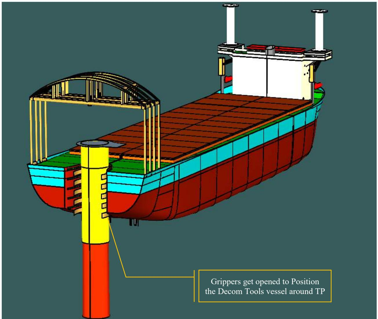
*Figure 6-94 Positioning the TP Inside the Grippers*
