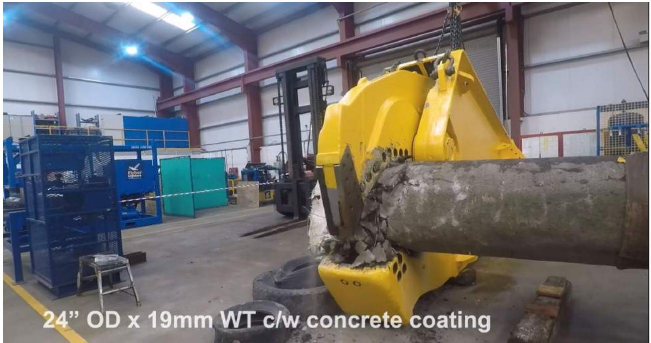
*Figure 6-4 Shear Cutting Tool*
