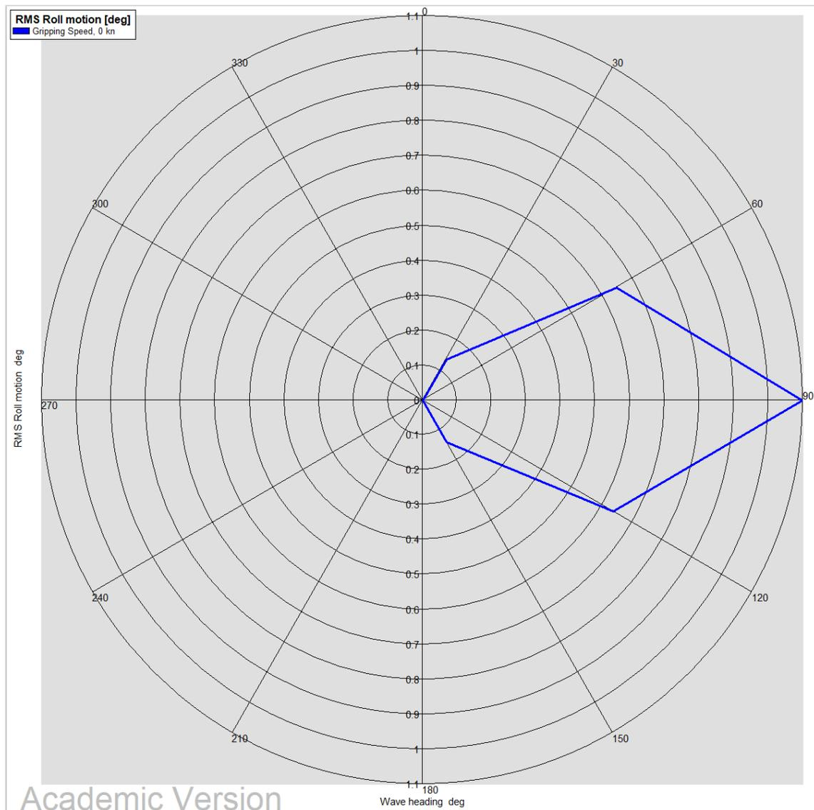
Figure 8-9 Roll Motion at COG – Slight Sea state
