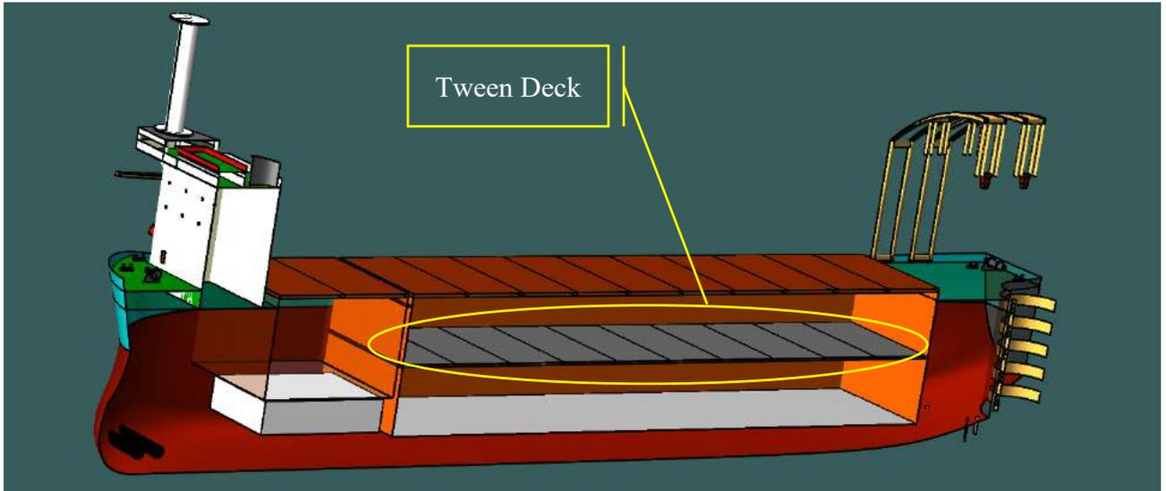
Figure 5-14 Cross Section of Decom Tools Vessel to show the Tween Deck
