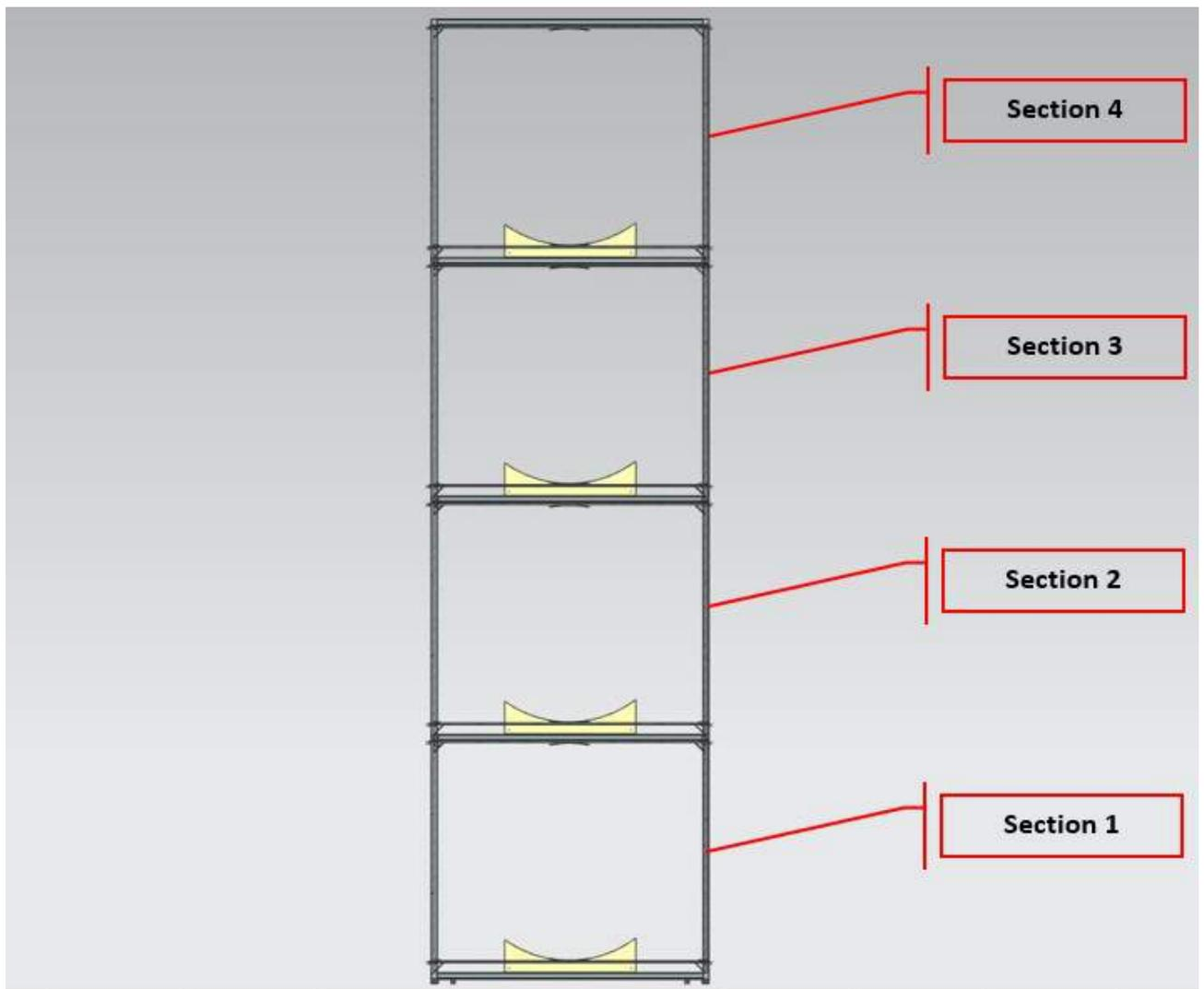
Figure 6-62 One rack for the Seafastening 4 blades (12 MW)
