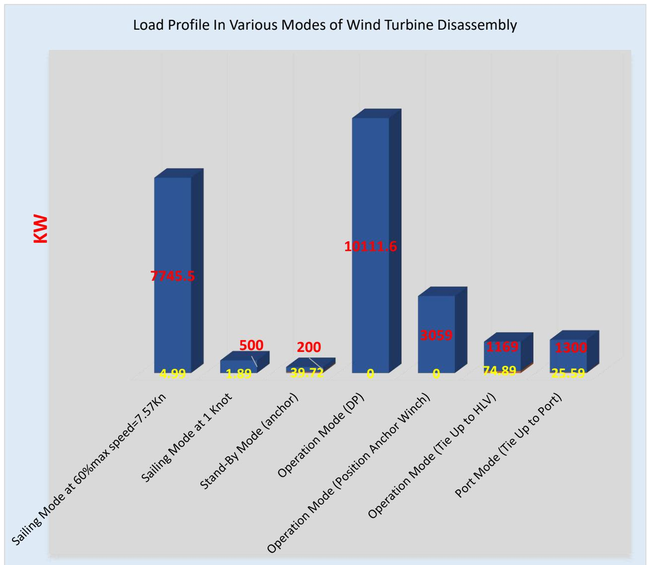
Figure 5-75 Load Profiles During Disassembly of Wind Turbines
