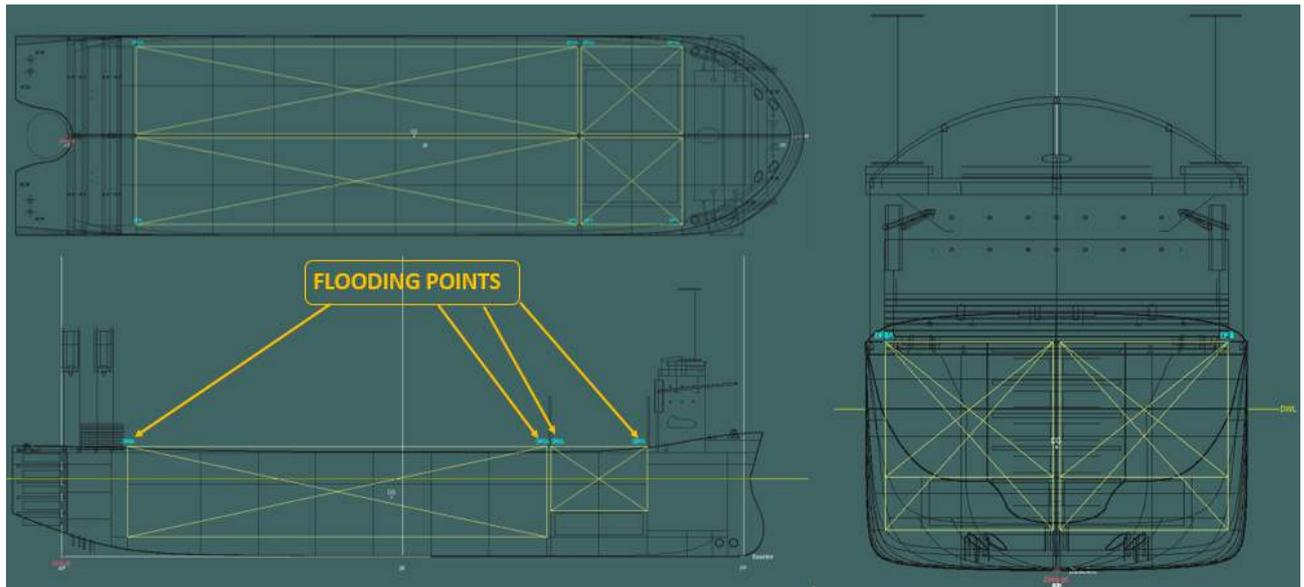
Figure 7-19 Flooding Point of the Decom Tools Vessel
