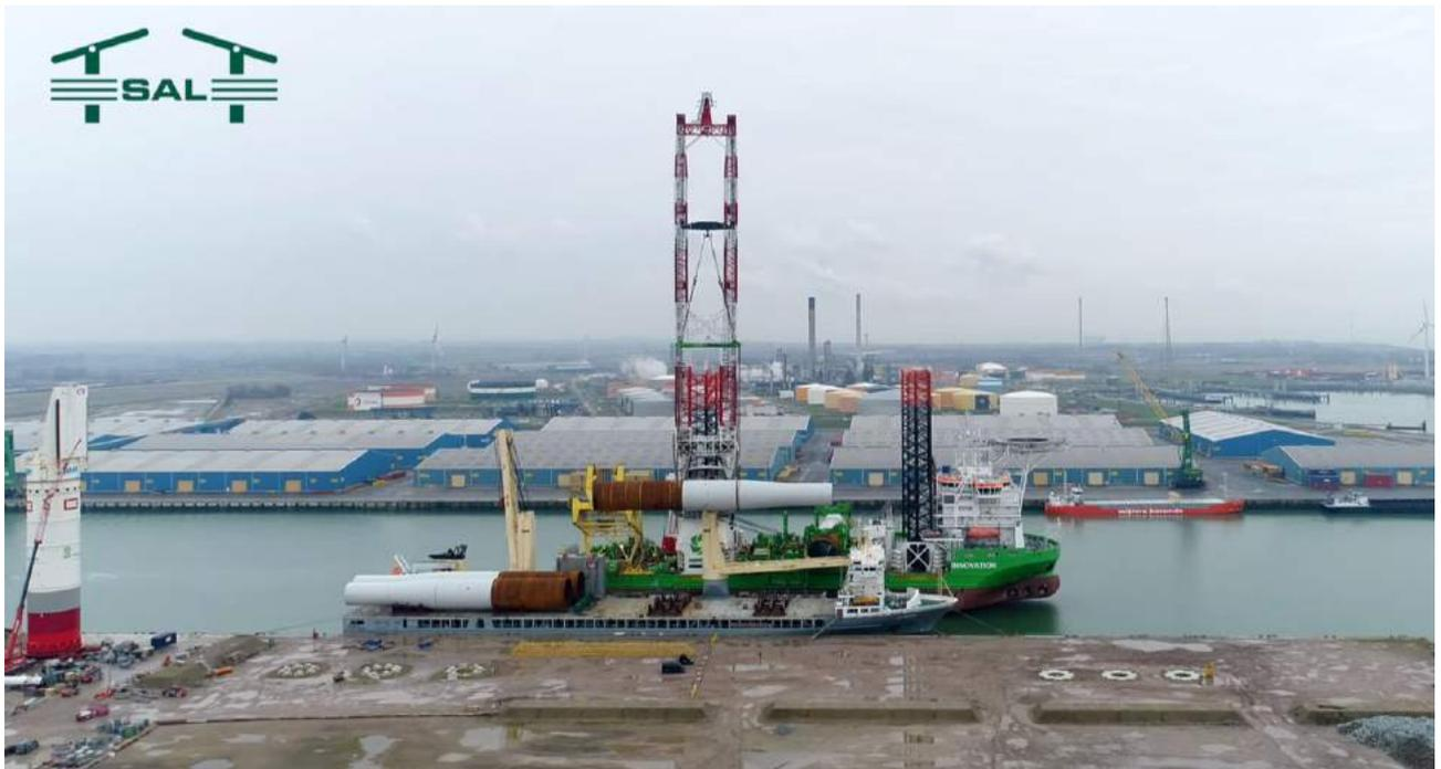
*Figure 3-17 Loading the Cargos from Cargo Vessel to The Installation Vessel*
