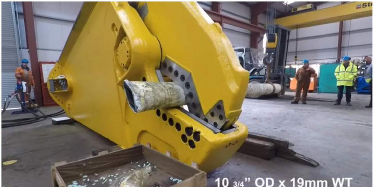
Figure 6-219 Shear Cutting Tool (James Fisher Offshore 2019)
