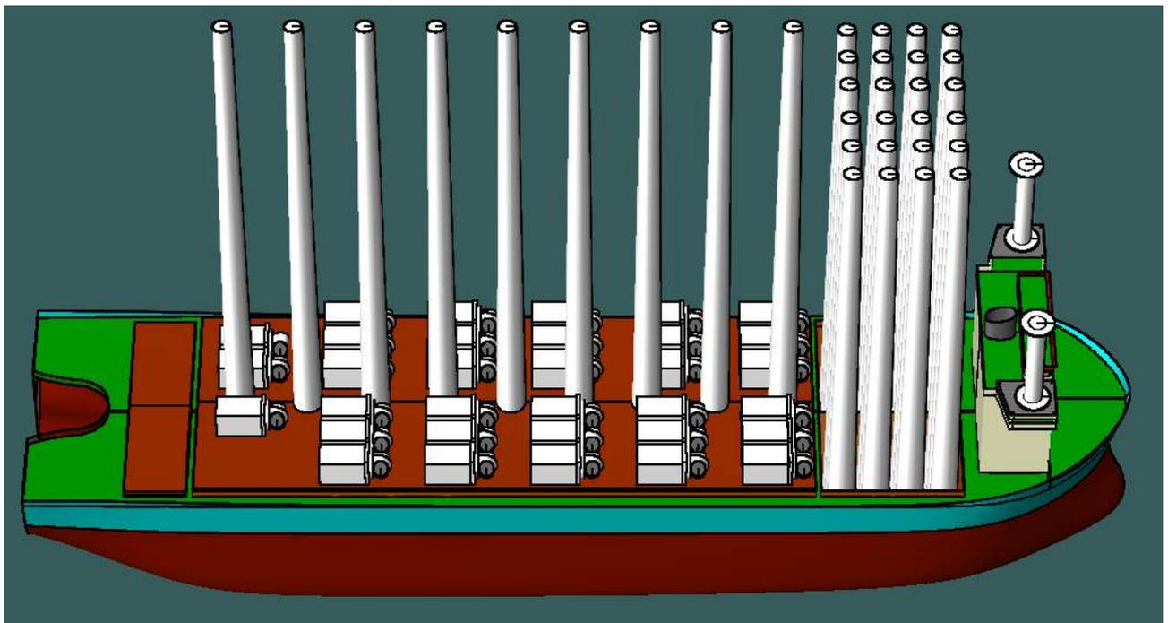
Figure 7-37 33 Sets of 3.6 MW WT Loaded on the Decom Tools Vessel
