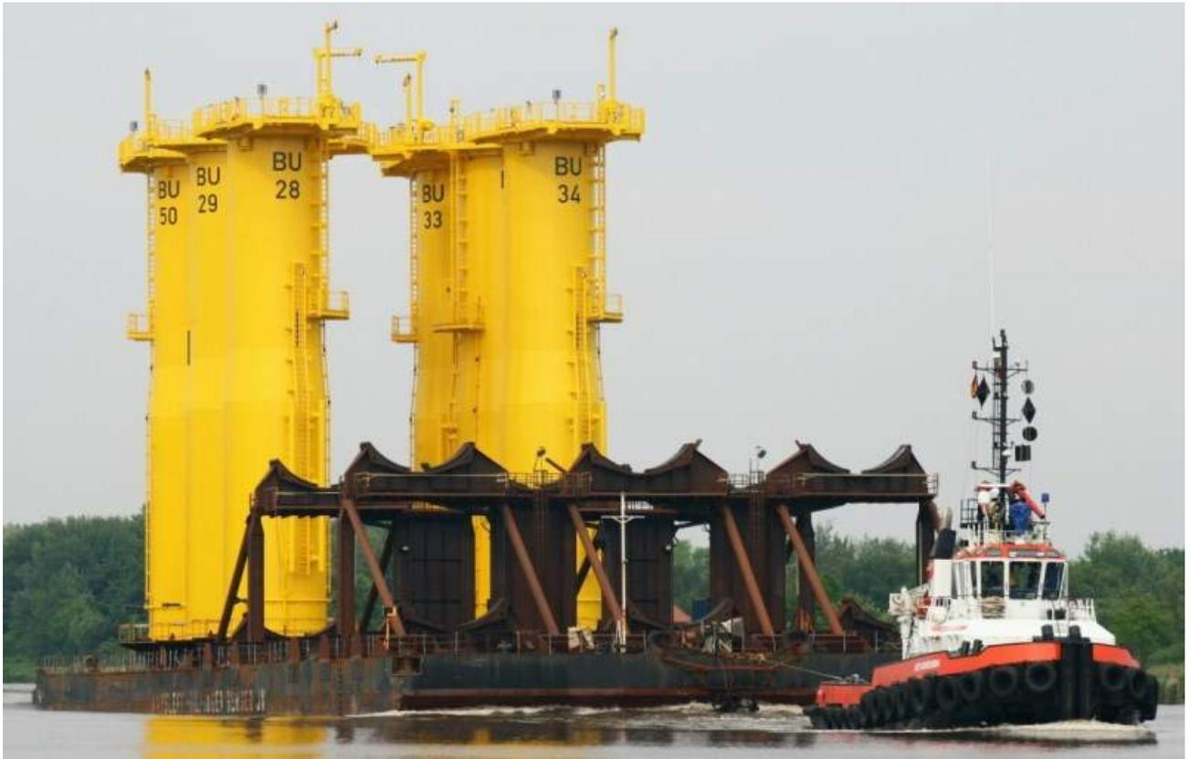
*Figure 3-11 None-Propelled Cargo Barge*
