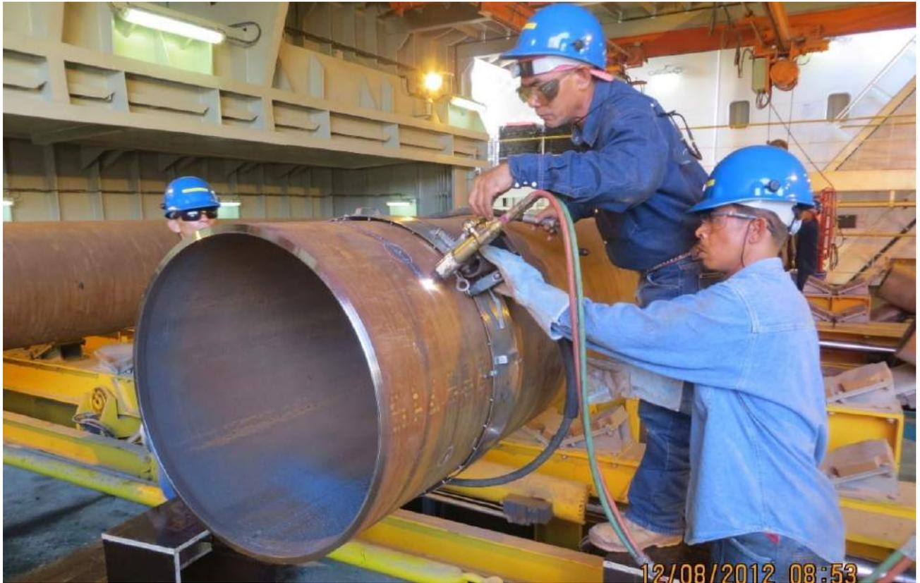
*Figure 6-143 Oxy Fuel Cutting Tools (Semi-Automatic)*
