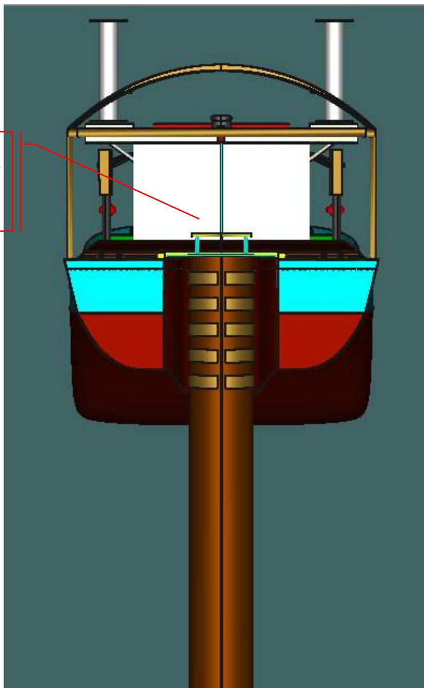
Figure 6-135 Both Cranes are connected to the monopile in tandem configuration
