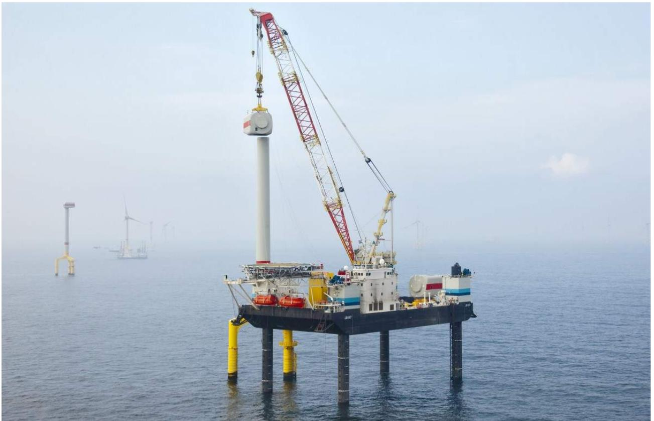
*Figure 3-7 None-propelled Jack up Barge (JB-117)*
