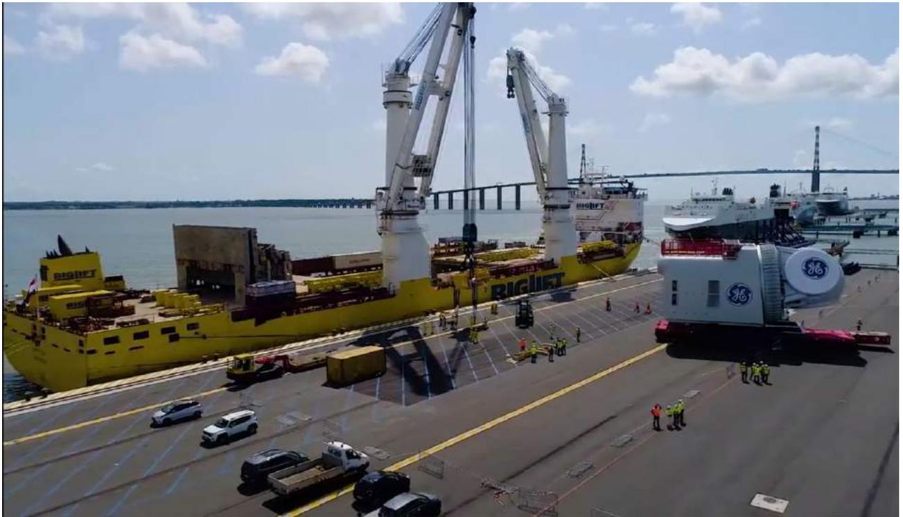
*Figure 6-7 Transportation of 12MW GE X-Heliade Nacelle to Quayside*
