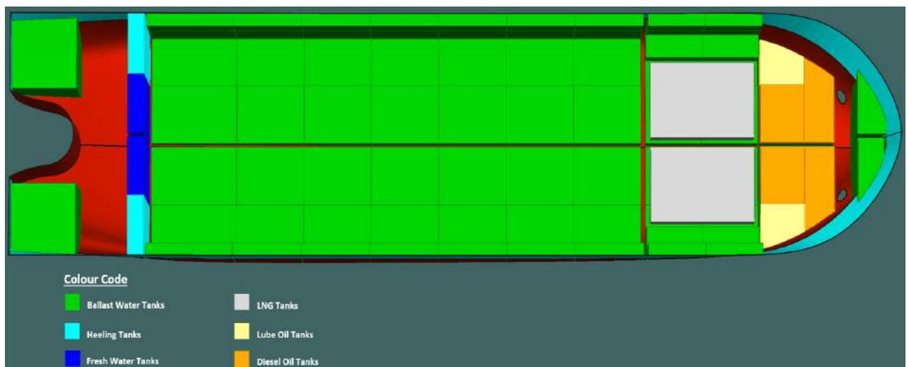
Figure 5-20 Plan of Tanks of Decom Tools Vessel
