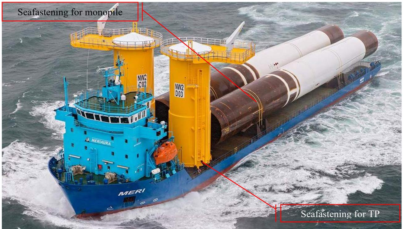
Figure 6-55 Conventional Seafastening of TP and Monopile
