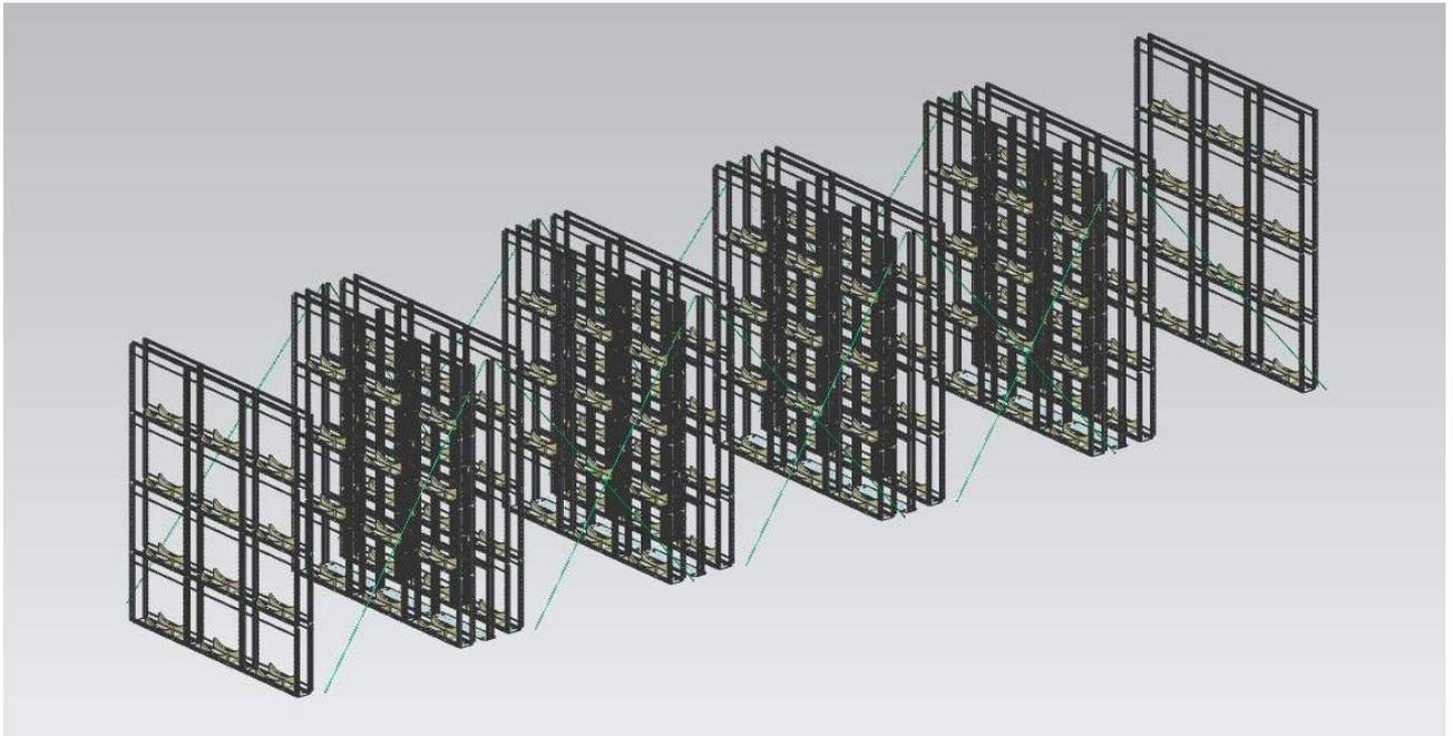
Figure 6-61 Blade's Seafastening of the Decom Tools Vessel
