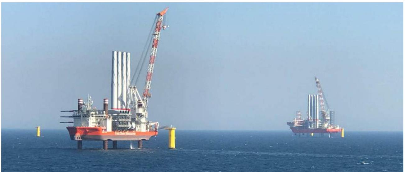
*Figure 3-28 Installation of OWP with Pendulum Config. (4 Set of WT in each Campaign)*
