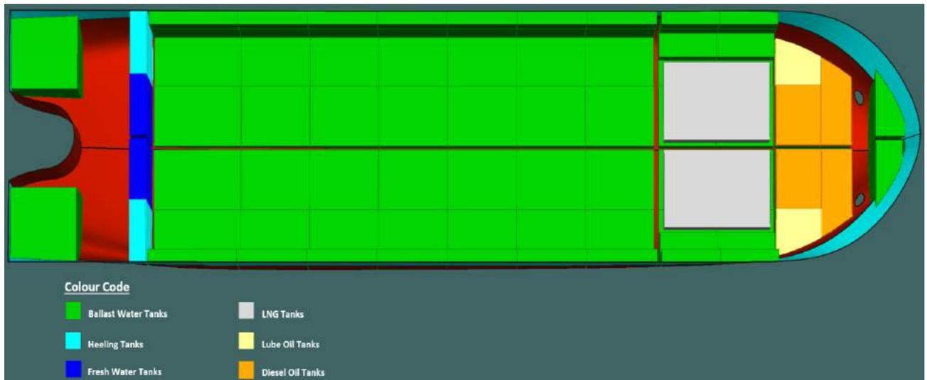
Figure 7-9 Plan of Tanks of Decom Tools Vessel
