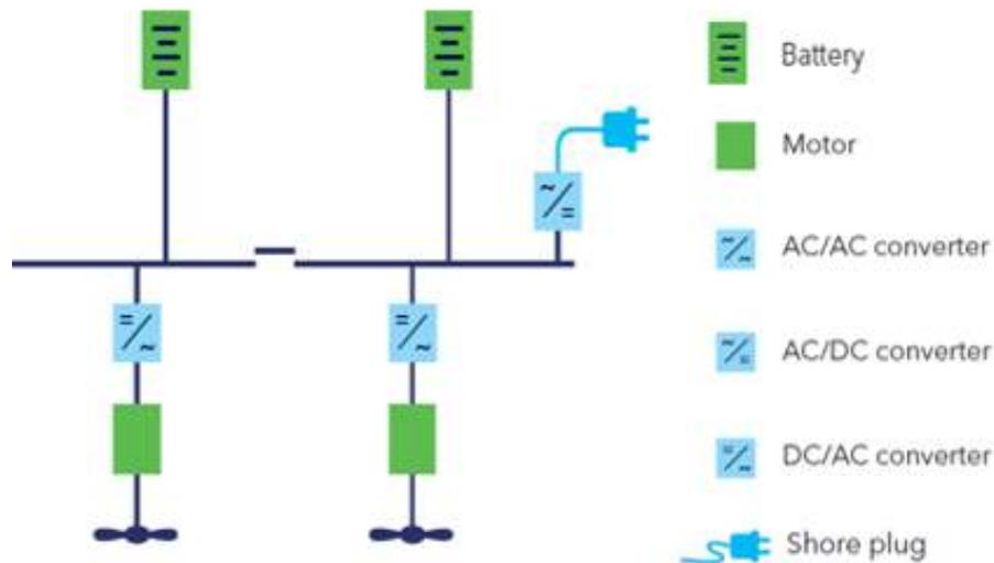
Figure 4-35 Battery Propulsion
