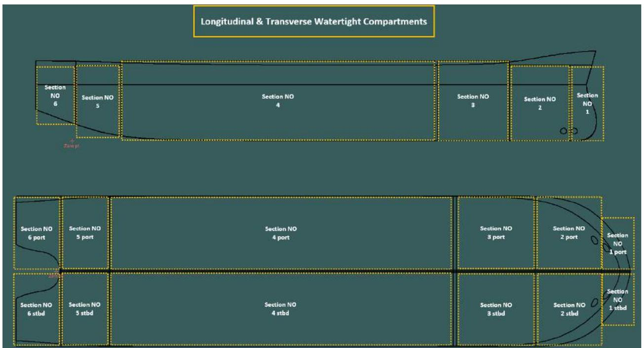
Figure 5-18 Longitudinal and Transverse Watertight Compartment
