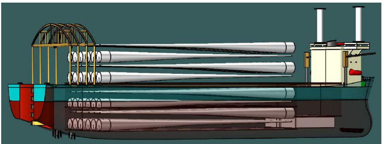
Figure 6-48 Perspective View of Load of 12MW Blade with Decom Tools Vessel
