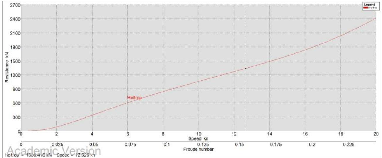
Figure 5-62 Correlation Between Speed and Resistance at Draft of 6 meters
