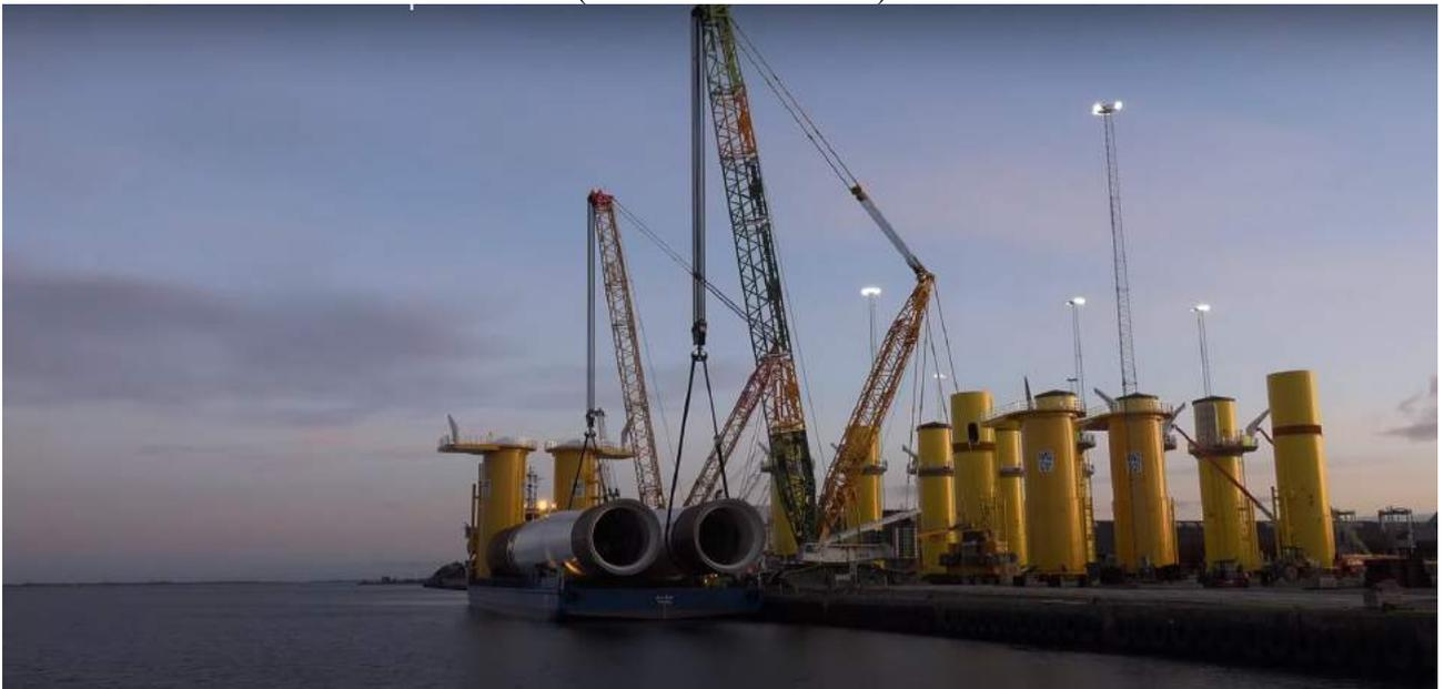
*Figure 3-22 Aura Heavy Load Carrier Loaded with 2 Monopiles+2 TP*
