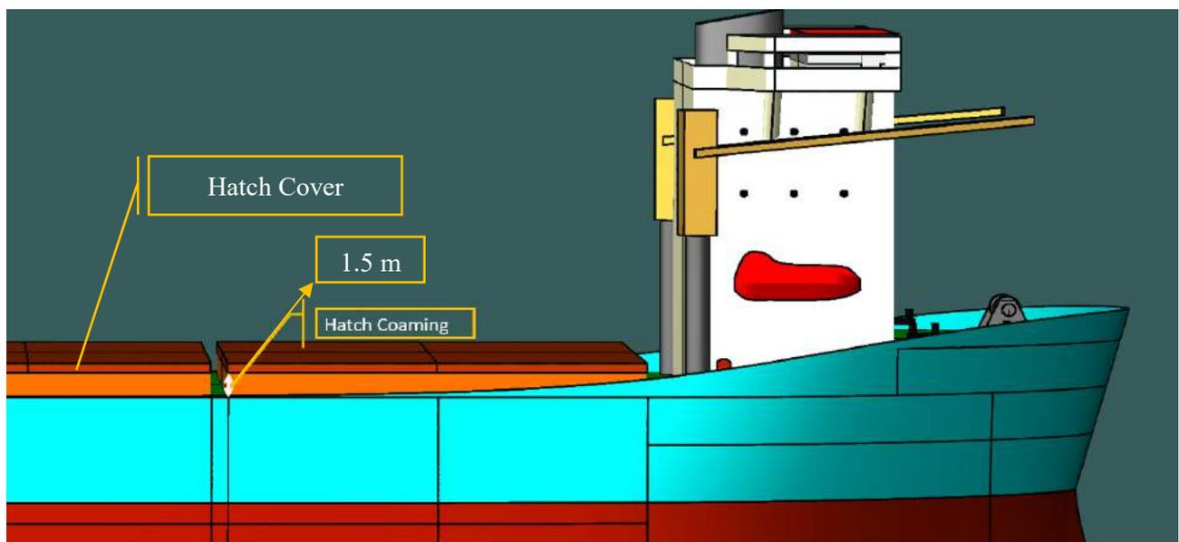
Figure 5-91 Hatch Coaming
