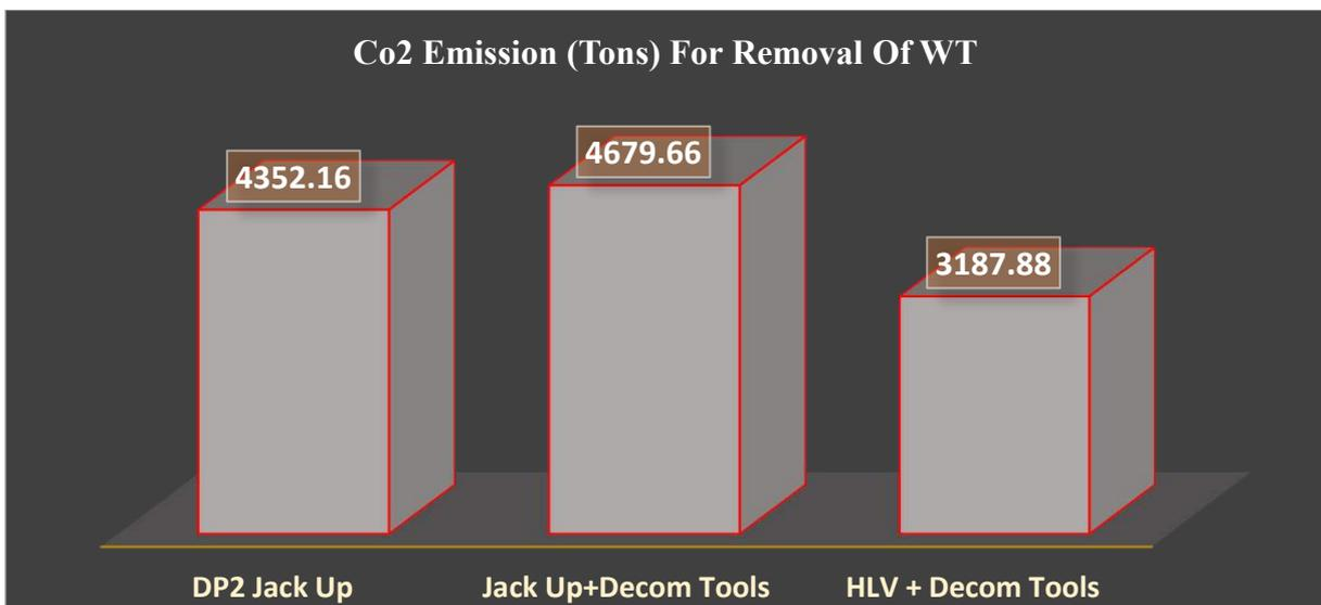
Figure 3-39 CO2 Emission of Various Logistic Configuration in Decommissioning of Noblewind OWP
