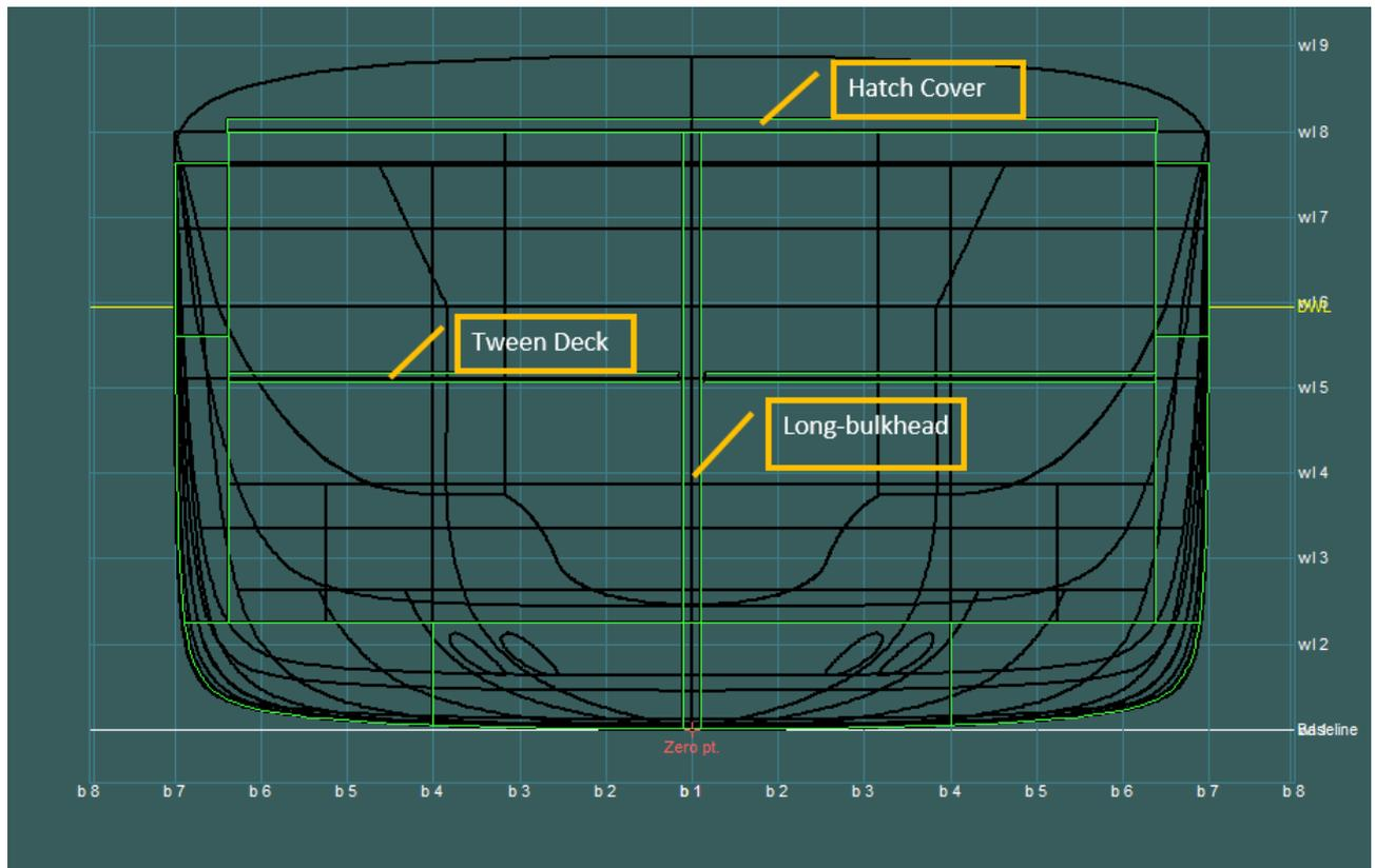
Figure 5-12 Aft View of Decom Tools Vessel's Deck
