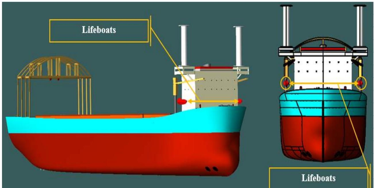
Figure 5-85 Perspective and Front (Bow) View of Lifeboats
