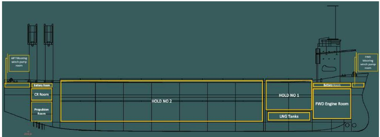
Figure 5-83 Engine room, Propulsion Room and Battery Room
