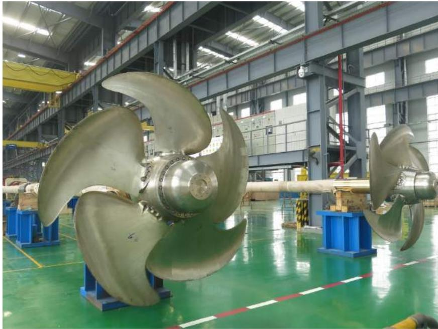
Figure 4-13 Pitch Controllable Propeller
