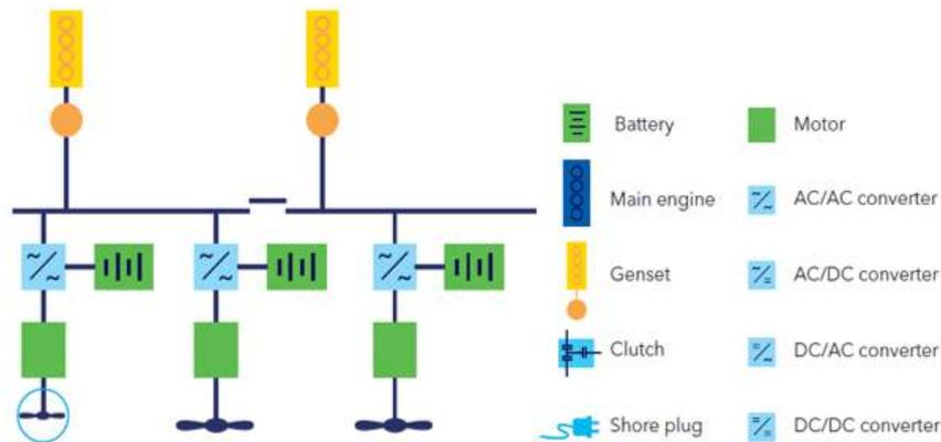
Figure 4-33 Hybrid Battery Propulsion, with Distributed Batteries
