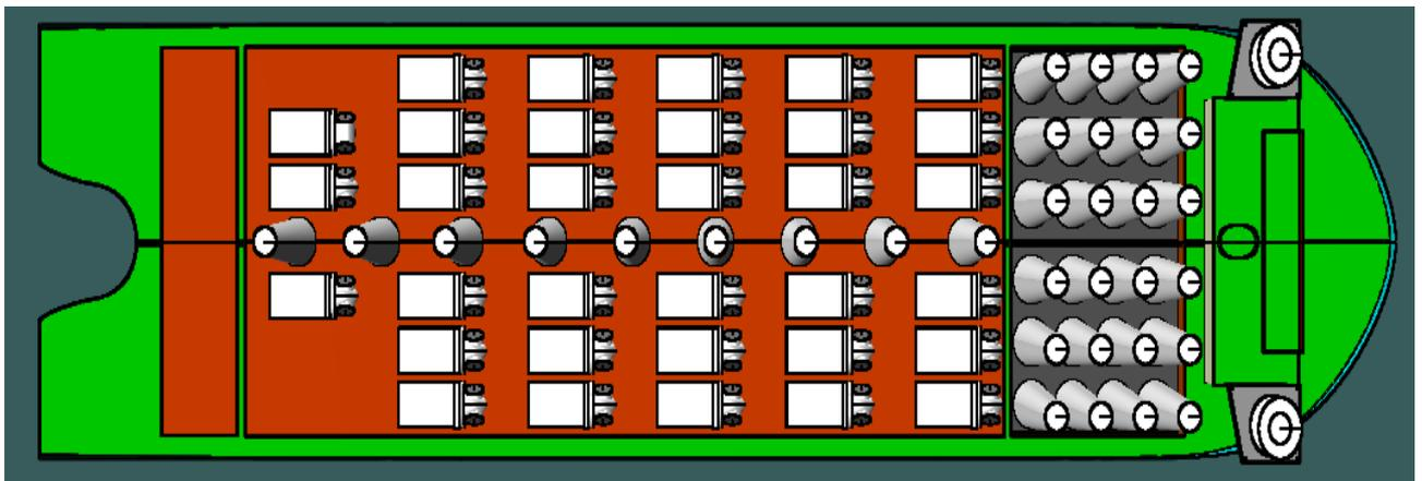
Figure 6-41 Top View of Load out of 3.6 MW Wind Turbine
