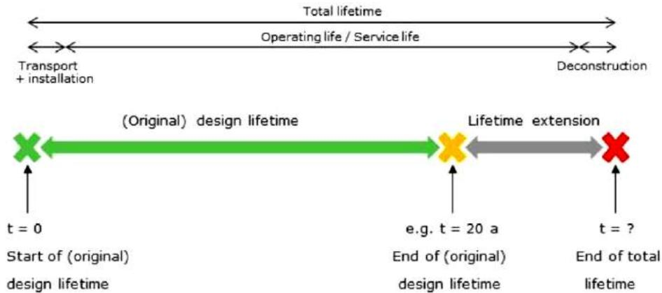
Figure 1-1 Definition of Lifetime & Lifetime Extension
