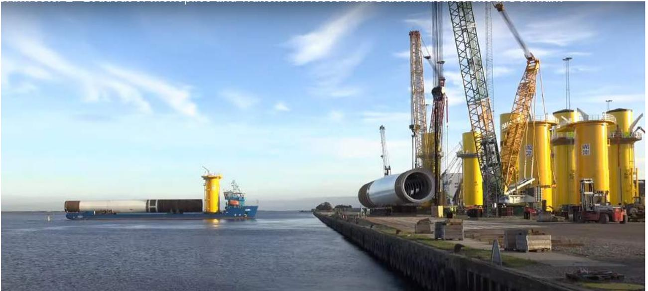
*Figure 3-21 Aura Heavy Load Carrier Loaded with 2 Monopiles+2 TP*
