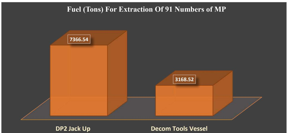
Figure 6-174 Comparison of Fuel Consumption for MP Extraction
