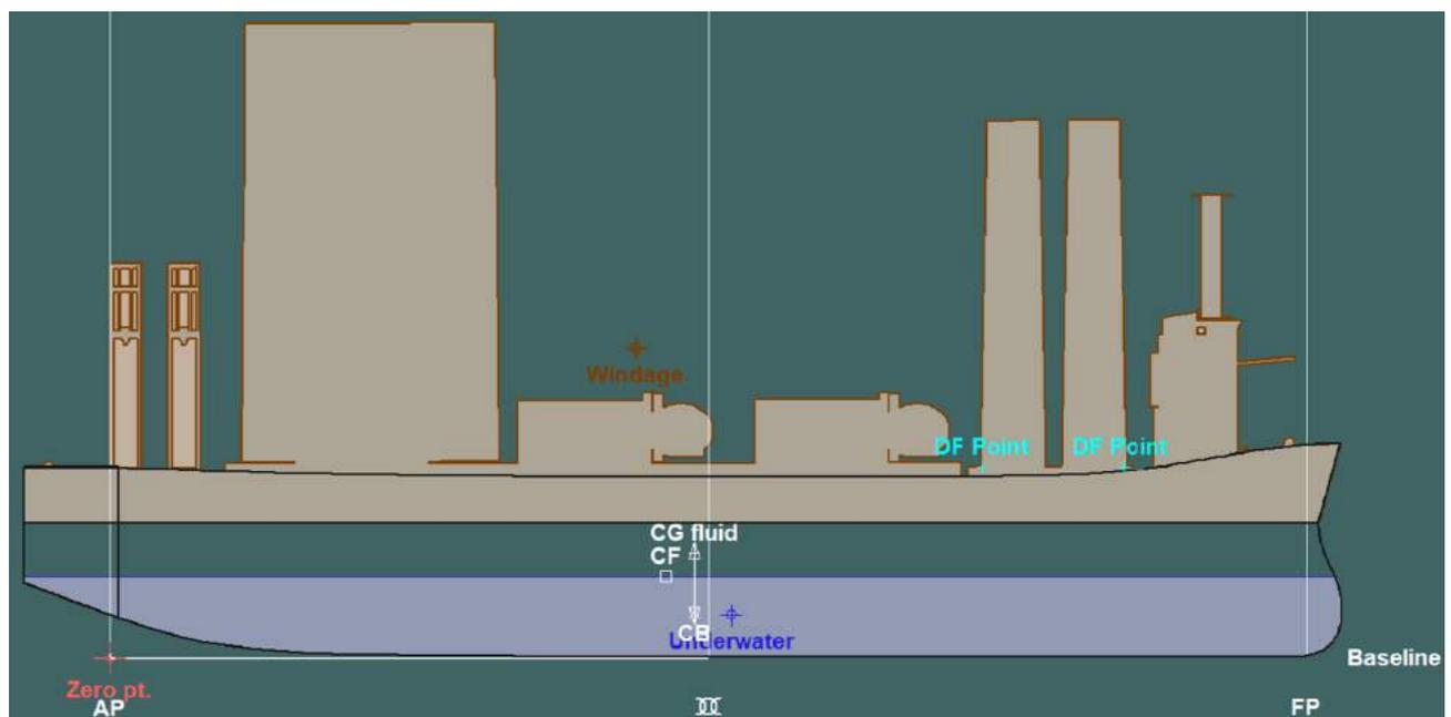
Figure 7-26 Decom Tools Vessel Windage Area After Loading 8 x 12MW WT
