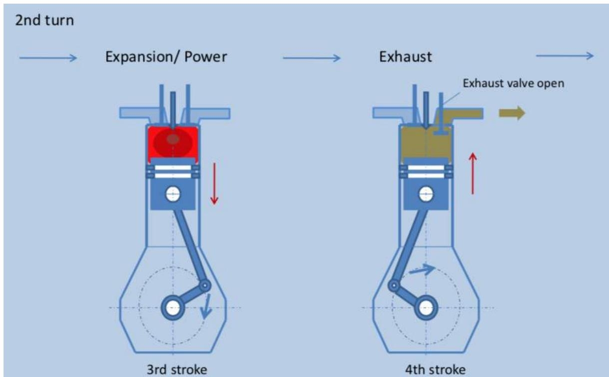
Figure 4-4 Third and Fourth Stroke of 4-Stroke Engine
