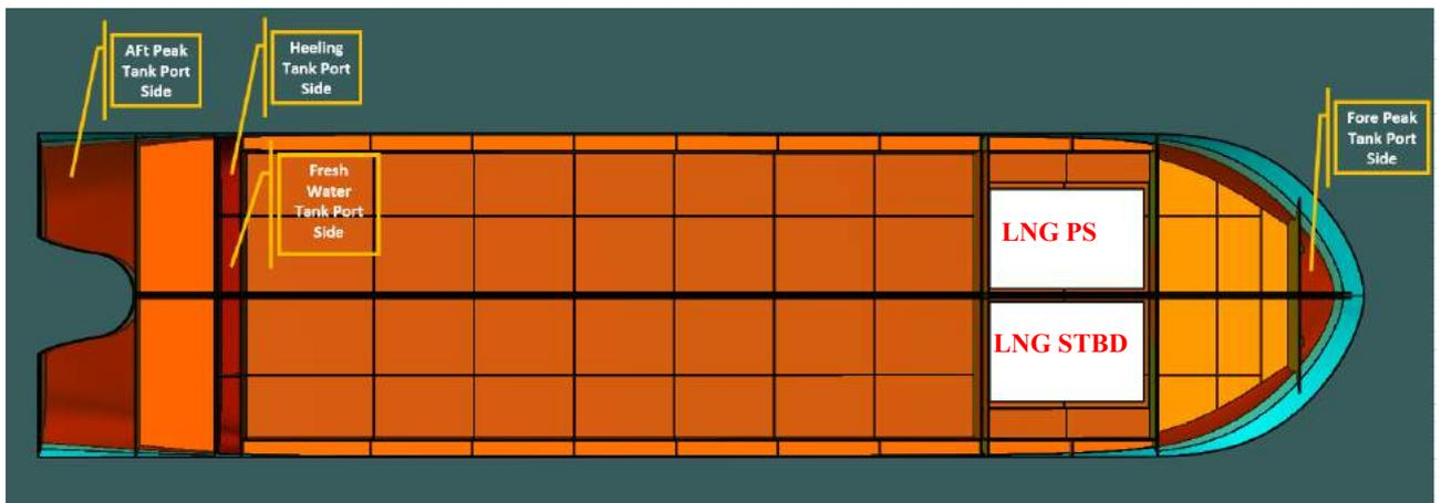
Figure 5-23 Top View of Decom Tools Vessel's Tanks
