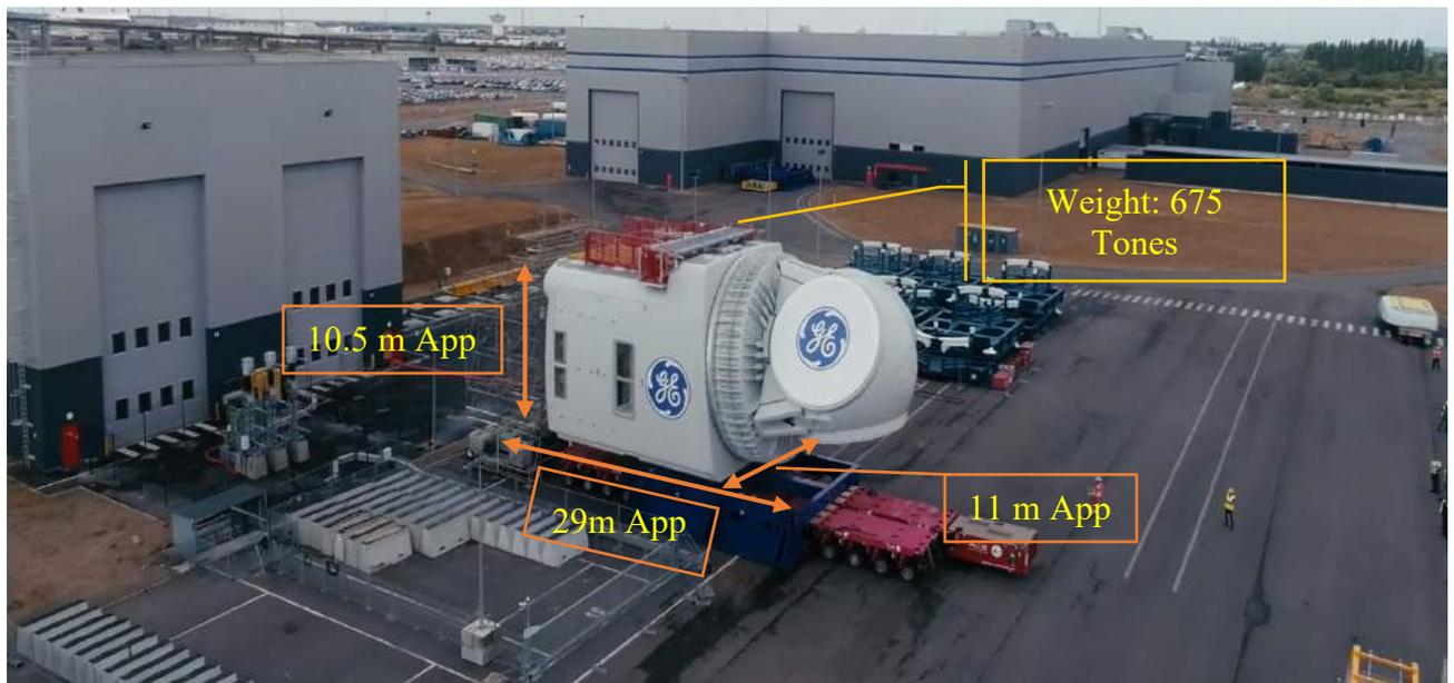
Figure 6-6 Transportation of 12MW GE X-Heliade Nacelle (Energyfacts.eu 2019)
