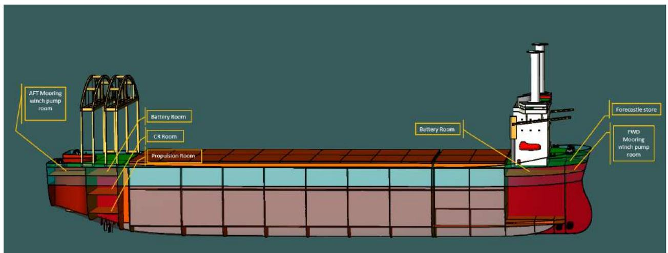
Figure 5-84 Engine room, Propulsion Room and Battery Room
