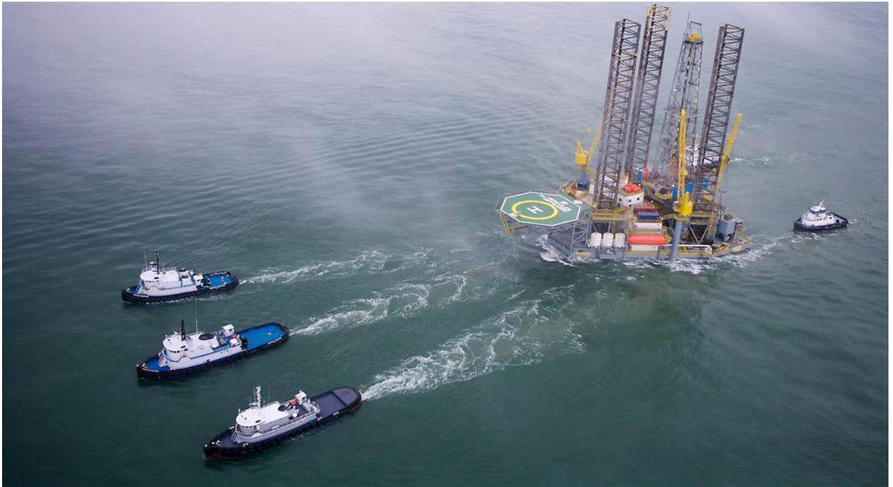
*Figure 3-6 Towing of Jack up Barge*
