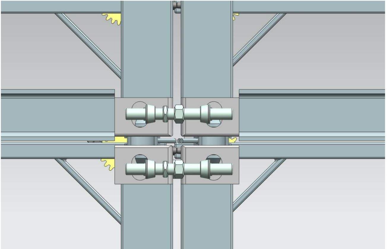
Figure 6-66 Connection of Blades Rack
