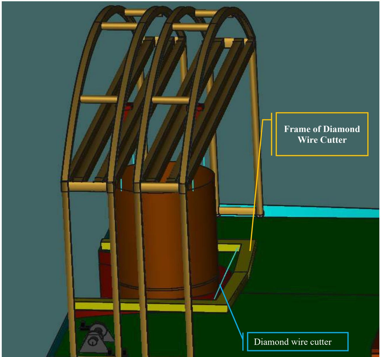
Figure 6-149 Completion of Cutting of Monopile
