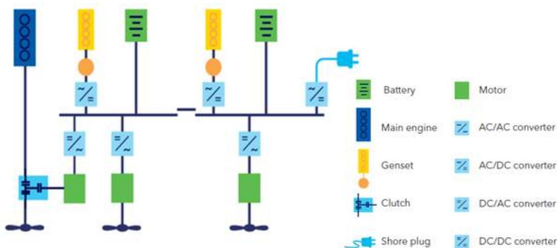
Figure 4-34 Hybrid Battery, Electrical, Mechanical Propulsion & DC Distribution
