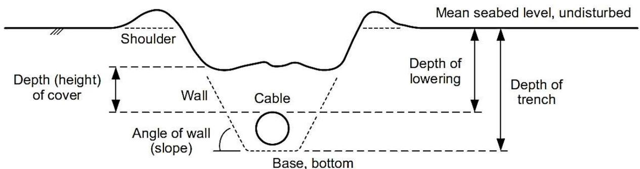
Figure 6-178 Burial of Submarine Cables (DNV.GL 2016)
