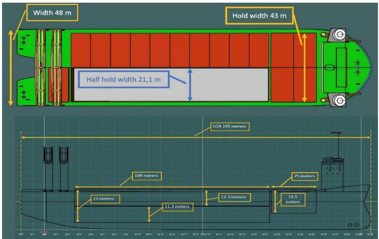
Figure 5-8 Dimension of Decom Tools Vessel
