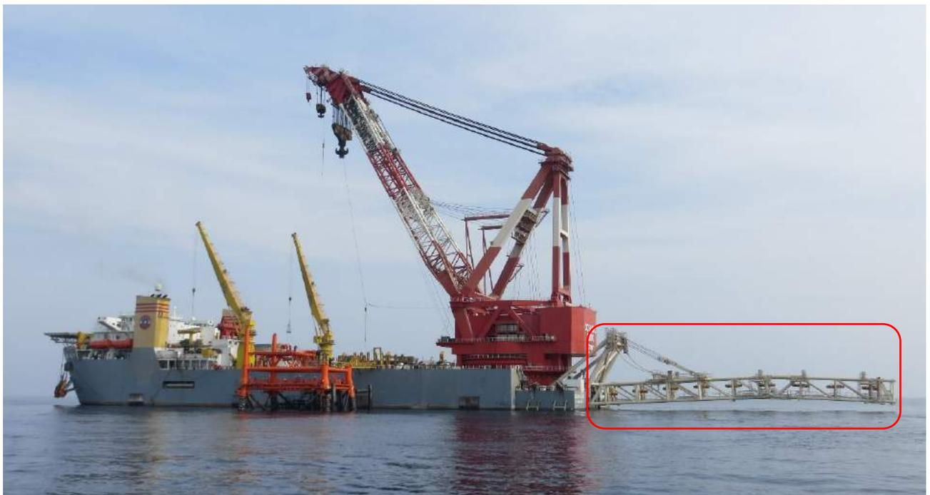
*Figure 6-206 Stinger of the Special Purpose Vessel*
