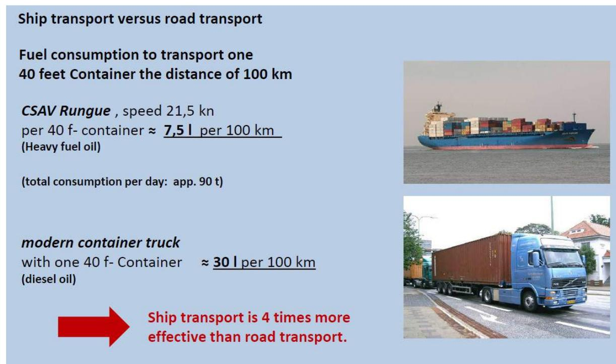
Figure 6-1 Shore Transportation VS offshore Transportation (Meyer 2019)
