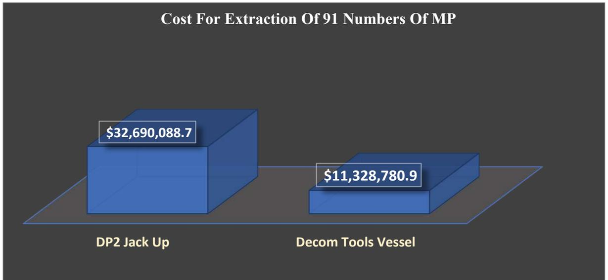
Figure 6-173 Comparison of Cost for MP Extraction
