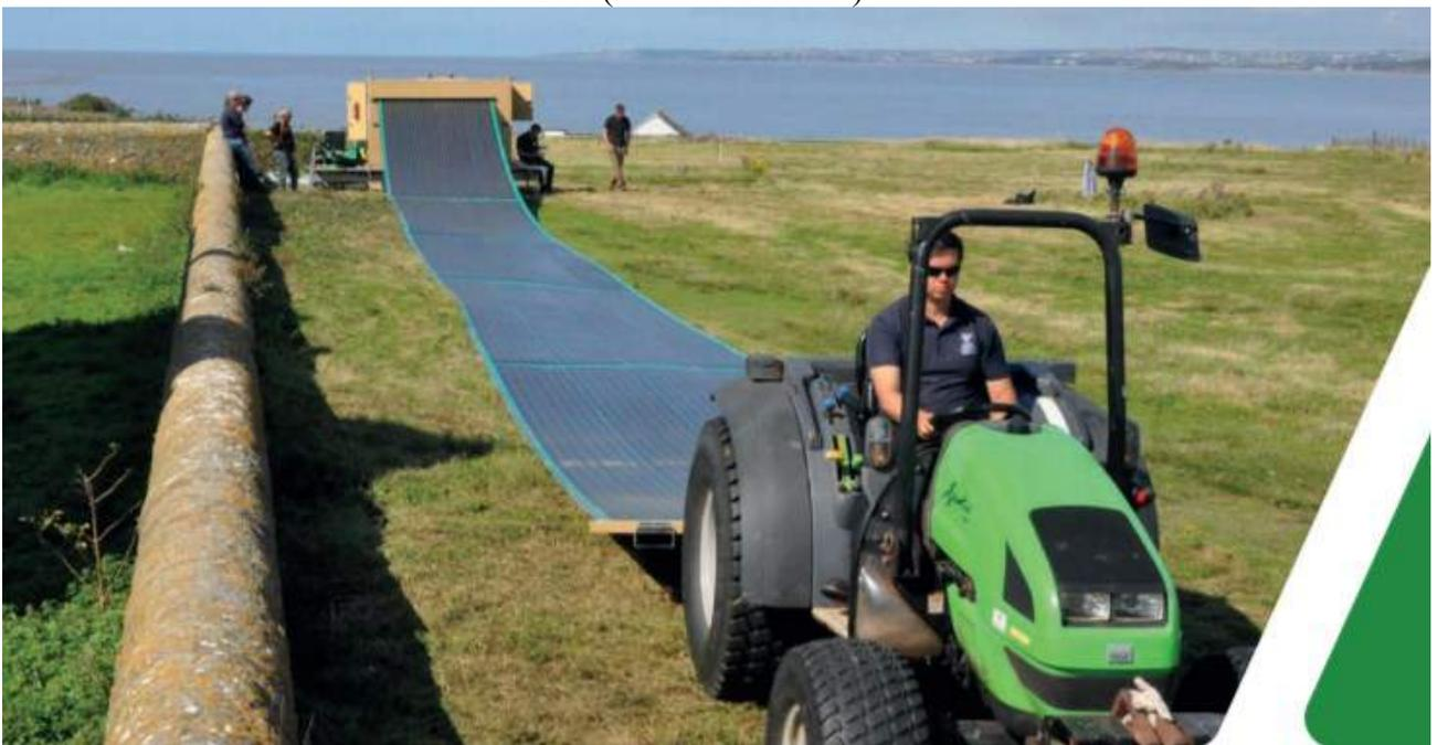
*Figure 5-58 Rollable and Portable Solar Panel (Renova Gen n.d.)*
