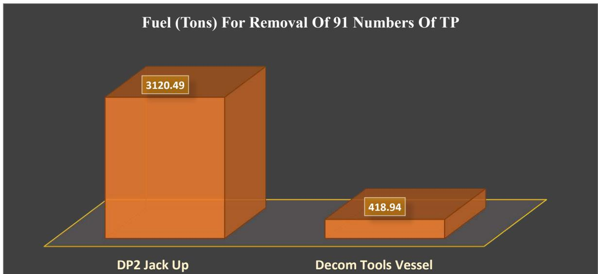
Figure 6-114 Fuel Consumption During Removal of 91 Number of TP
