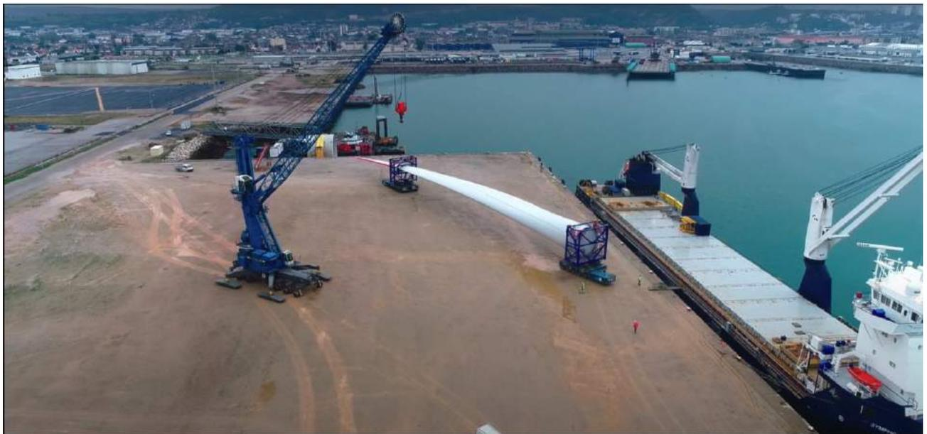
*Figure 6-12 Transportation of 12 MW GE X-Heliade Blade (LM Wind Power, 2019)*
