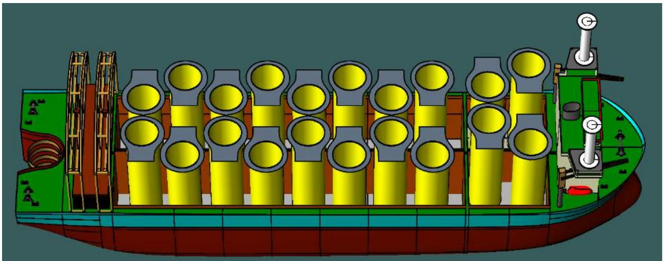
*Figure 6-45 Top View of Load of 12MW TP with Decom Tools Vessel*
