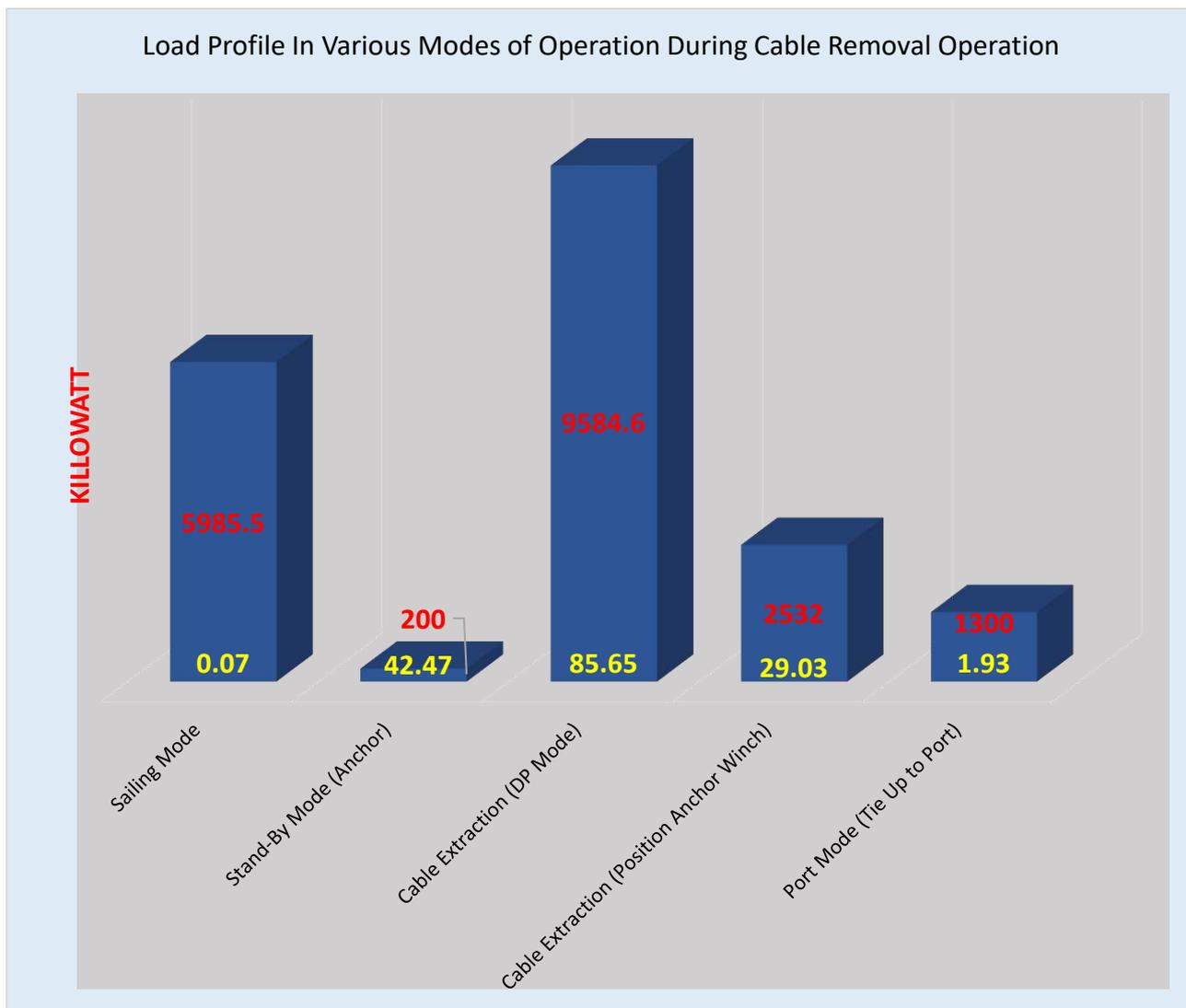
Figure 5-73 Load Profile for Cable Removal Operation
