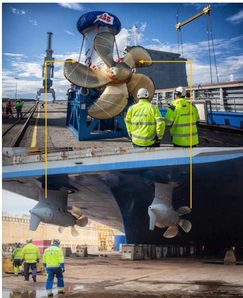
Figure 4-15 ABB Azipod Propeller Installed on a Ferry
