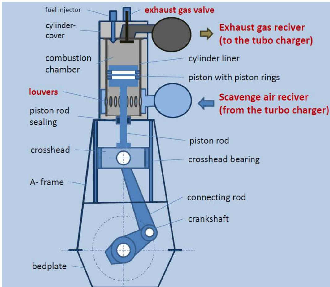
Figure 4-5 Cross Section of 2-Stroke Crosshead Engine
