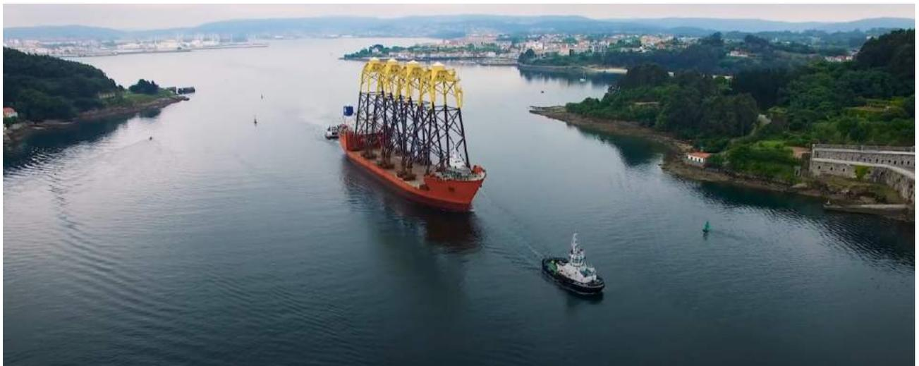
*Figure 3-24 Transportation Of Wikinger Wind Farm Jacket To The Field By A Heavy Load Career*
