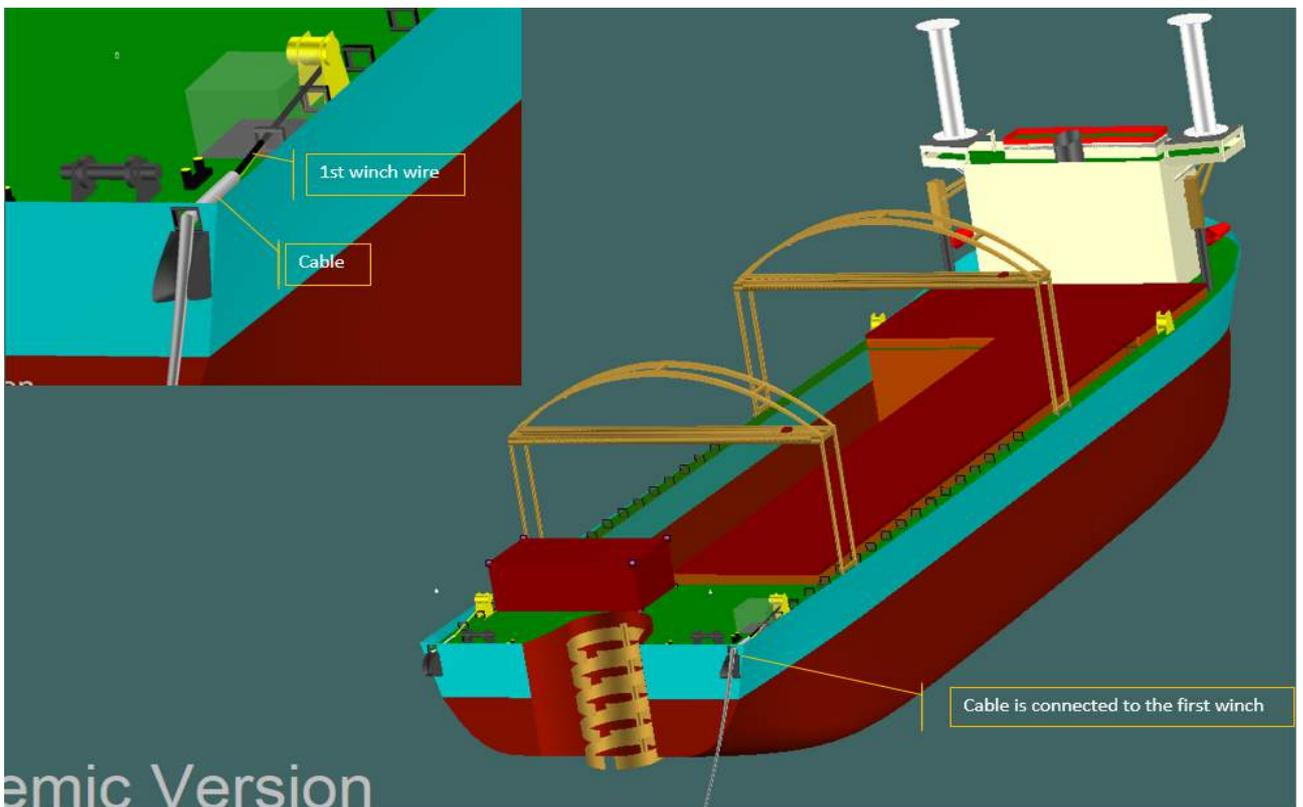
Figure 6-227 Cabled is pulled by first winch onto the deck
