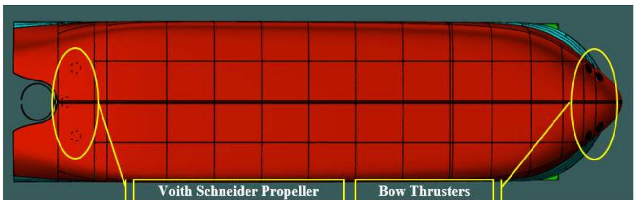
Figure 5-70 Bottom View of Decom Tools Vessel
