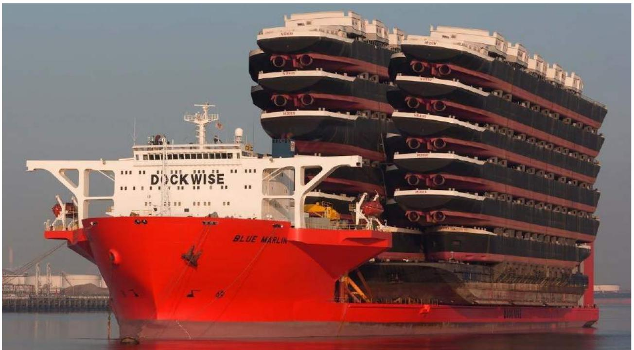
*Figure 3-12 Heavy Load Carrier Semi-Submersible Ship*
