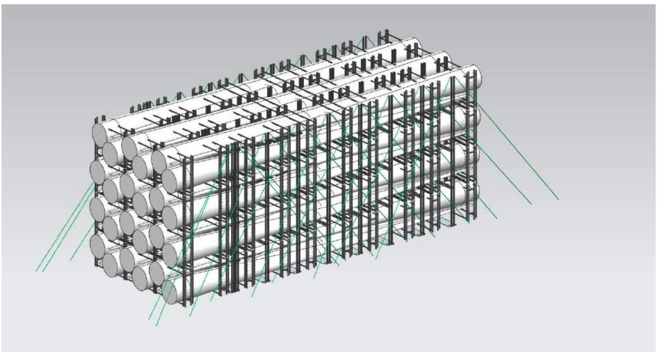
Figure 6-82 Optimum Arrangement of Rack and Cutting Tools for 3.6 MW blades
