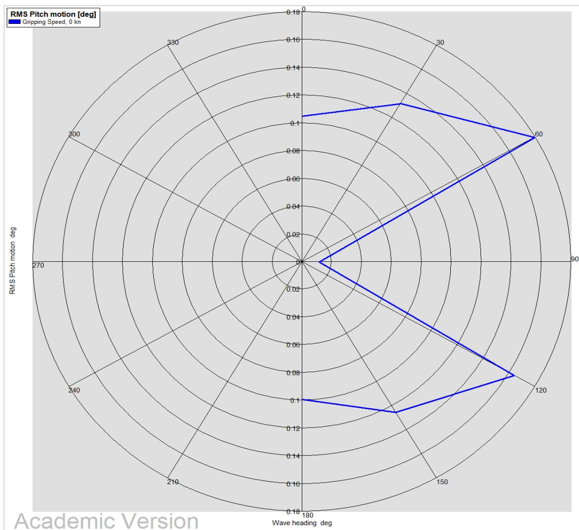
Figure 8-7 Pitch Motion at COG – Slight Sea state
