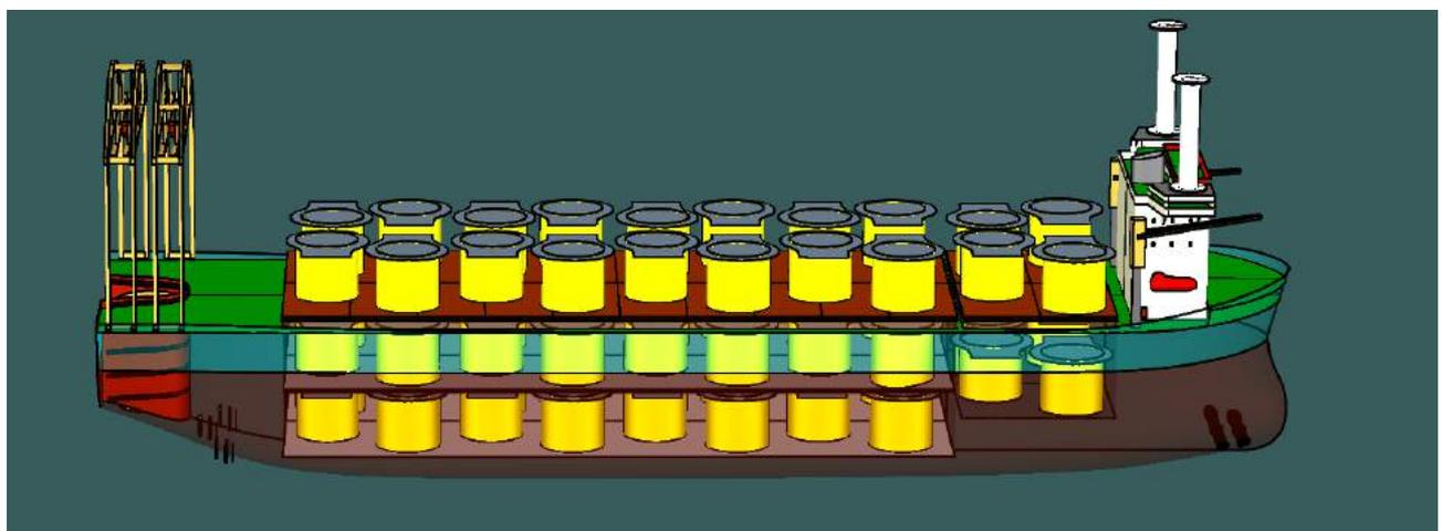
Figure 6-110 TPs loading arrangement (Bird's Eye View)
