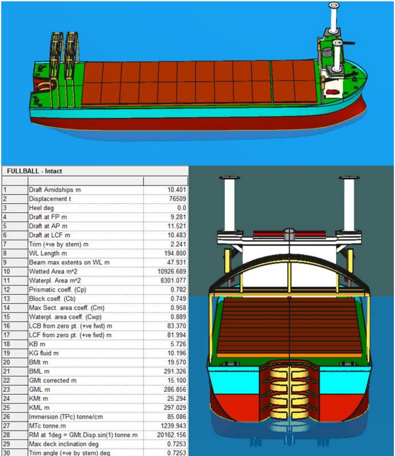
Figure 7-12 Decom Tools Vessel at full Ballast Equilibrium
