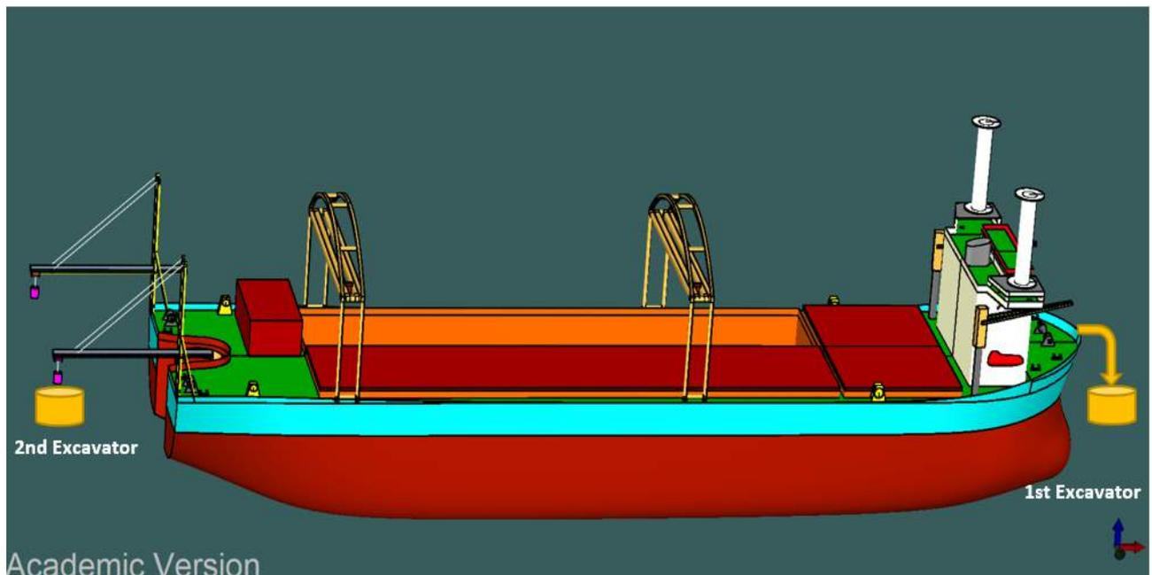
Figure 6-207 Decom Tools LARS Structure (Movable Overhead Crane)
