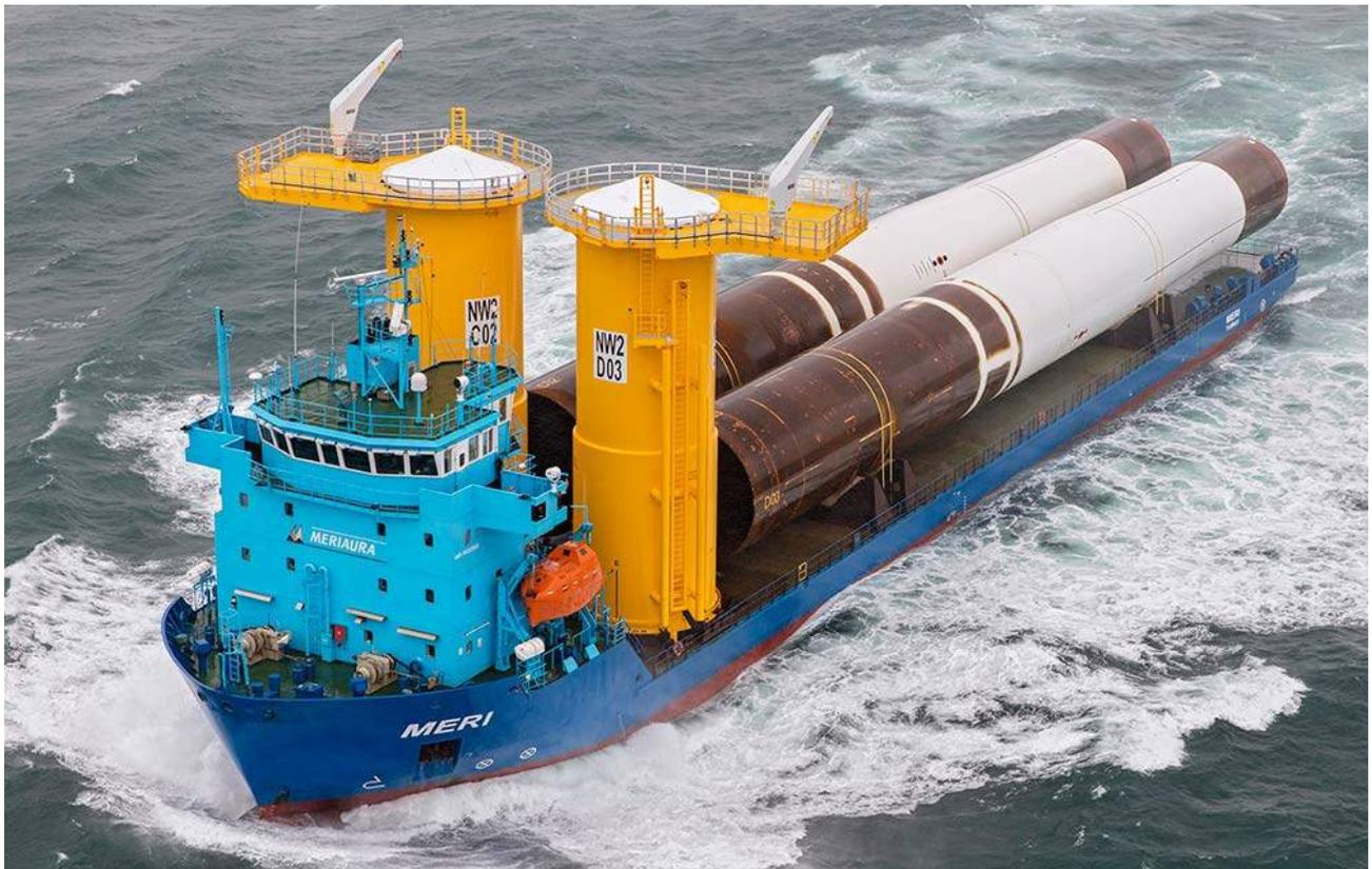
*Figure 6-171 Lashing of the Monopile*
