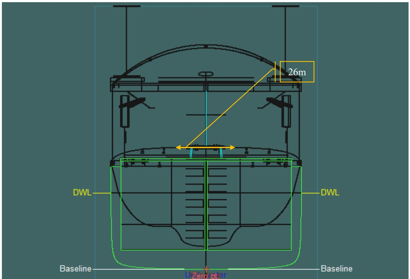
Figure 6-123 Location of Pile Extraction System
