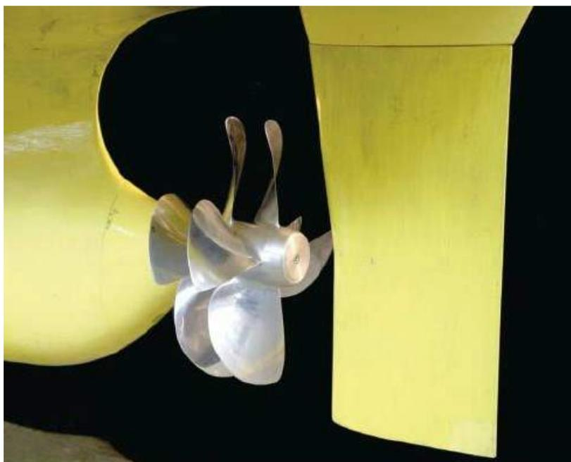
*Figure 4-11 Tandem Propeller*
