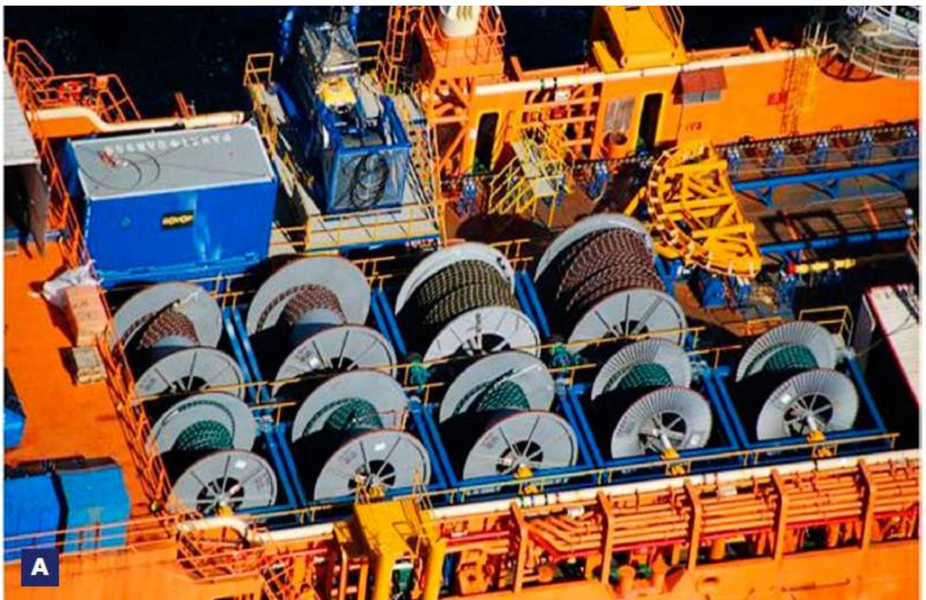
Figure 6-203 Cable Drum on the CLV (Boskalis 2019)
