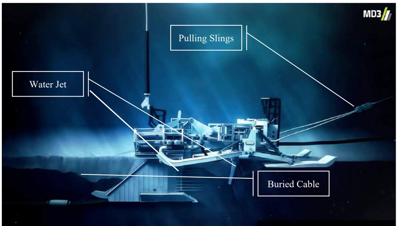
Figure 6-186 Cable Plough (SMD - Subsea Technology 2014)
