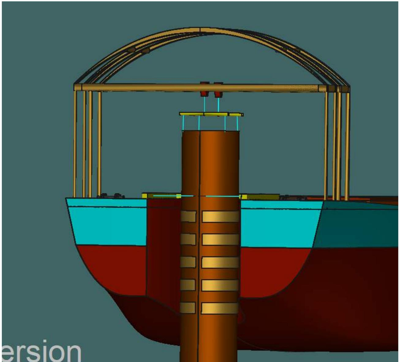
Figure 6-146 Commencement of Cutting with Diamond Wire Cutter
