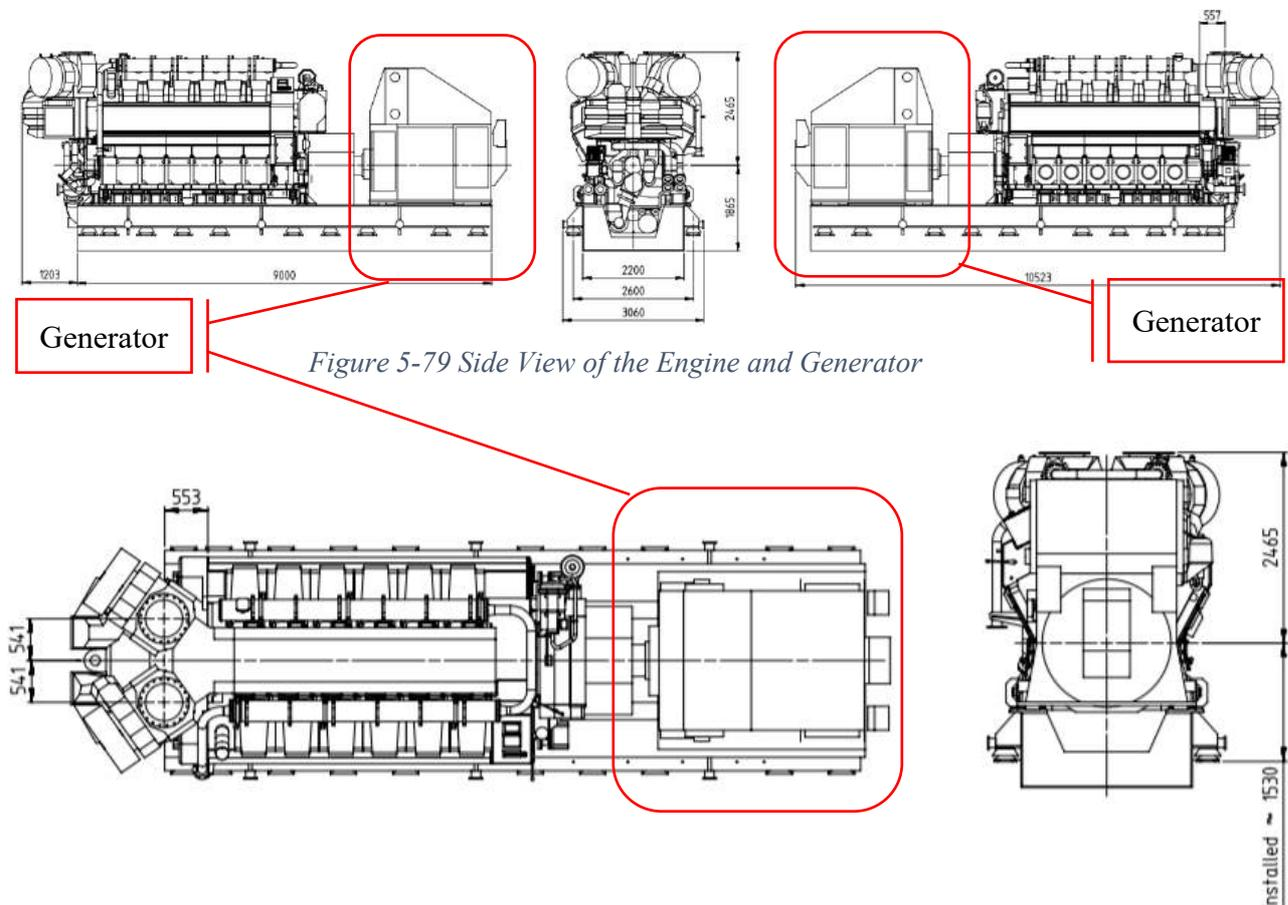
Figure 5-79 Side View of the Engine and Generator
