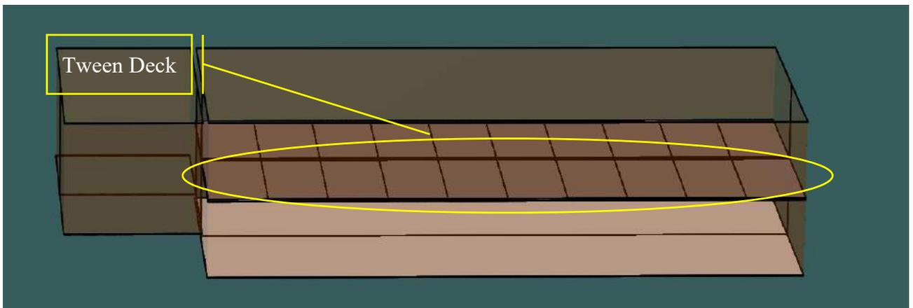
Figure 5-15 Holds and Tween Deck of Decom Tools Vessel
