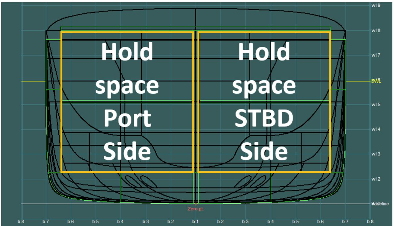
Figure 5-16 Aft View of Decom Tools Vessels Hold
