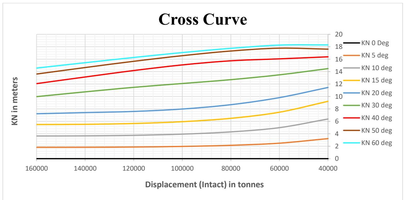
Figure 7-18 KN Curves of Decom Tools Vessel
