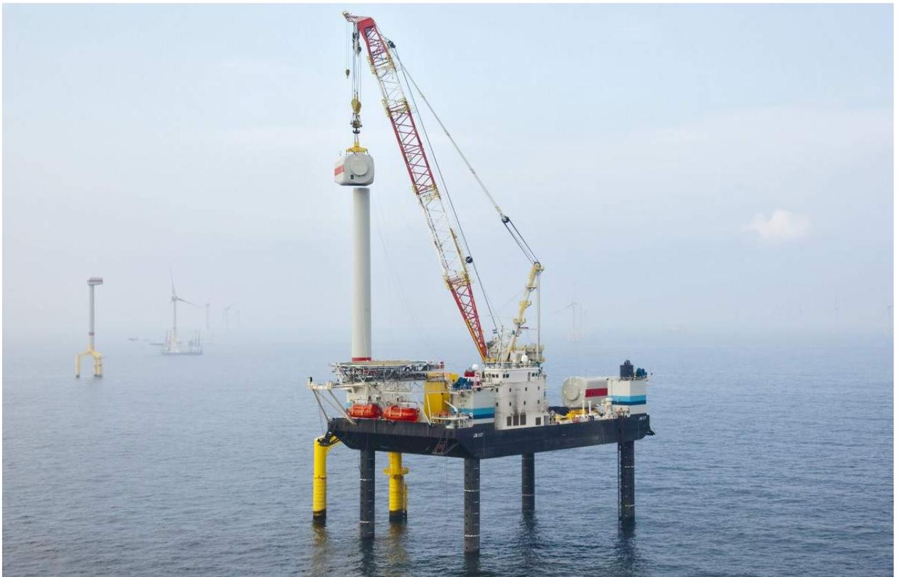
*Figure 3-7 None-propelled Jack up Barge (JB-117)*
