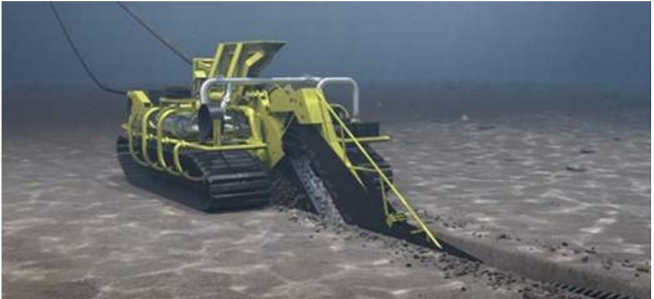
Figure 6-191 Mechanical Trencher
