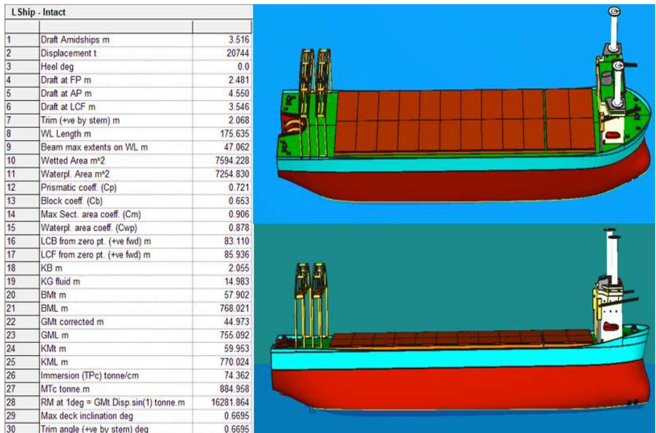
Figure 7-11 Decom Tools Vessel at Lightweight Equilibrium
