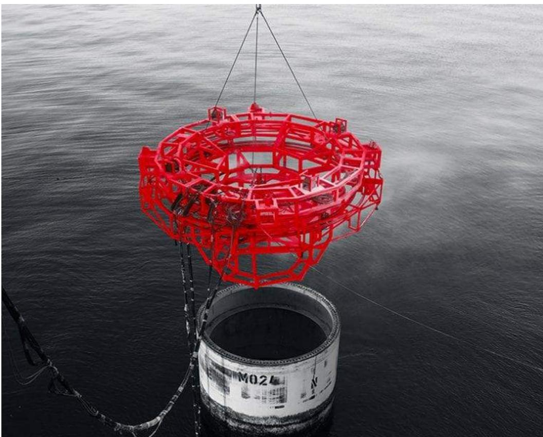
Figure 6-156 Marine Growth Removal Tool (CLAXTON n.d.)
