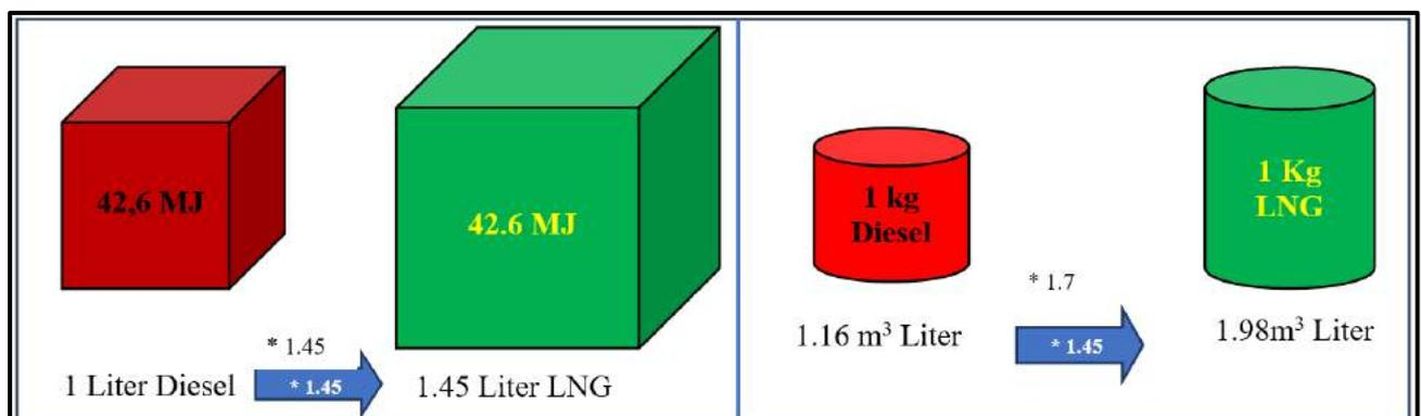
Figure 4-26 Volume and Calorific Value of Diesel Oil VS LNG
