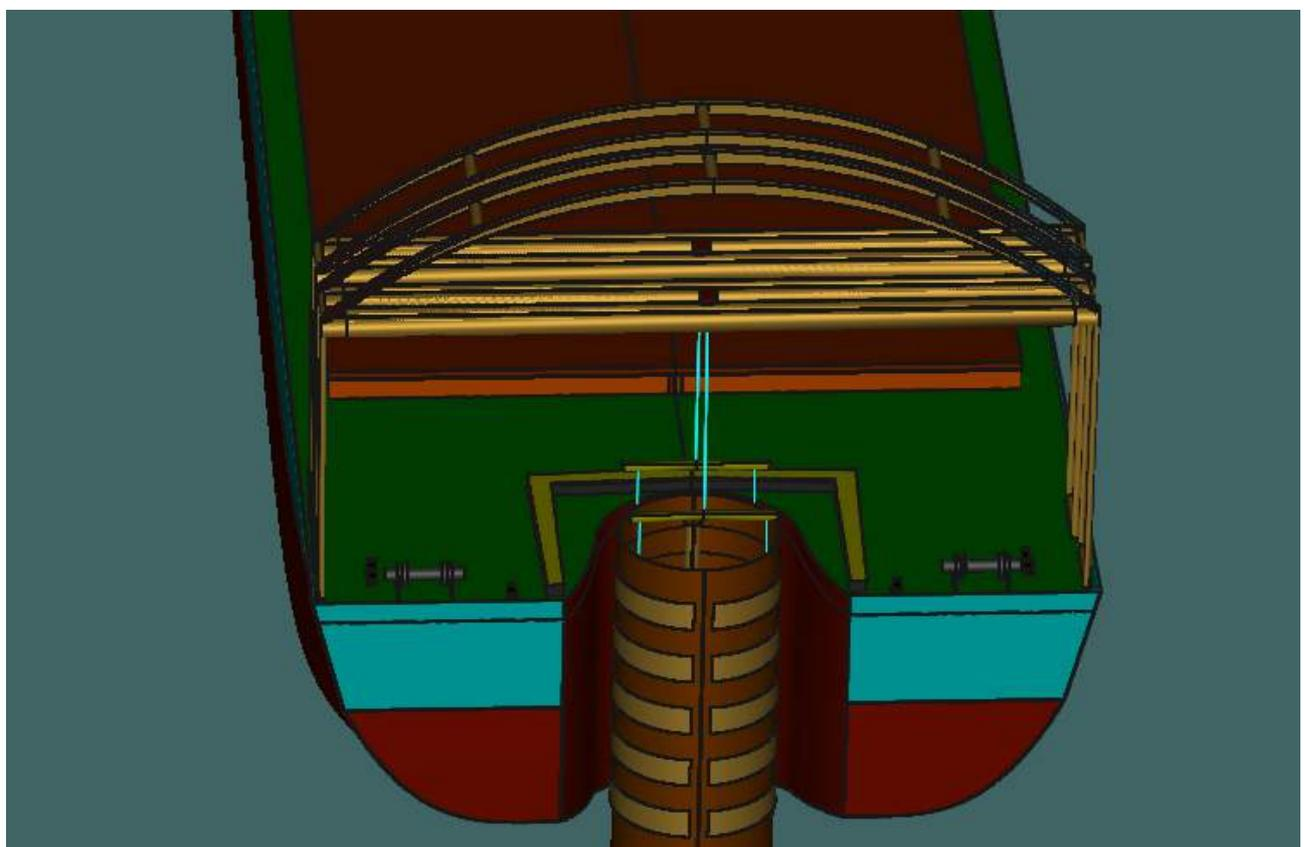
*Figure 6-137 Plan of Tandem connection of Cranes to the monopile and Spreader bar*
