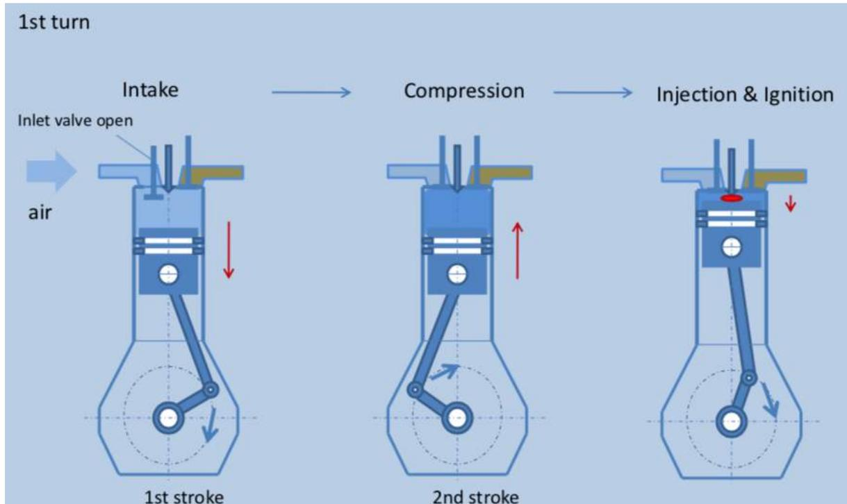
Figure 4-3 First and Second Stroke of 4-Stroke Engine
