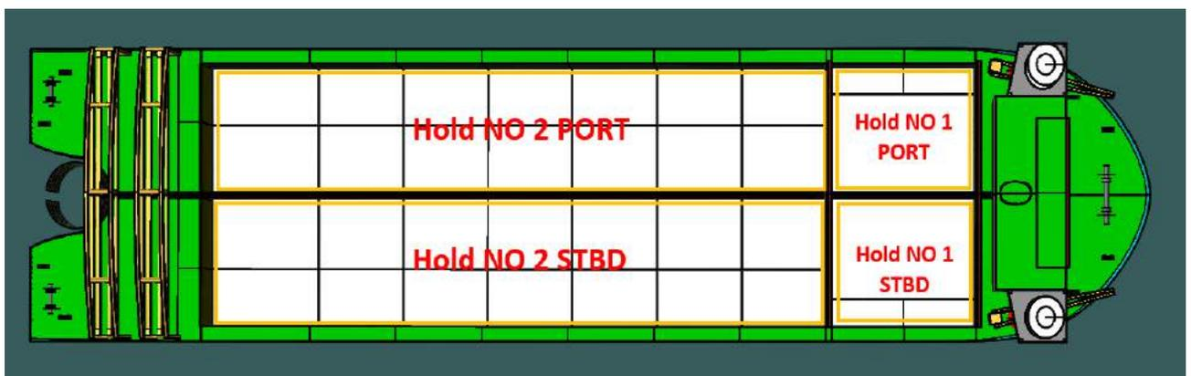
Figure 5-11 Decom Tools Vessel Holds
