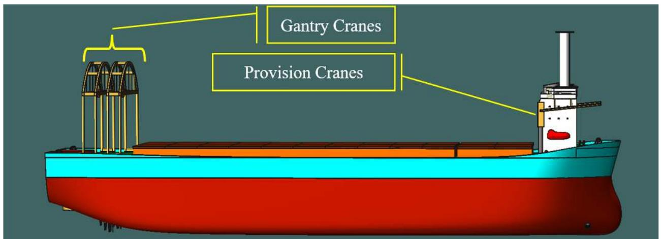
Figure 5-45 Cranes of the Decom Tools Vessel
