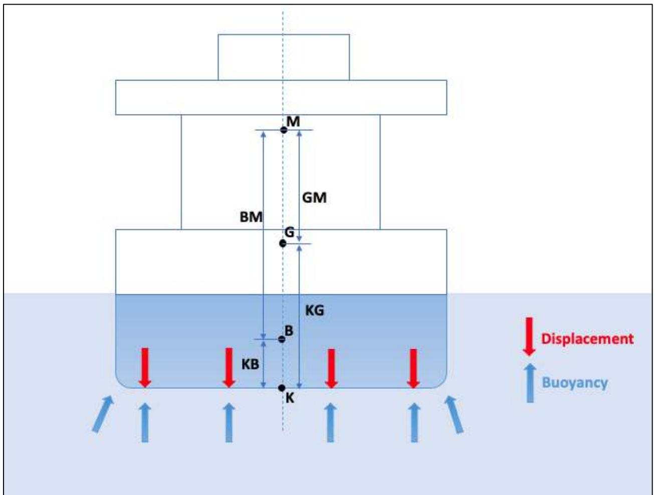
Figure 7-8 Displaying the M, GM, BM, B, KB & K
