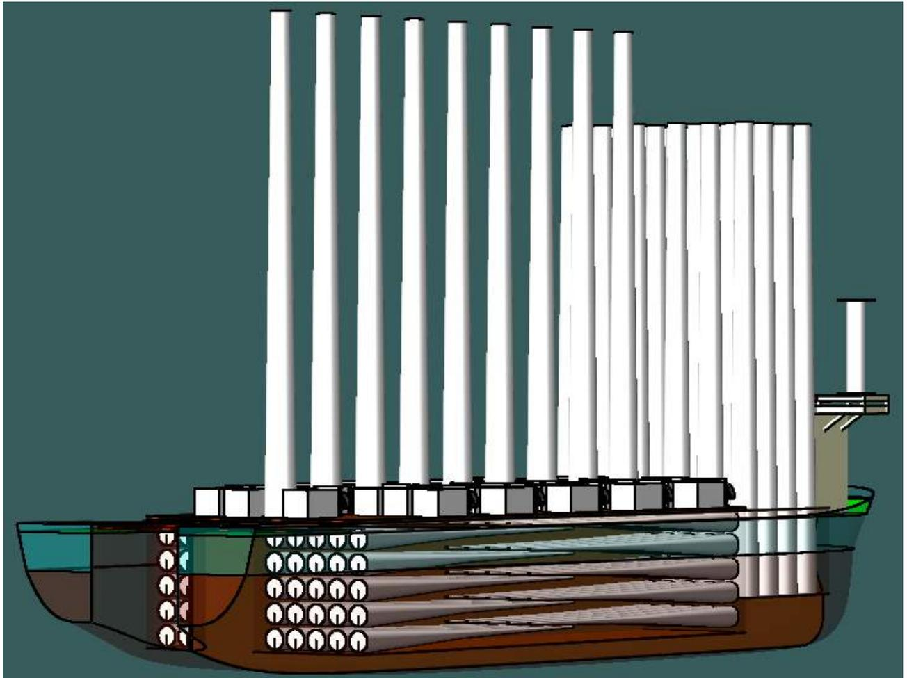
*Figure 6-44 Perspective view of Load out of 3.6MW Wind Turbine*
