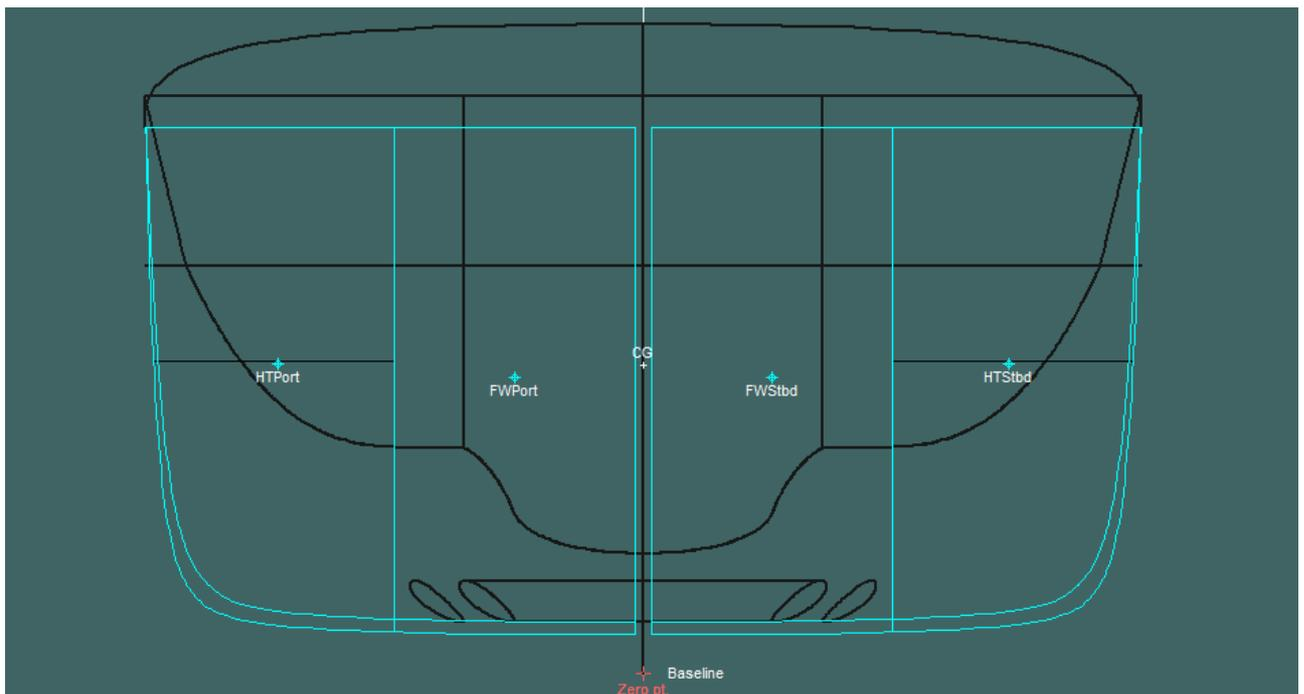
Figure 5-35 Back View of Fresh Water and Heeling Tank
