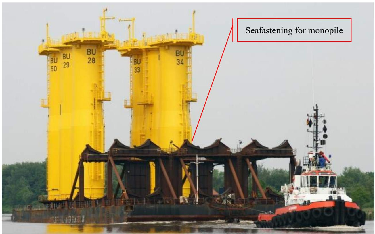
Figure 6-54 Conventional Seafastening of TP and Monopile
