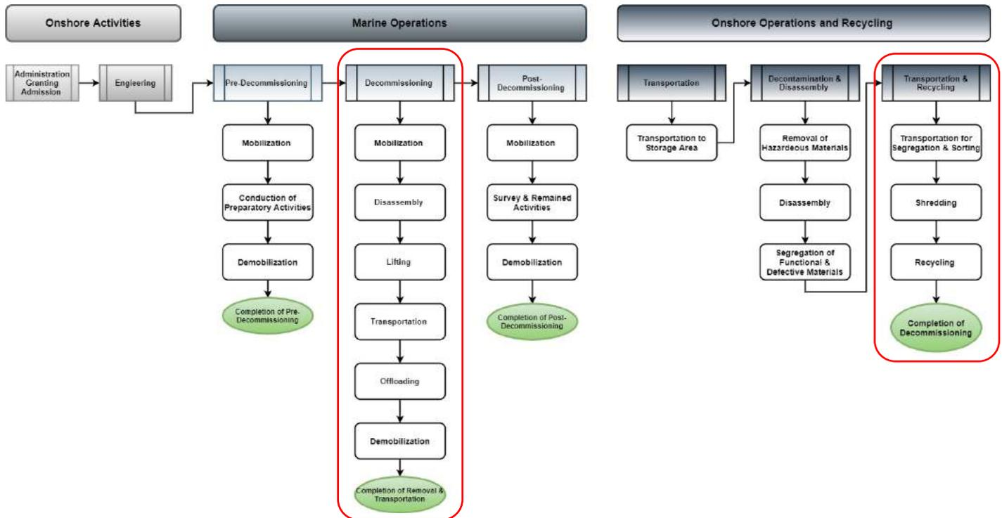
Figure 3-1 Overall Phases of Decommissioning of an OWP
