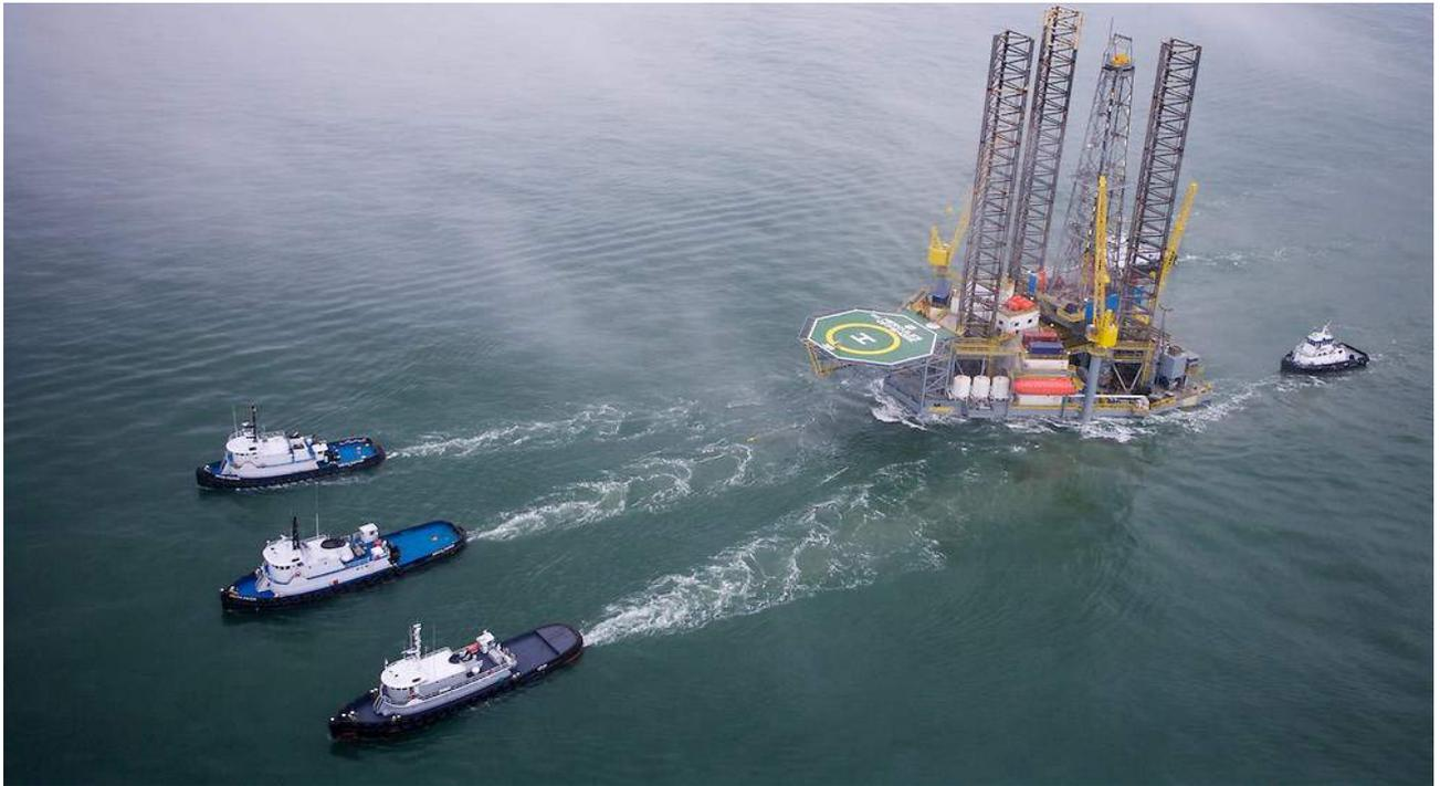
*Figure 3-6 Towing of Jack up Barge*
