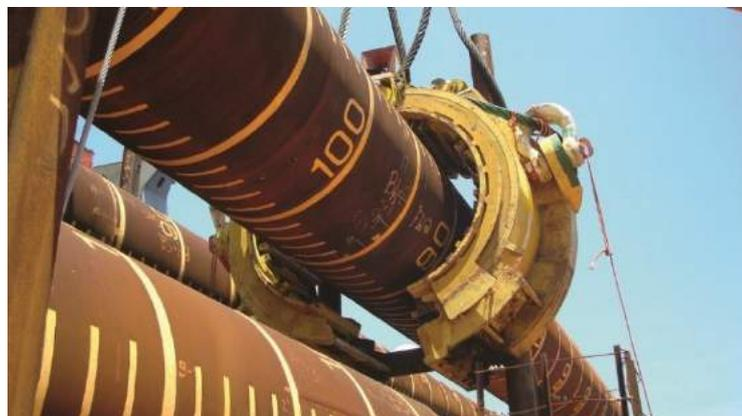
*Figure 6-119 External Lifting Tool (ELT) (IHC n.d.)*
