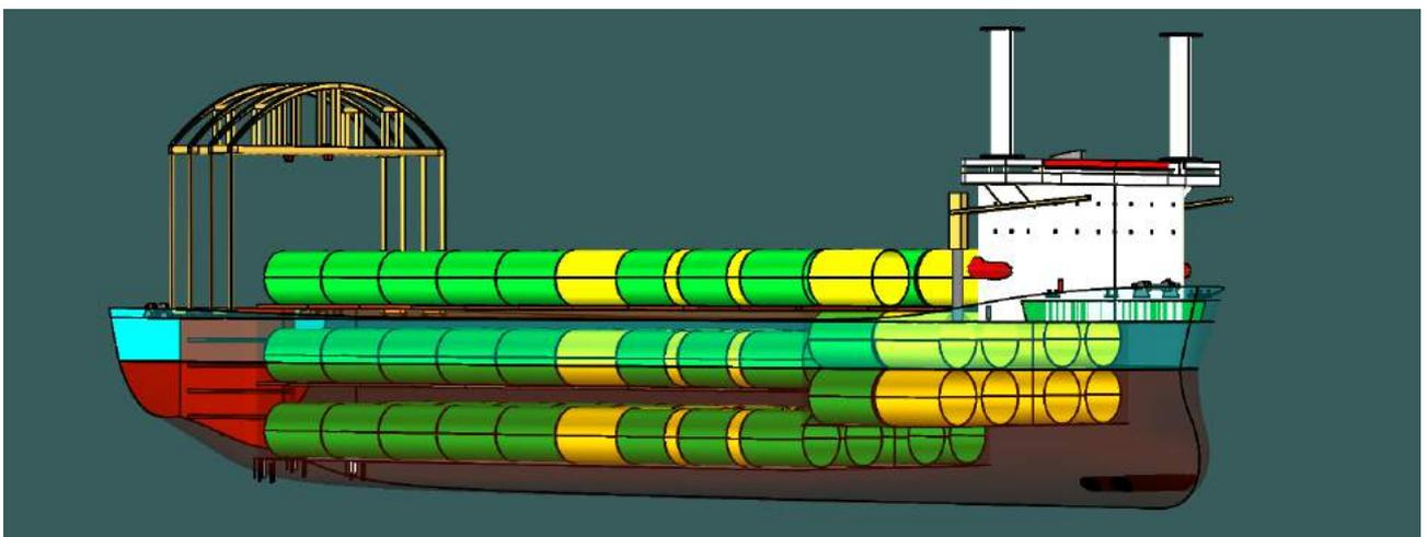
Figure 6-168 Loading of 24 set of MP plus TP (Perspective View)
