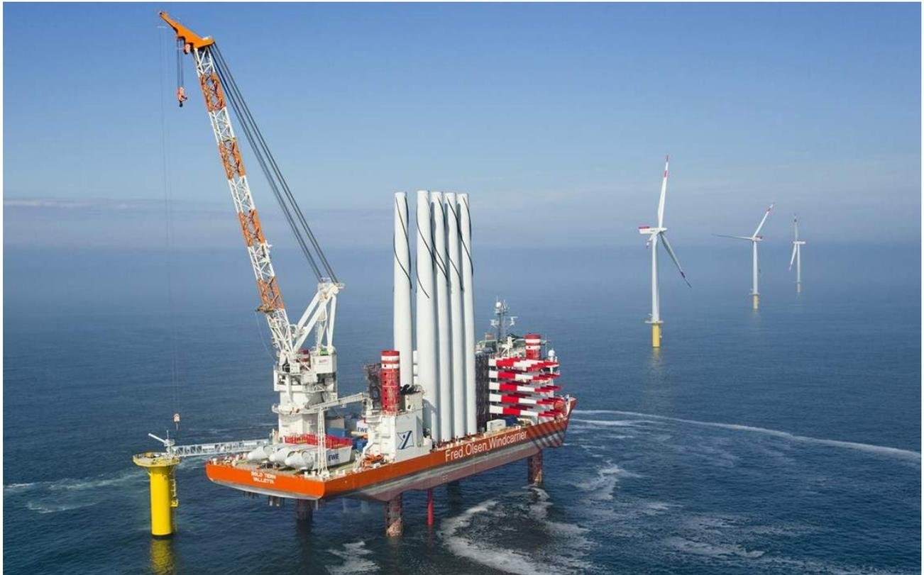
*Figure 3-8 Jack Up Installation Vessel or Wind Turbine Installation Vessel*
