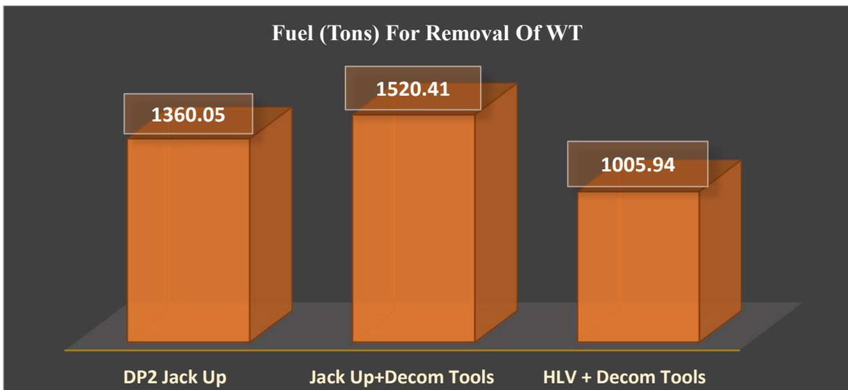
Figure 3-38 Fuel Consumption of Various Logistic Configuration in Decommissioning of Noblewind OWP
