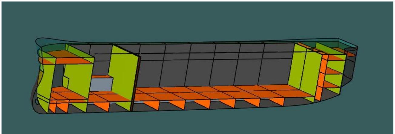
Figure 5-26 Cross Section of Double Bottom, (top)side Tanks
