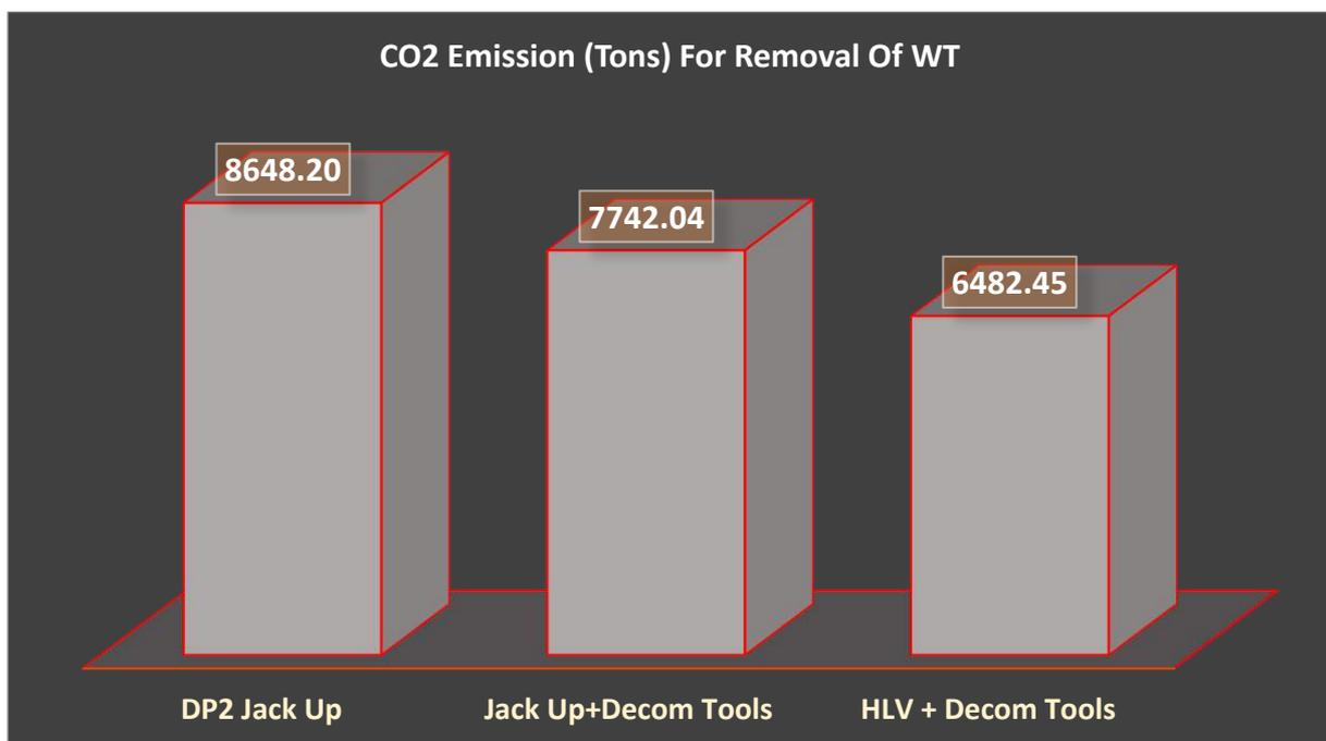
Figure 3-46 CO2 Emission of Various Logistic configuration for Decommissioning of Hornsea 1 OWP
