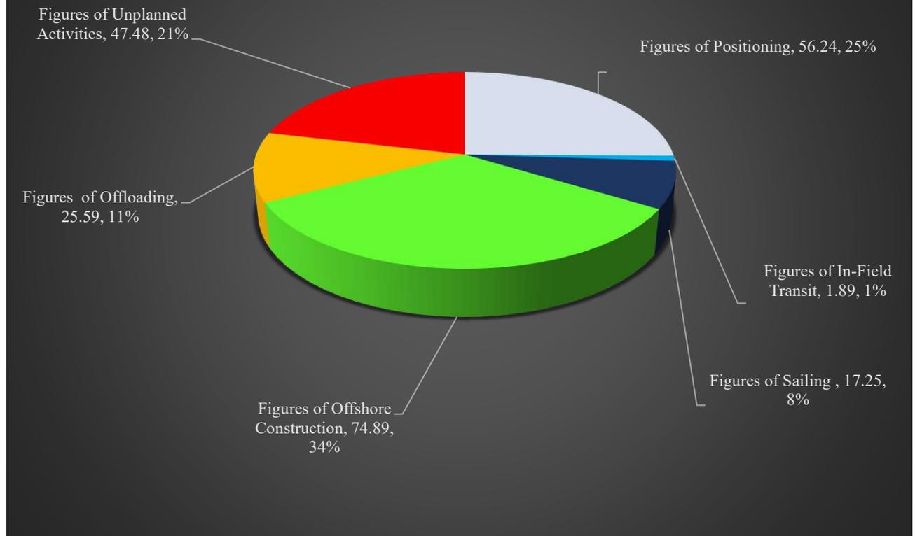
Figure 3-40 Break Down of Hornsea 1 offshore Wind Farm Decommissioning with a Jack up
