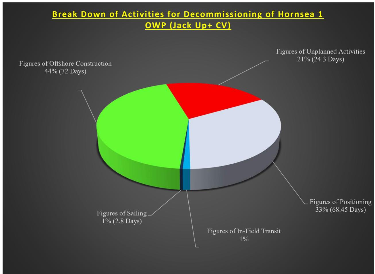
Figure 3-41 Break Down of Hornsea 1 offshore Wind Farm Decommissioning with a Jack Up+ Decom Tools Vessel
