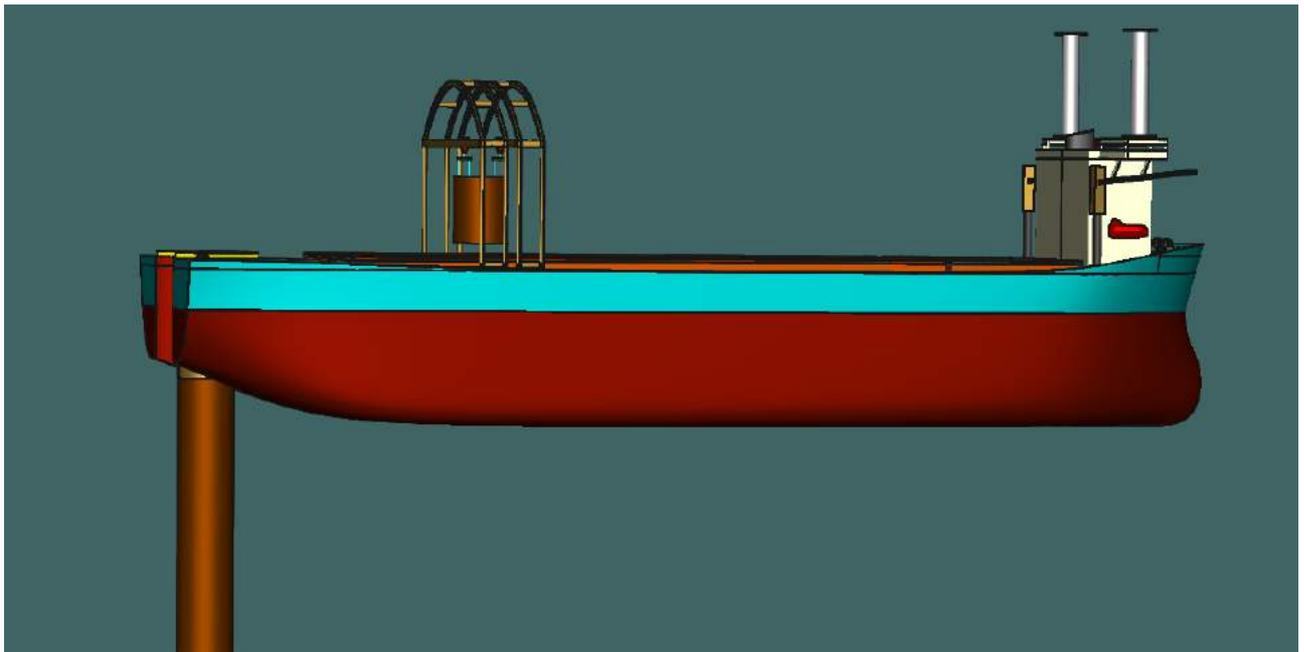
*Figure 6-153 Transferring the Cut Section of Monopile*
