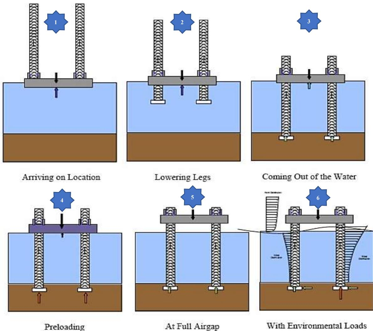
Figure 3-5 Transition Modes of a Jack up Vessel
