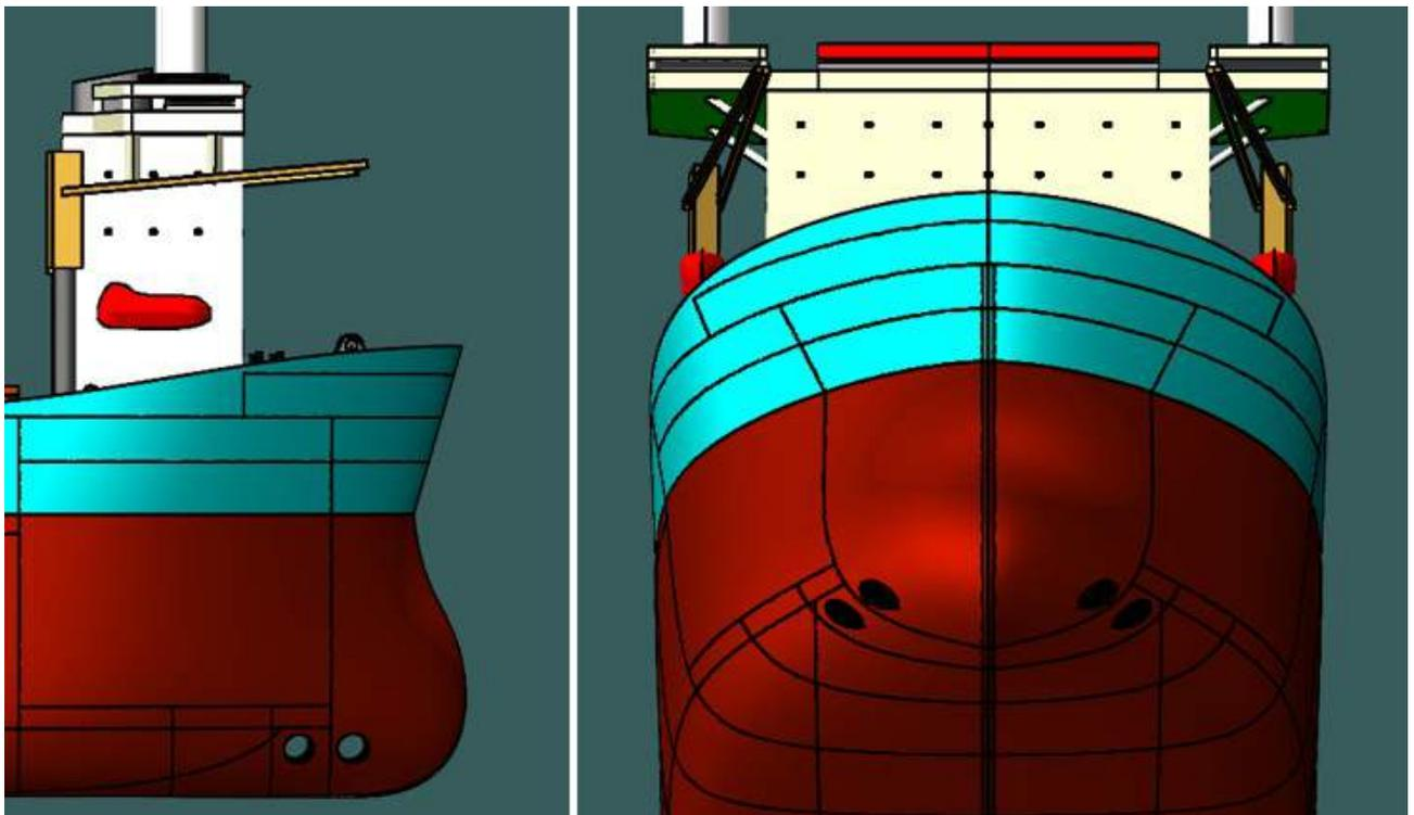
Figure 5-72 Bow Thrusters of Decom Tools Vessel
