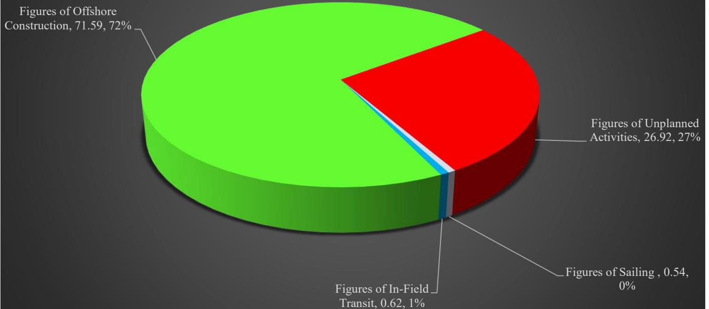
Figure 3-51 Break Down of Hohe See offshore Wind Farm Decommissioning with a HLV DP2+ Decom Tools Vessel
