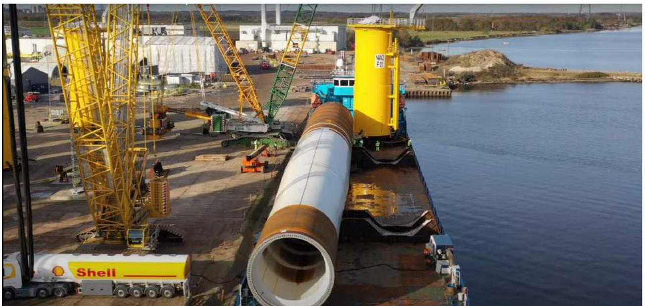
*Figure 3-20 Aura Heavy Load Carrier Loaded with 2 Monopiles+2 TP*
