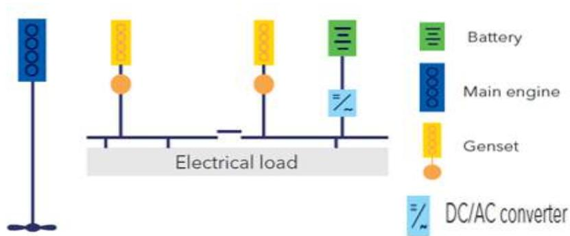
Figure 4-31 Mechanical Propulsion with Battery Hybrid Electrical Power Plant
