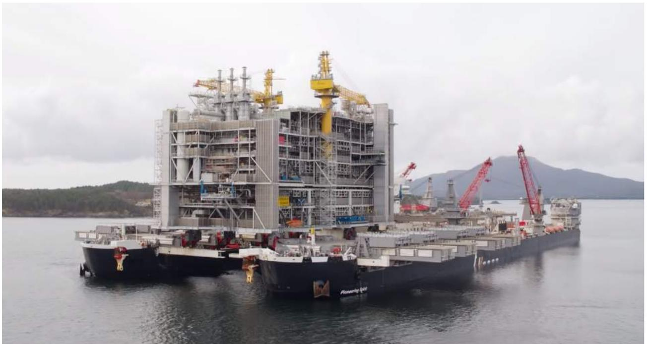
*Figure 3-3 Topside is Loaded onto the Pioneering Spirit*
