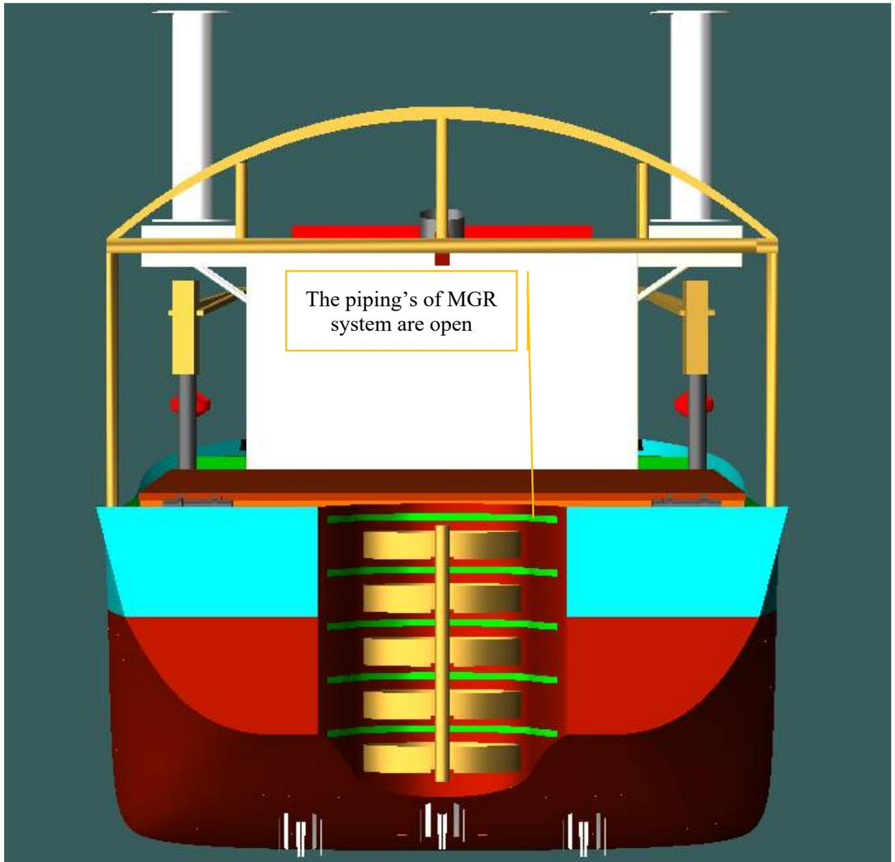
Figure 6-158 The Marine Growth System (In green colour)
