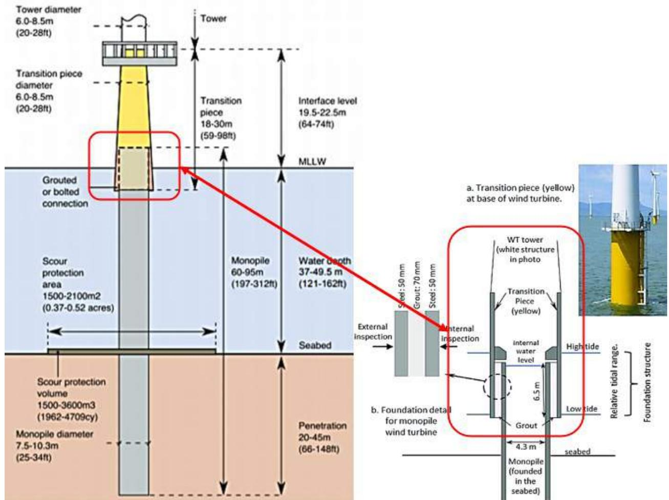
Figure 6-87 Detail of Installation of TP & MP
