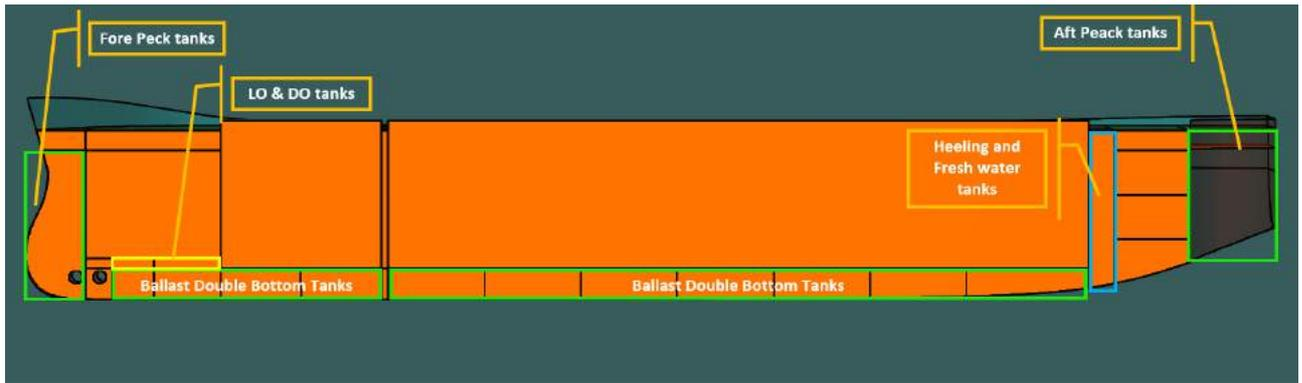
Figure 5-22 Side View of Decom Tools Vessel's Tanks
