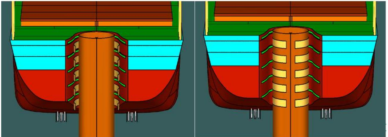
Figure 6-134 Status of Pile Grippers
