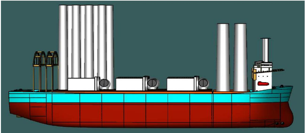
Figure 6-25 Side View of Load out of 12MW Blades, Nacelle & Tower
