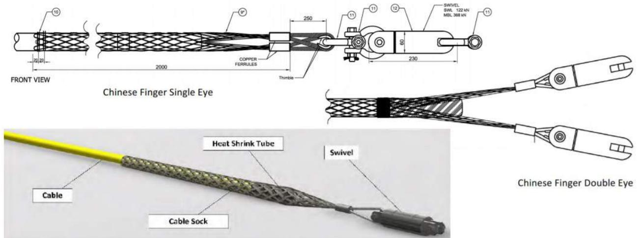
Figure 6-199 Chinese Finger and Drawing of Connection
