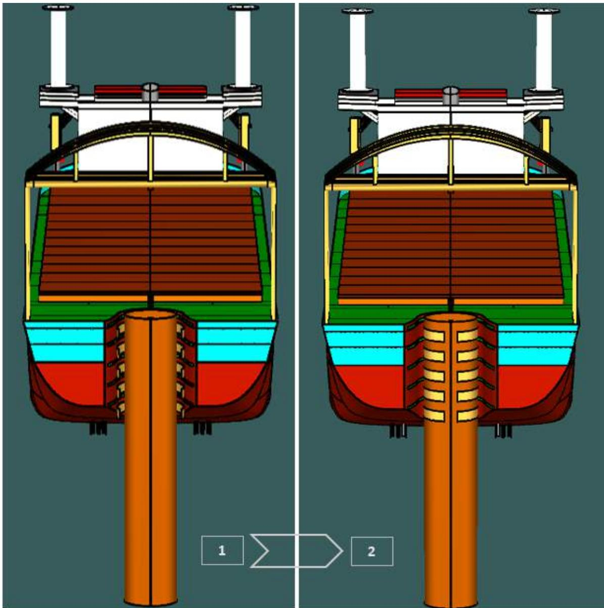
Figure 6-133 Decom Tools Vessel Positioned Around the Monopile
