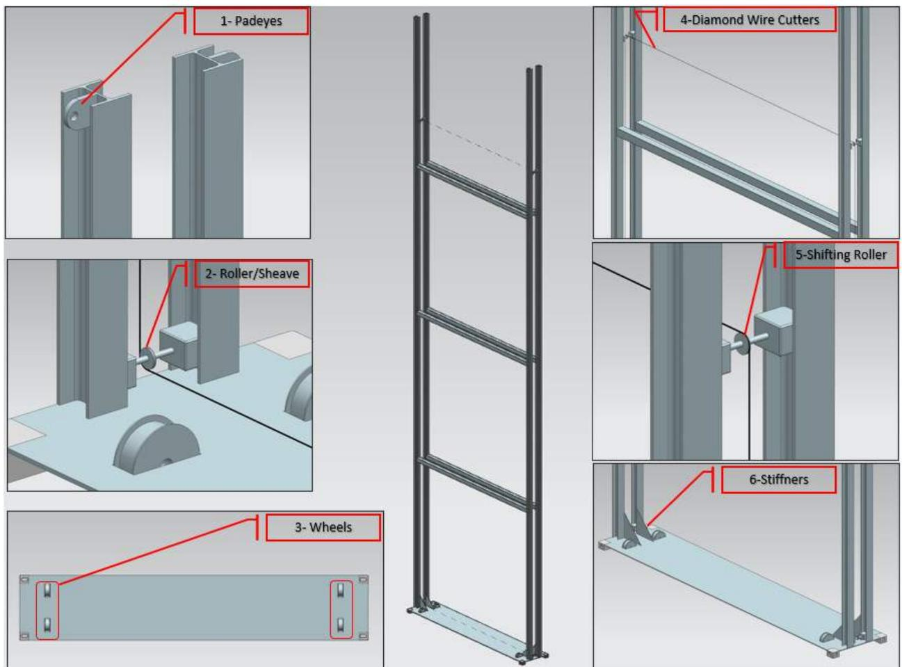
Figure 6-73 Details of Blade Cutting Tool
