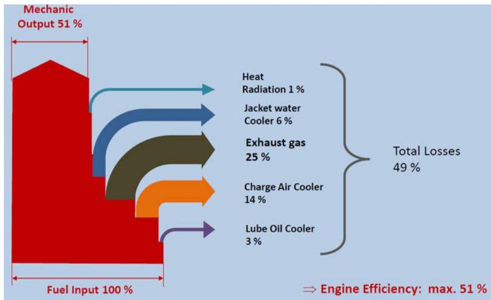
Figure 4-7 Thermal energy balances or Sankey-diagram of 2-Stroke Cross Head Engine (Meyer 2019)
