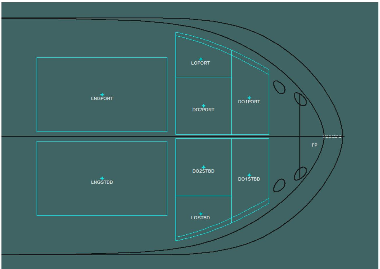
Figure 5-33 Plan of LNG and Diesel Oil Tanks
