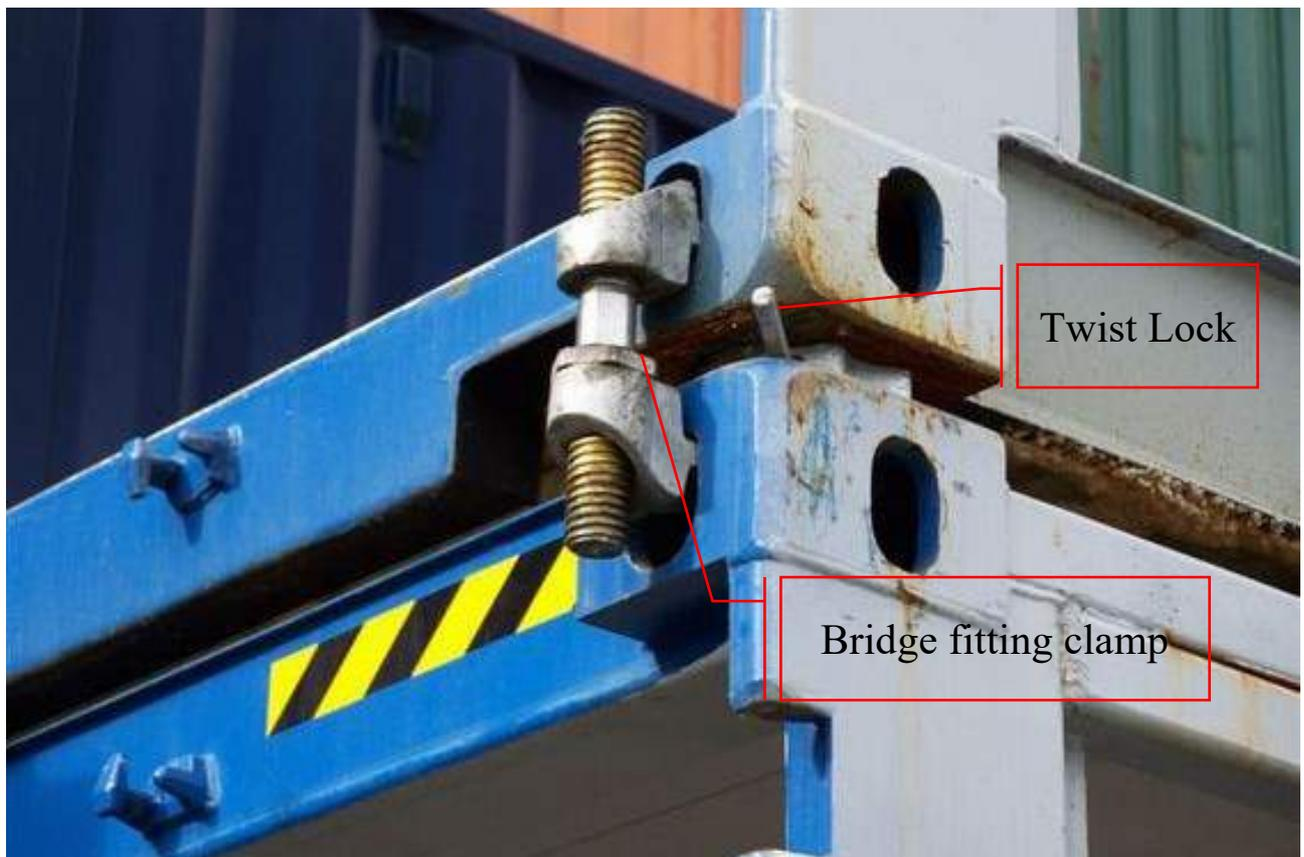
*Figure 6-65 Application of Twist lock in securing containers*
