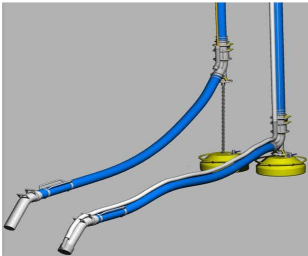
*Figure 6-190 Common Type of Airlift (inzenjering n.d.)*
