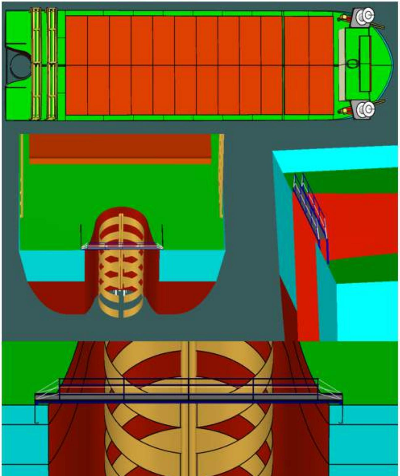
*Figure 6-95 Mobile Access Platform for Cutting MP/TP*
