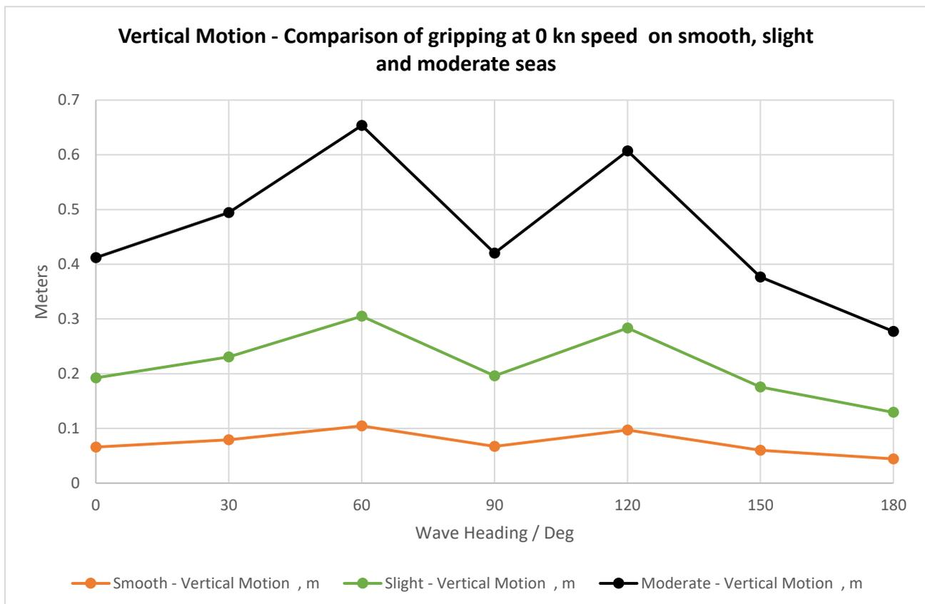
Figure 8-11 Absolute Vertical Motion at Gripper point on three different Sea States
