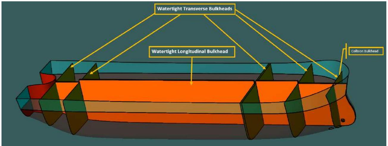
Figure 5-17 Longitudinal and Transverse Bulkhead of Decom Tools Vessel
