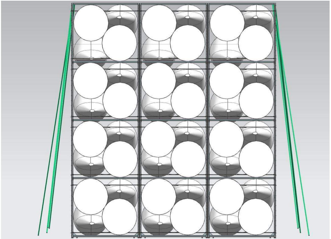
*Figure 6-83 3.6 MW blades inside the racks (front View)*
