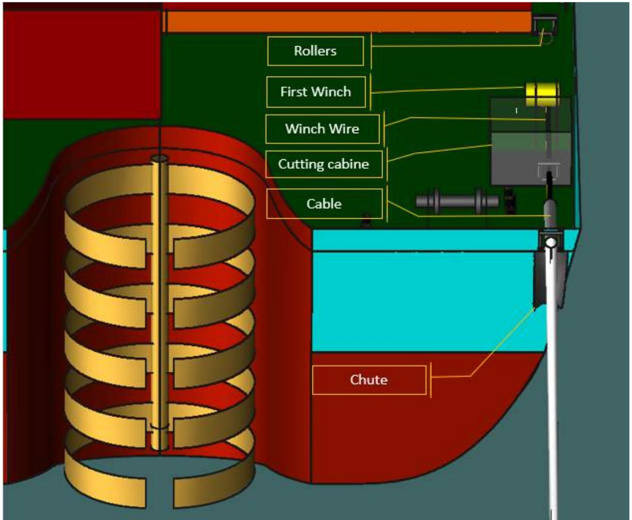
Figure 6-215 Chute, Hydraulic Cable Clamp and 1st Winch
