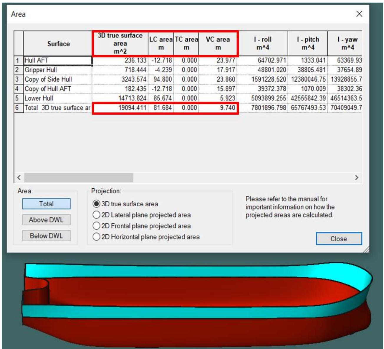
Figure 7-5 Calculating the Surface of Decom Tools Hull
