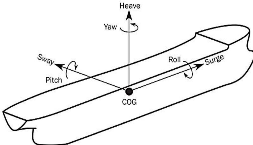
*Figure 8-1 Motions of a Floating Vessel*
