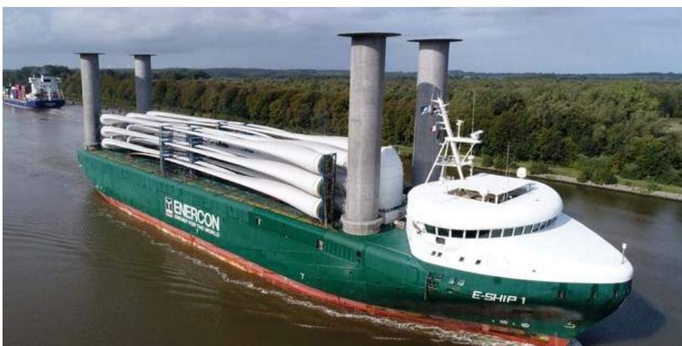
Figure 4-29 Enercon E-Ship 1 is Equipped with 4 Rotors<sup>41</sup>
