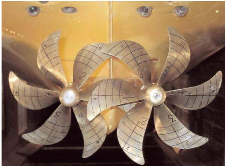
*Figure 4-12 Overlapping Propeller*
