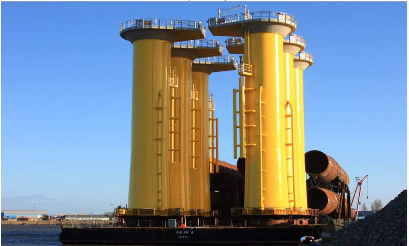
*Figure 3-18 Transportation barge is loaded with Monopile & TP*
