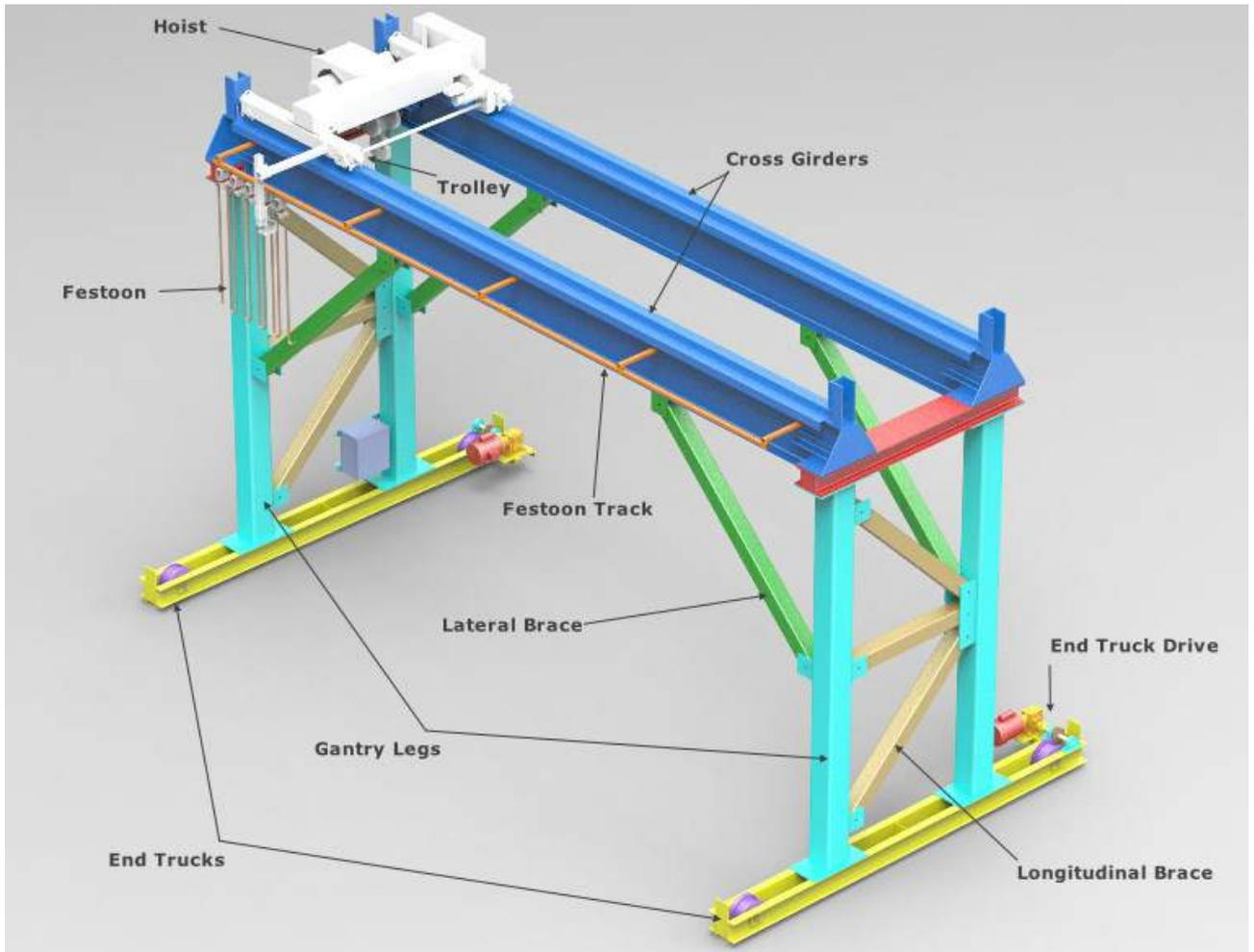
Figure 5-40 Elements of a Gantry Crane (NAICRANES n.d.)
