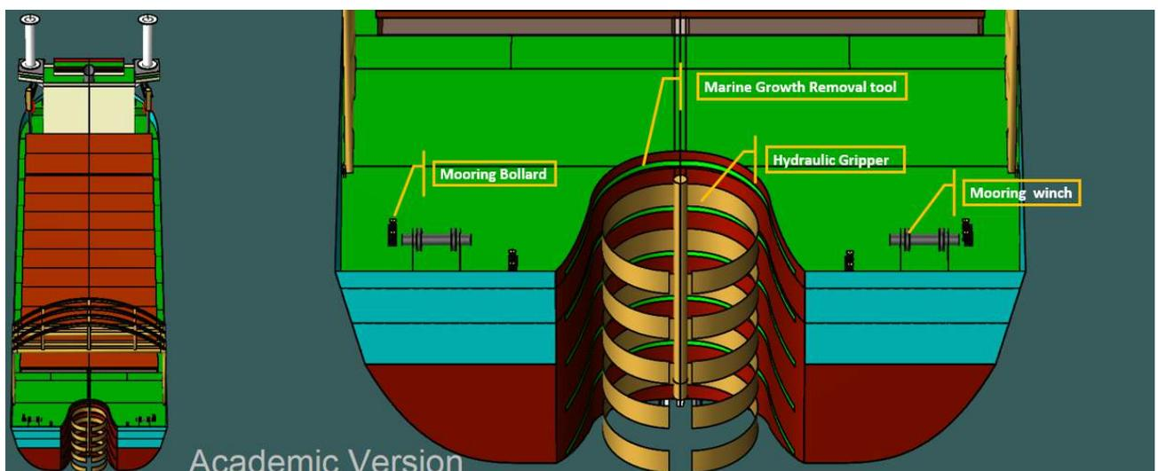
Figure 6-157 The Marine Growth System (In green colour)
