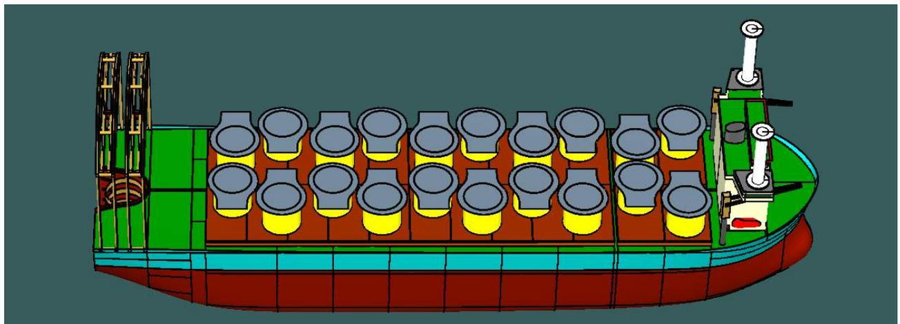
Figure 6-109 TPs loading arrangement (Bird's Eye View)
