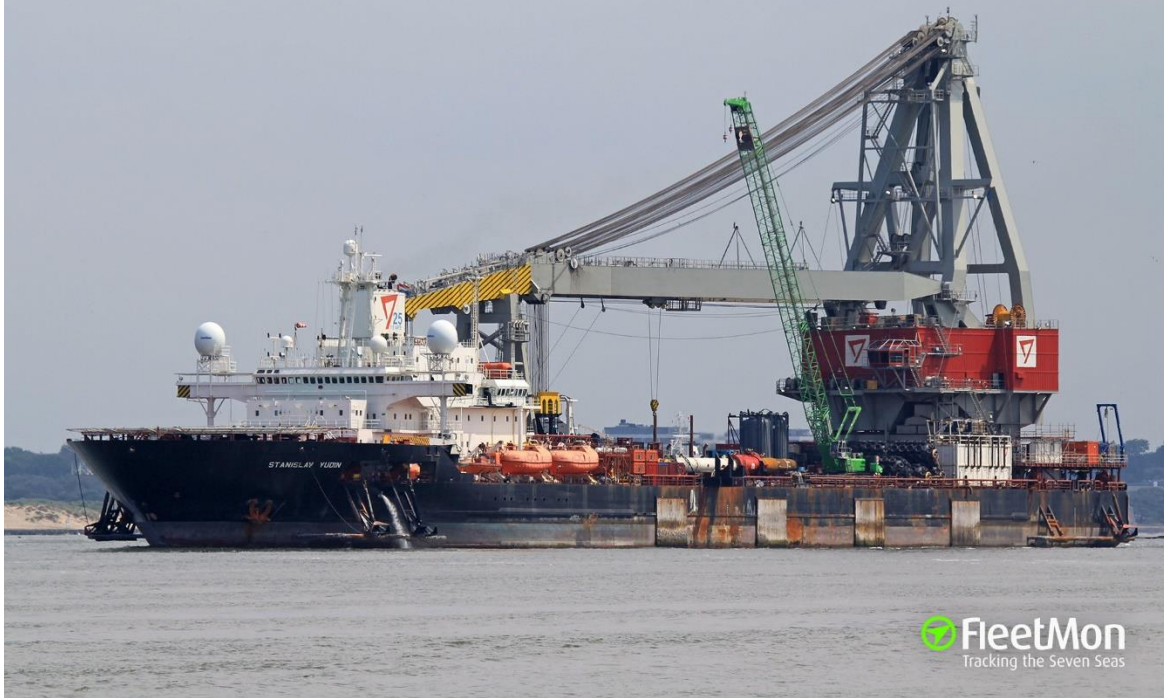
Fig. 12. The Stanislav Yudin HLV was used for foundation installation in Greater Gabbard, Gwynt y Mor, and Global Tech I wind farms
