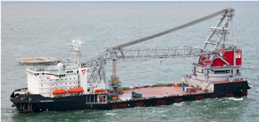
Fig. 11. The Oleg Strashnov HLV used for foundation installation in Sheringham Shoal, Trianel Windpark Borkum 1, Borkum Riffgat, and Meerwind wind farms 1
