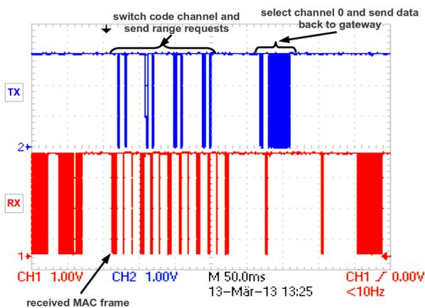
Fig. 11: Timing of a slave node with four ranging measurements
