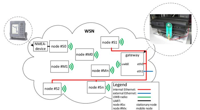
Fig. 2: Ad-hoc network topology consisting of mobile nodes (slaves), stationary anchors and a master (gateway)
