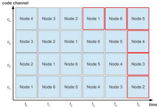
Fig. 6: Scheduling of slave nodes inside the ranging period with 6 slave nodes
