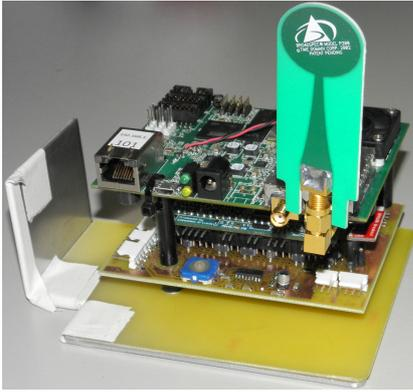
Fig. 3: Picture of the current evaluation model, showing a custom baseboard and off the shelf UWB transceiver modul.
