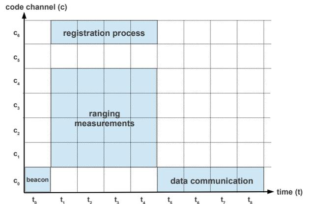
Fig. 5: Detailed view of slot configuration by code channel and time assignment
