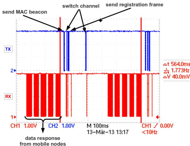
Fig. 10: Timing of the master with five slave nodes connected
