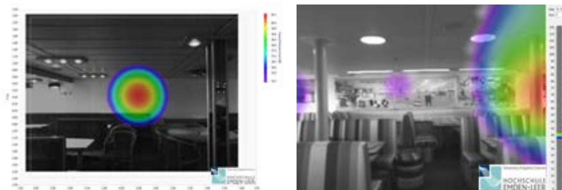
Figure 16: Colour-coded acoustic measurement in the rear saloon before (left) and after (right) the reconstruction of the vessel. Frequency range: 1500 Hz - 1750 Hz.
