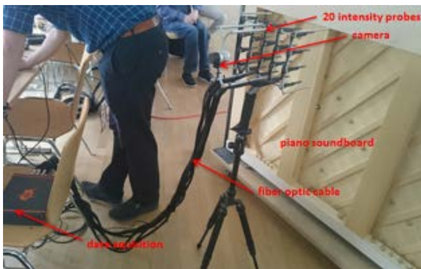
Figure 10: Experimental setup of the acoustic measurements on the piano soundboard using a handheld intensity array.
